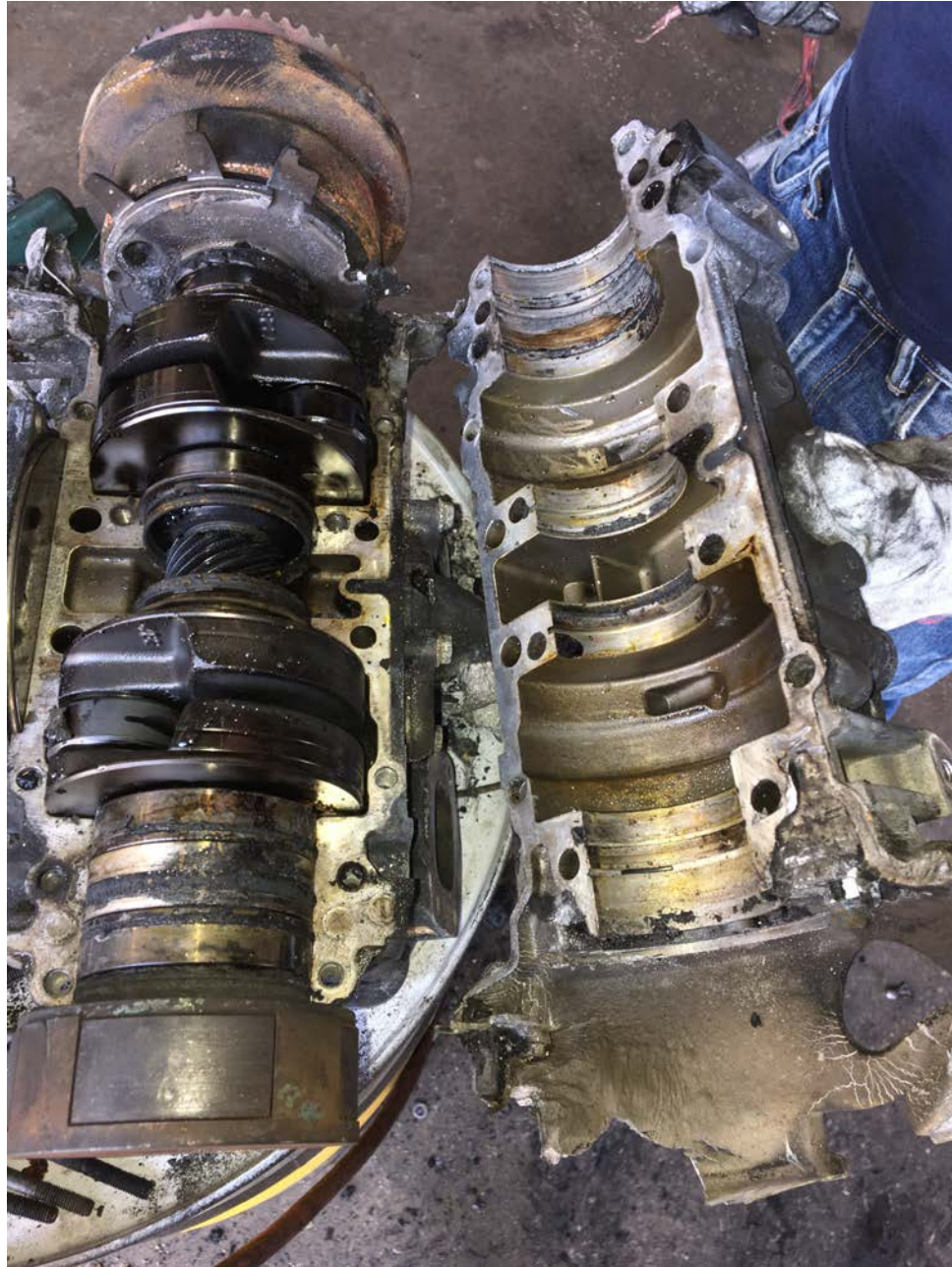
Photo 6 – Interior of engine after crankcase separation.
