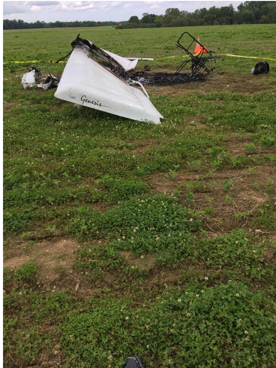
Photo 4 – Left profile of entire airplane impact and fire damage.
