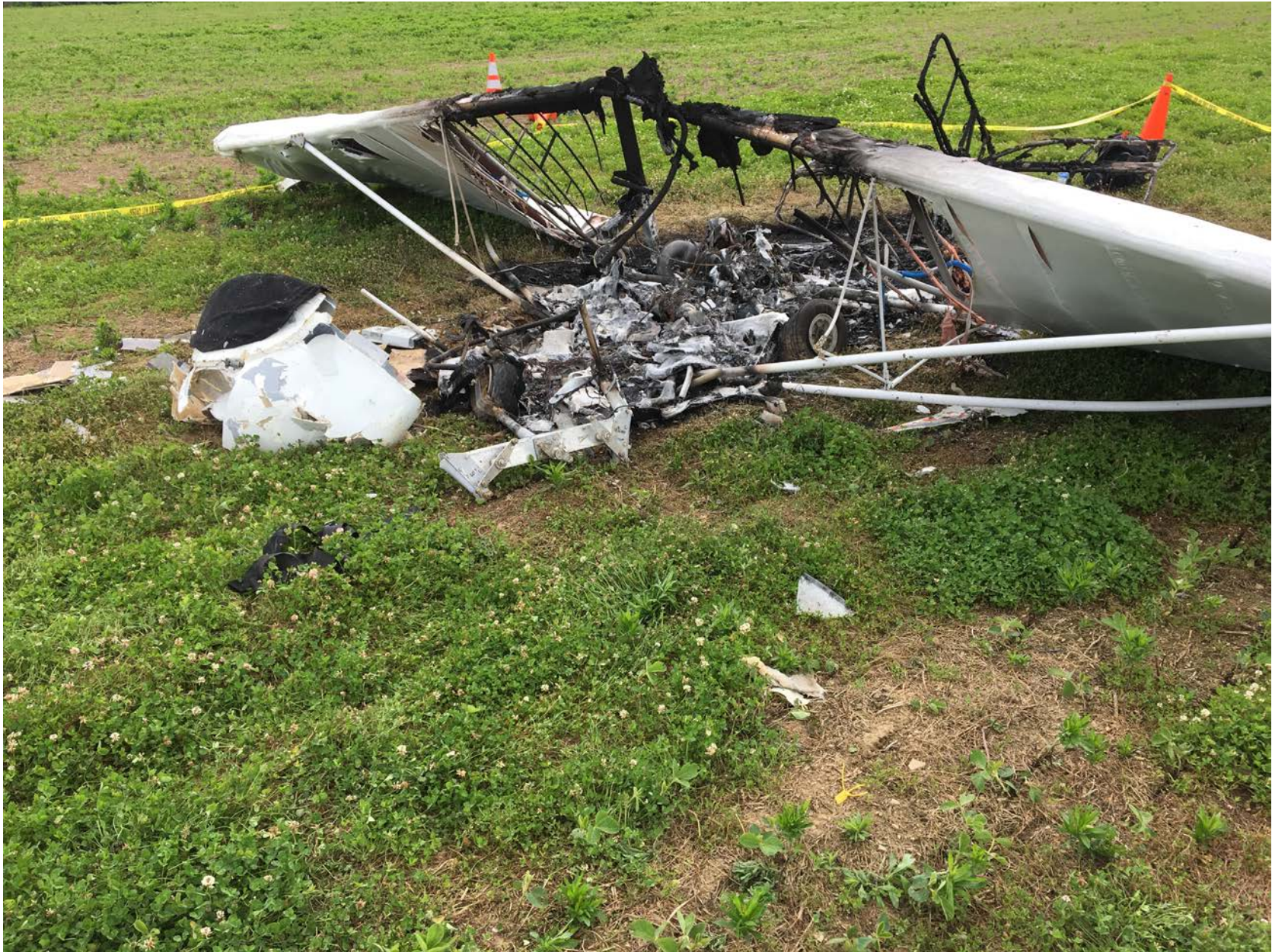
Photo 1 – Airplane impact and fire damage looking at left front quarter.
