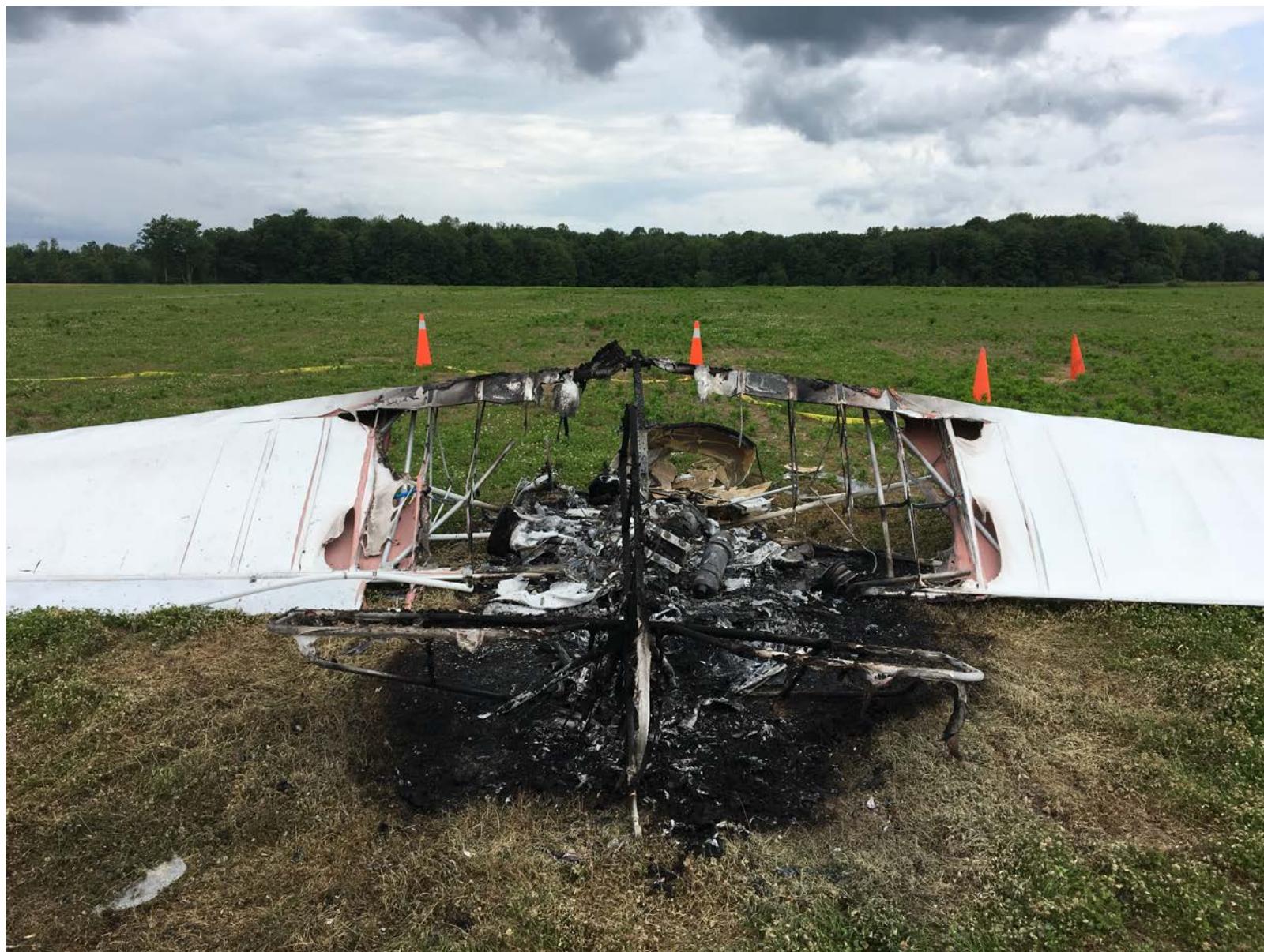
Photo 2 – Airplane impact and fire damage looking from the tail forward.
