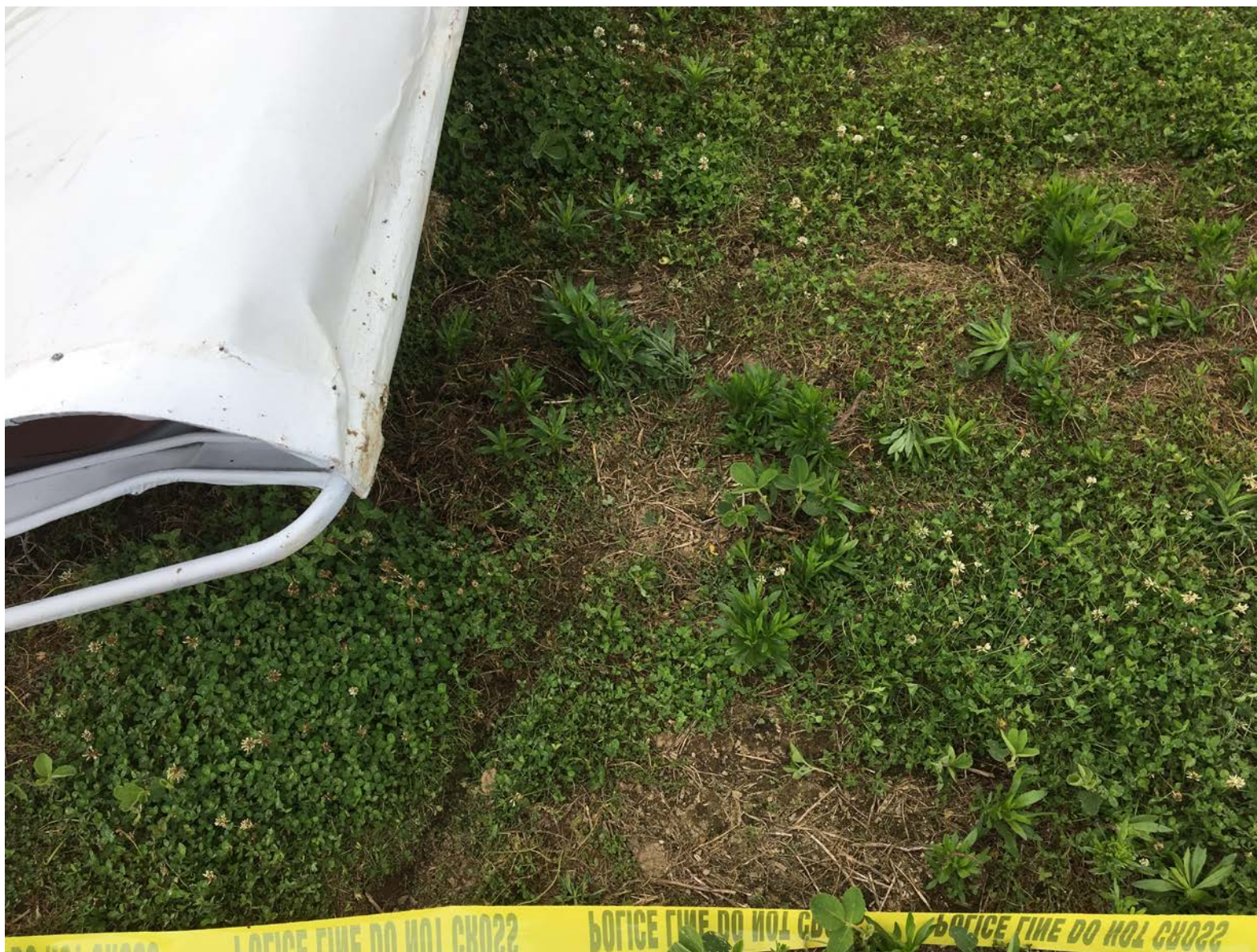
Photo 3 – Right wing damage and ground impact mark.
