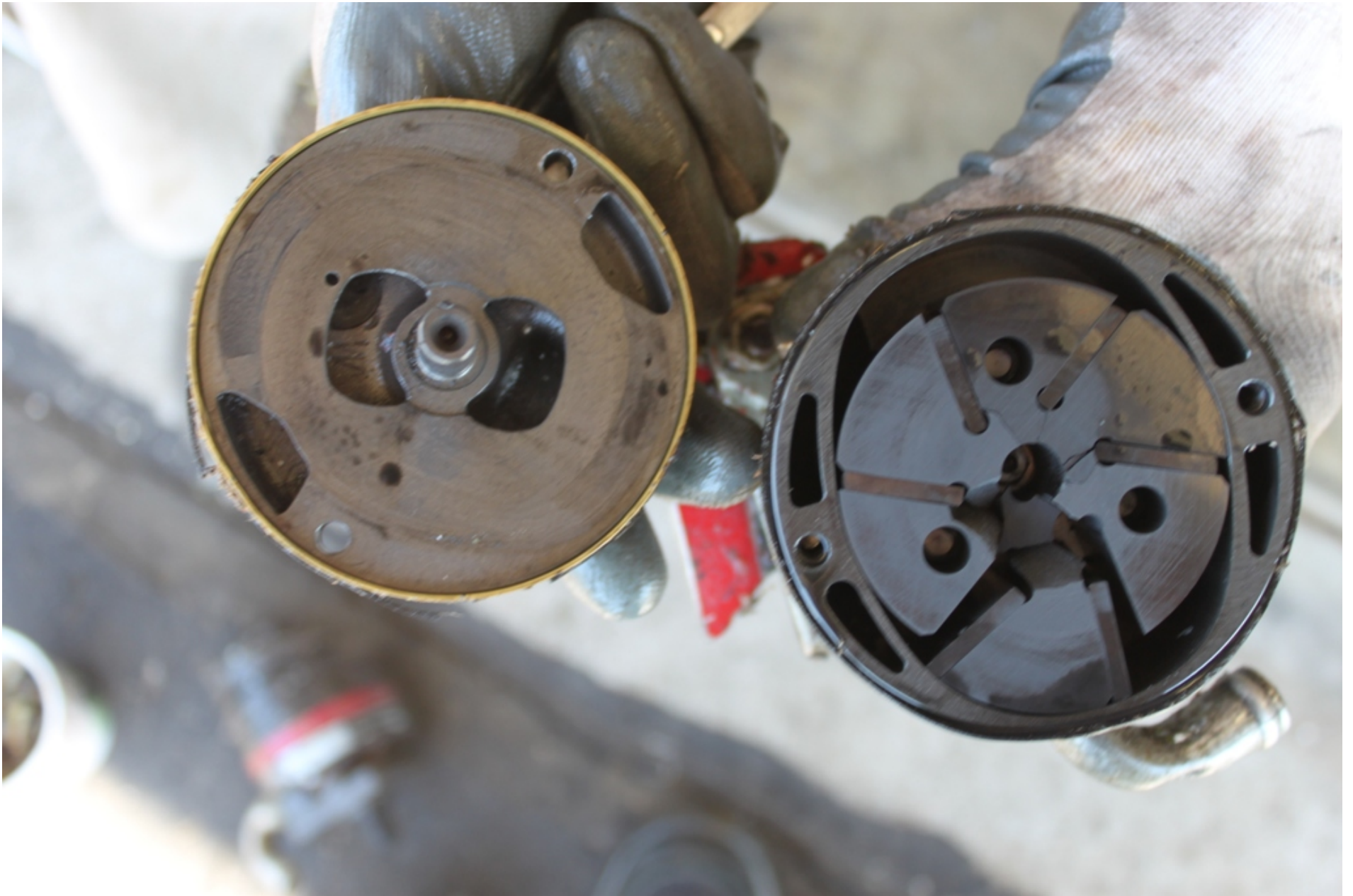
Photo 17 - NTSB Digital Photograph. View of the Interior of The Second Recovered Dry Air Pump. Note the Fractured Rotor.
