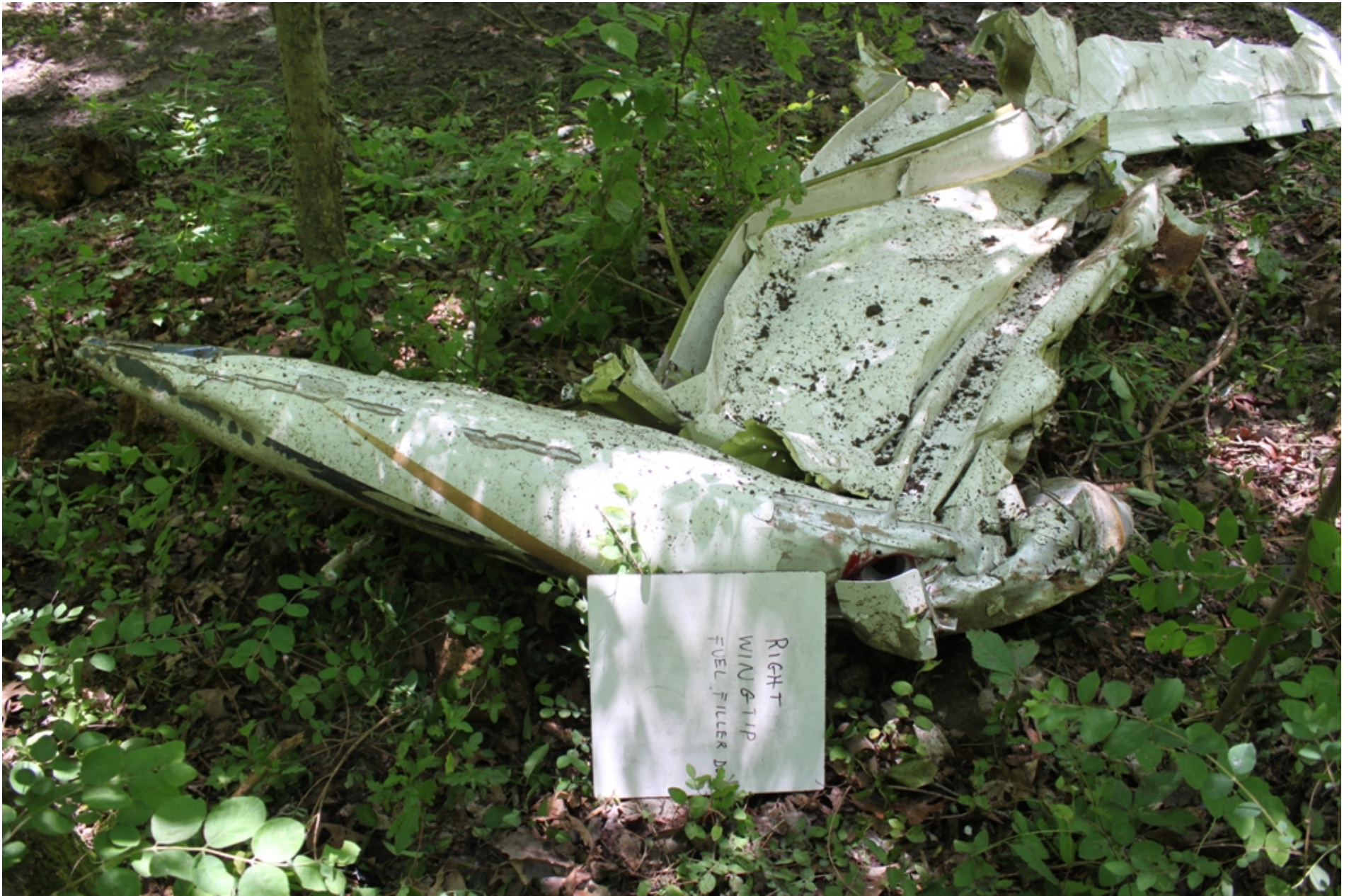
Photo 7 - NTSB Digital Photograph. View of the Outer Section of the Right Wing.
