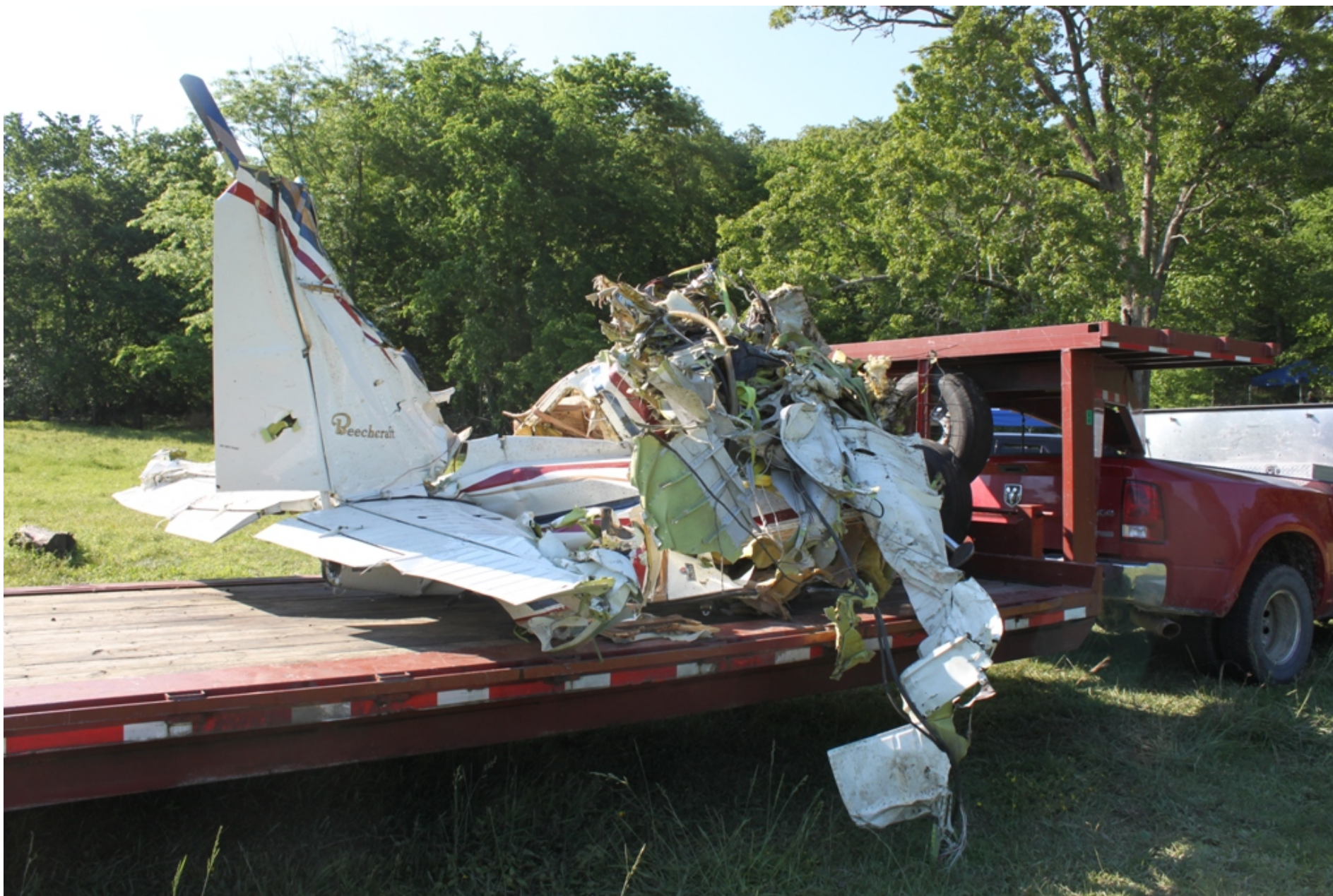
Photo 10 - NTSB Digital Photograph. Right Rear Quartering View of the Wreckage During Recovery. Note the damage to the Right Horizontal Stabilizer
