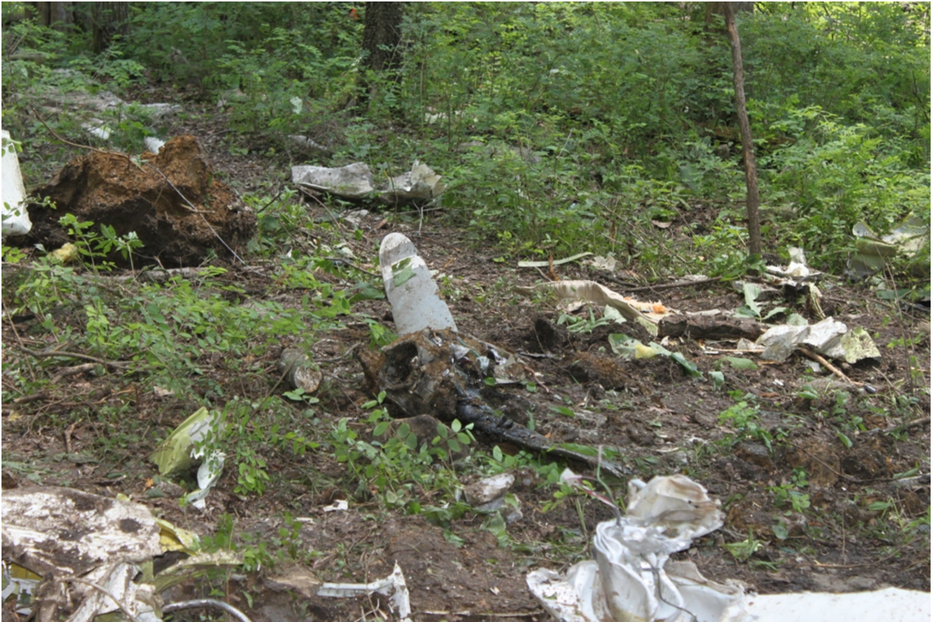
Photo 6 - NTSB Digital Photograph. View of the As-Found Position of the Propeller Assembly. Note the Missing Blade.
