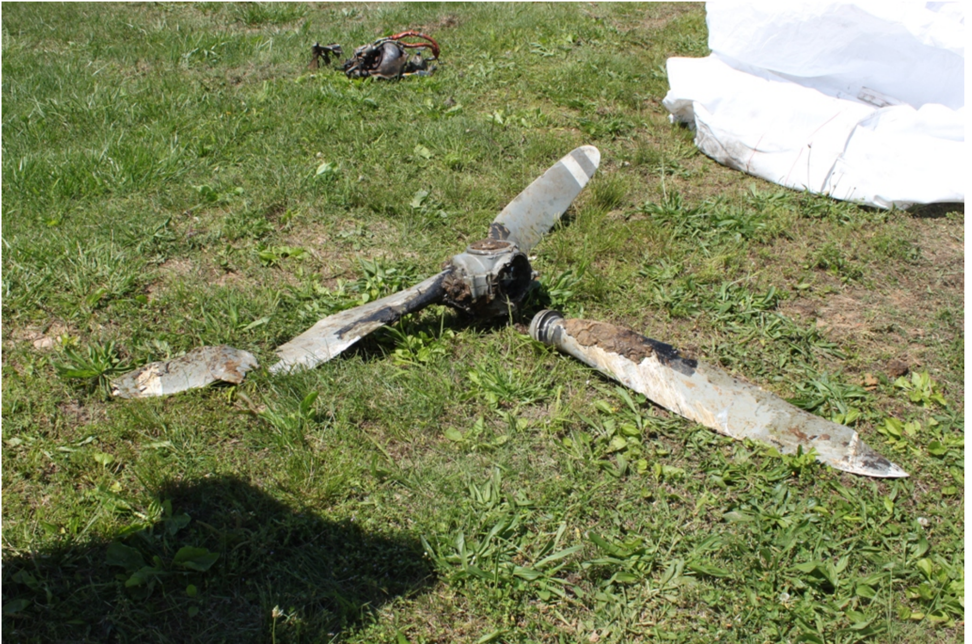
Photo 13 - NTSB Digital Photograph. View of the Propeller Assembly with the Separated and Fractured Blade Pieces in Position.
