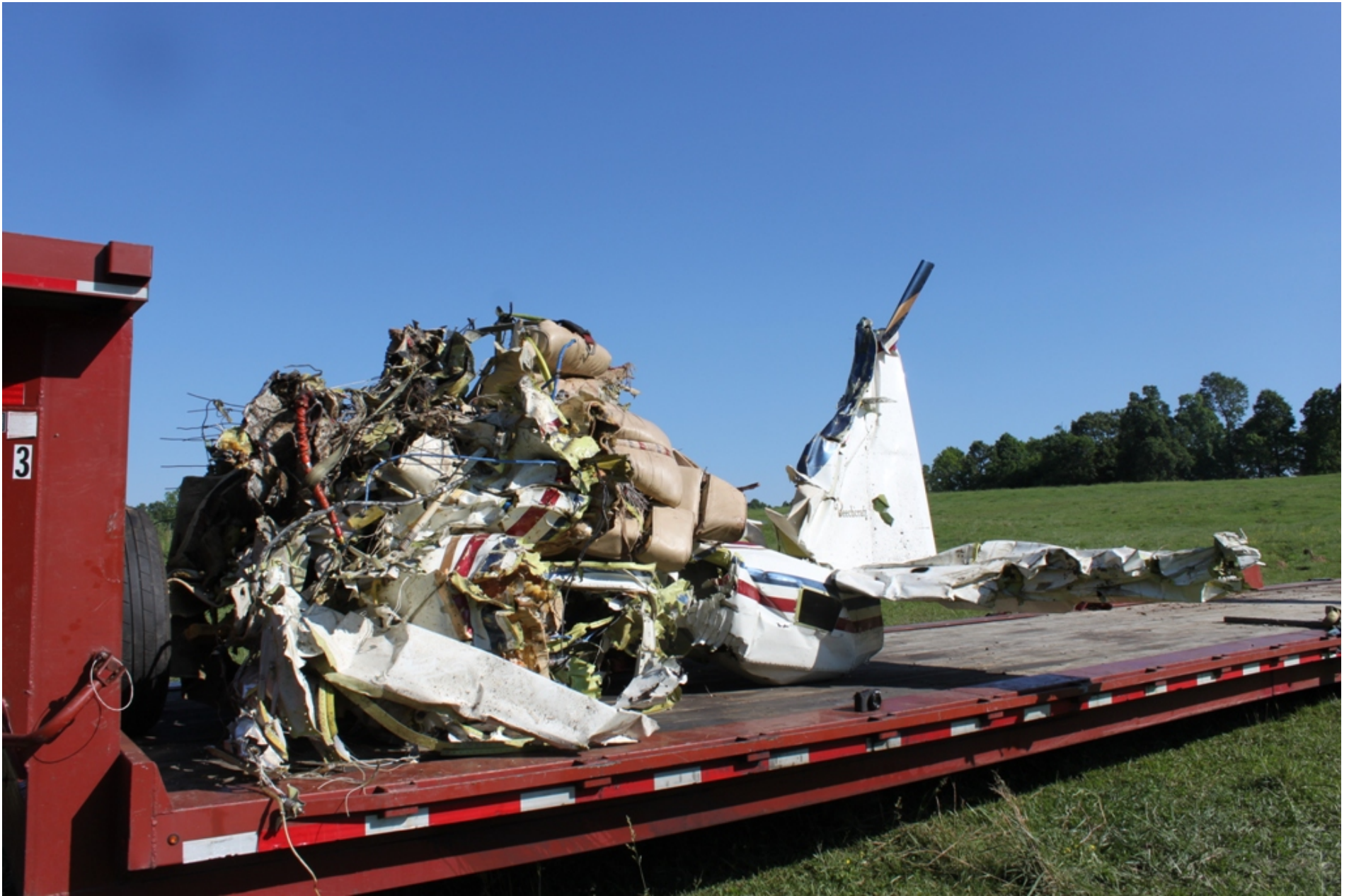
Photo 9 - NTSB Digital Photograph. Left Side View of the Wreckage During Recovery. Note the Damage to the leading edges of the Left Horizontal and Vertical Stabilizers
