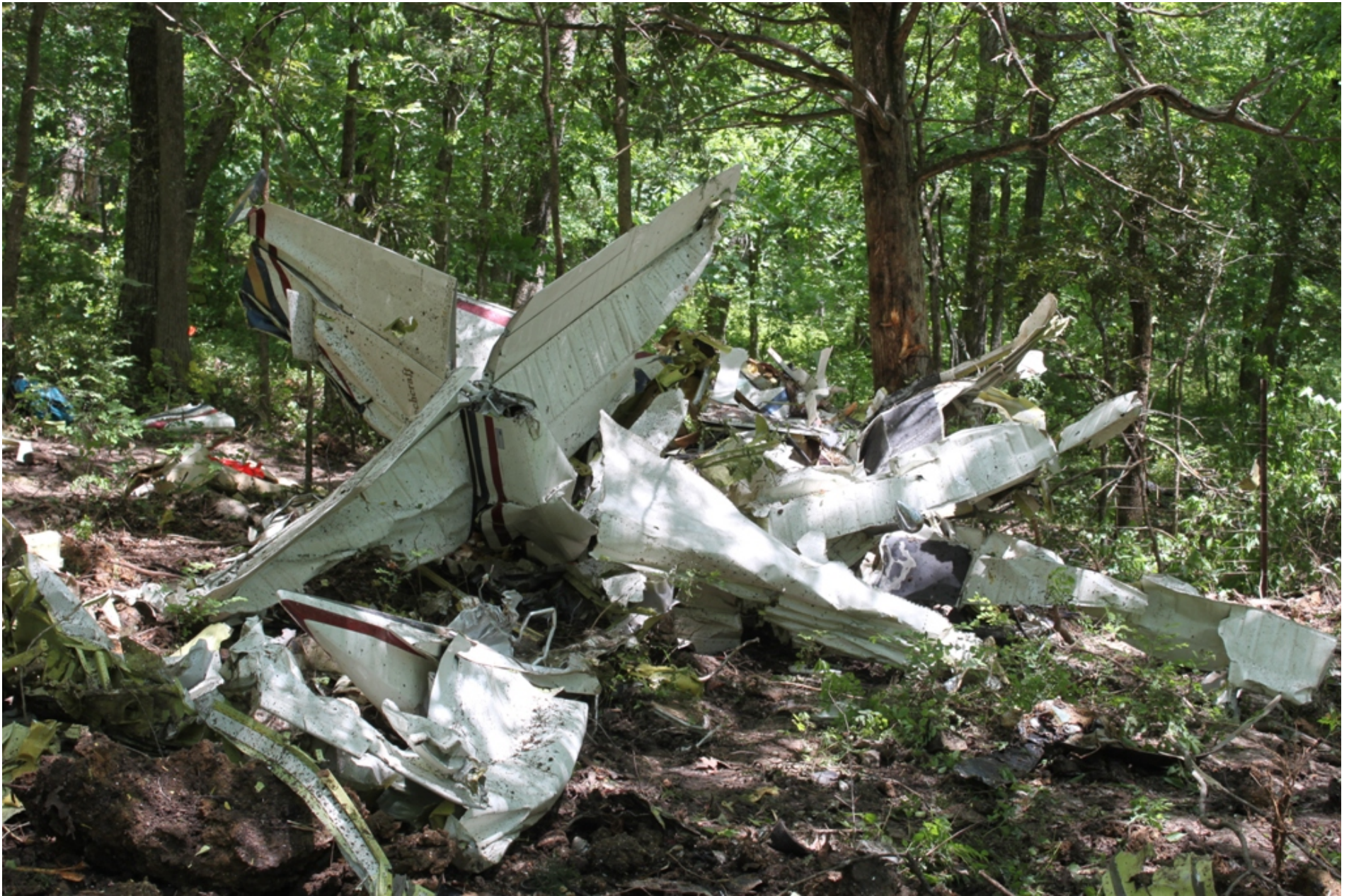
Photo 5 - NTSB Digital Photograph. Rear View of the Aft Empennage, Horizontal Stabilizers with Attached Elevators and Elevator Trim Tabs, Vertical Stabilizer with Attached Rudder
