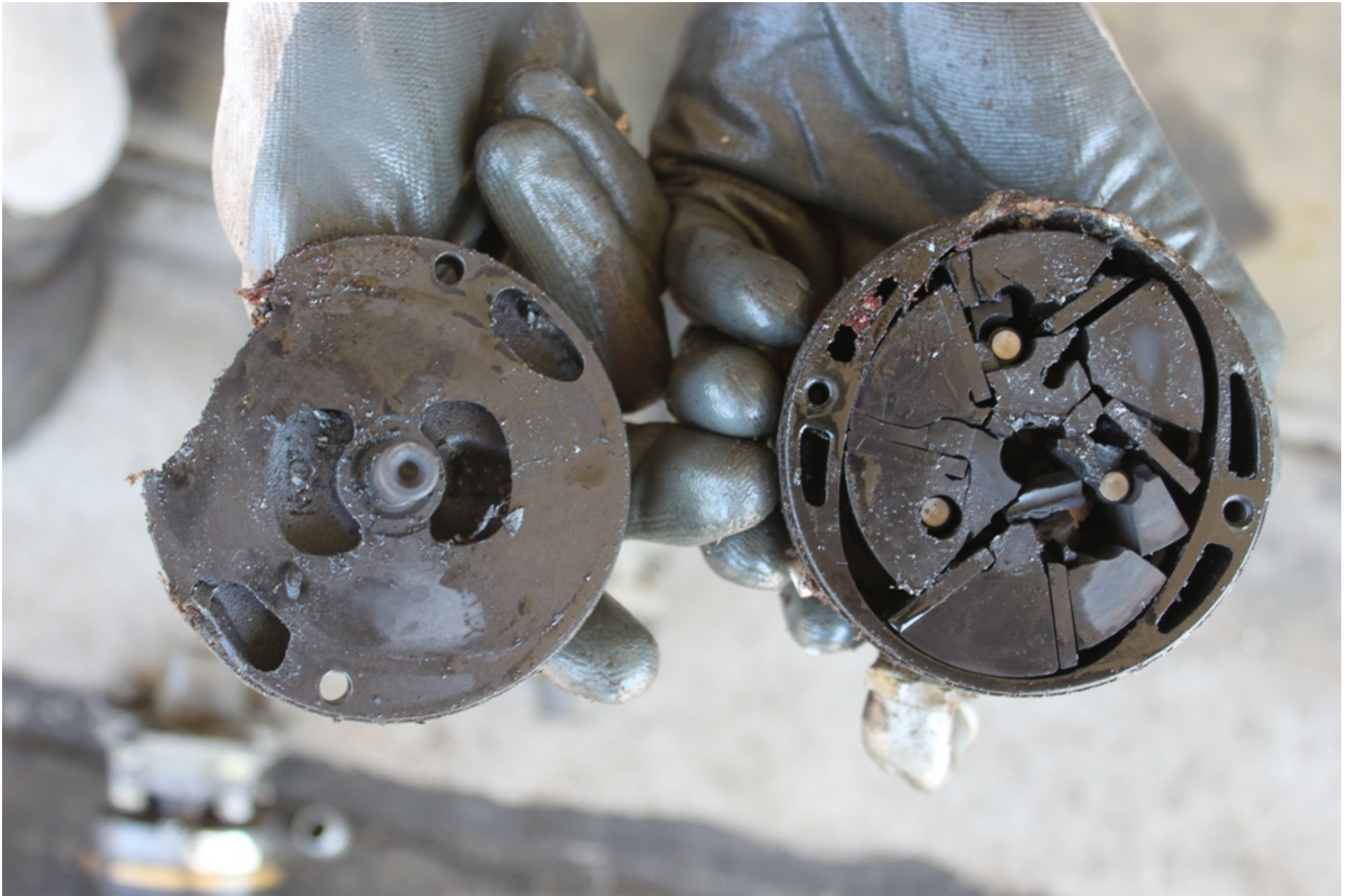
Photo 16 - NTSB Digital Photograph. View of the Interior of One Recovered Dry Air Pump. Note the Fractured Rotor and Several Vanes.
