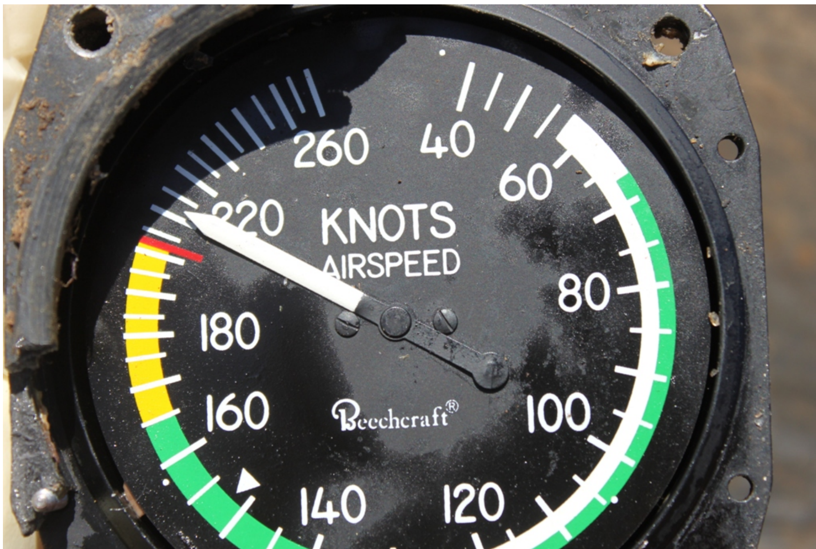
Photo 14 - NTSB Digital Photograph. View of the Airspeed Indicator with the Glass Removed. The needle was Stuck at 211 Knots.
