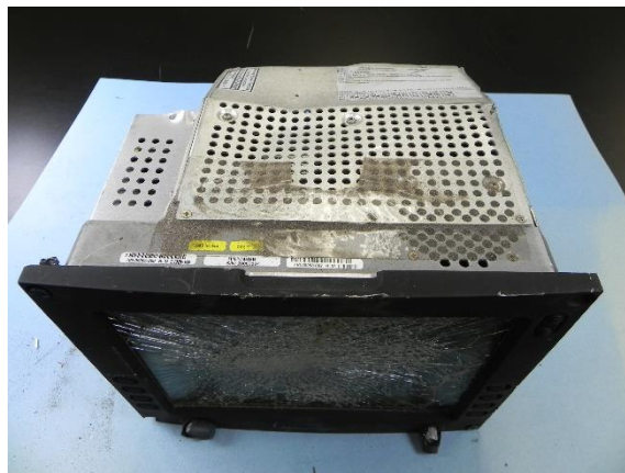
Figure 1. Damaged exterior of PFD.
