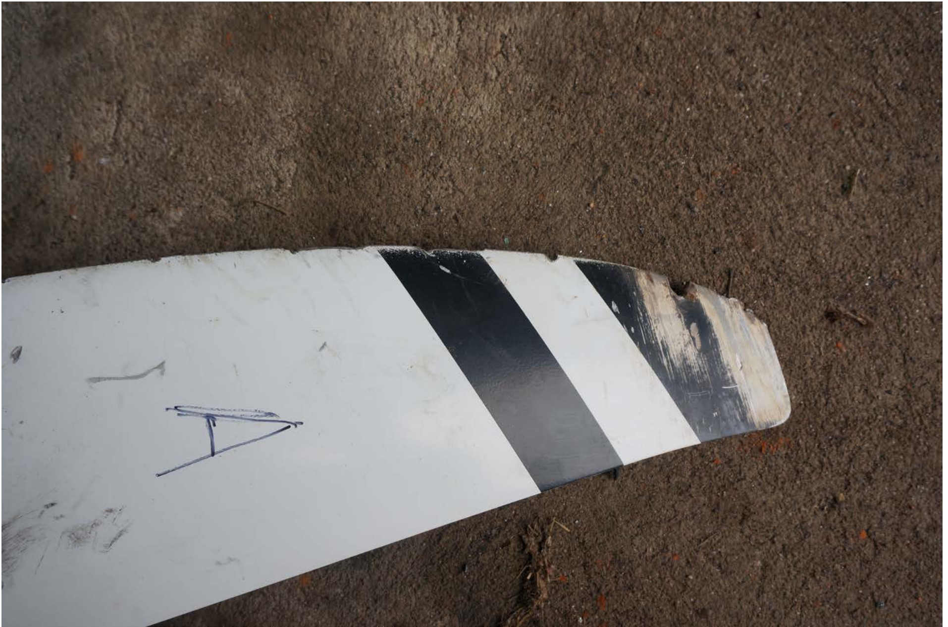
Photo 13 – Leading Edge Gouging on Propeller Blade
