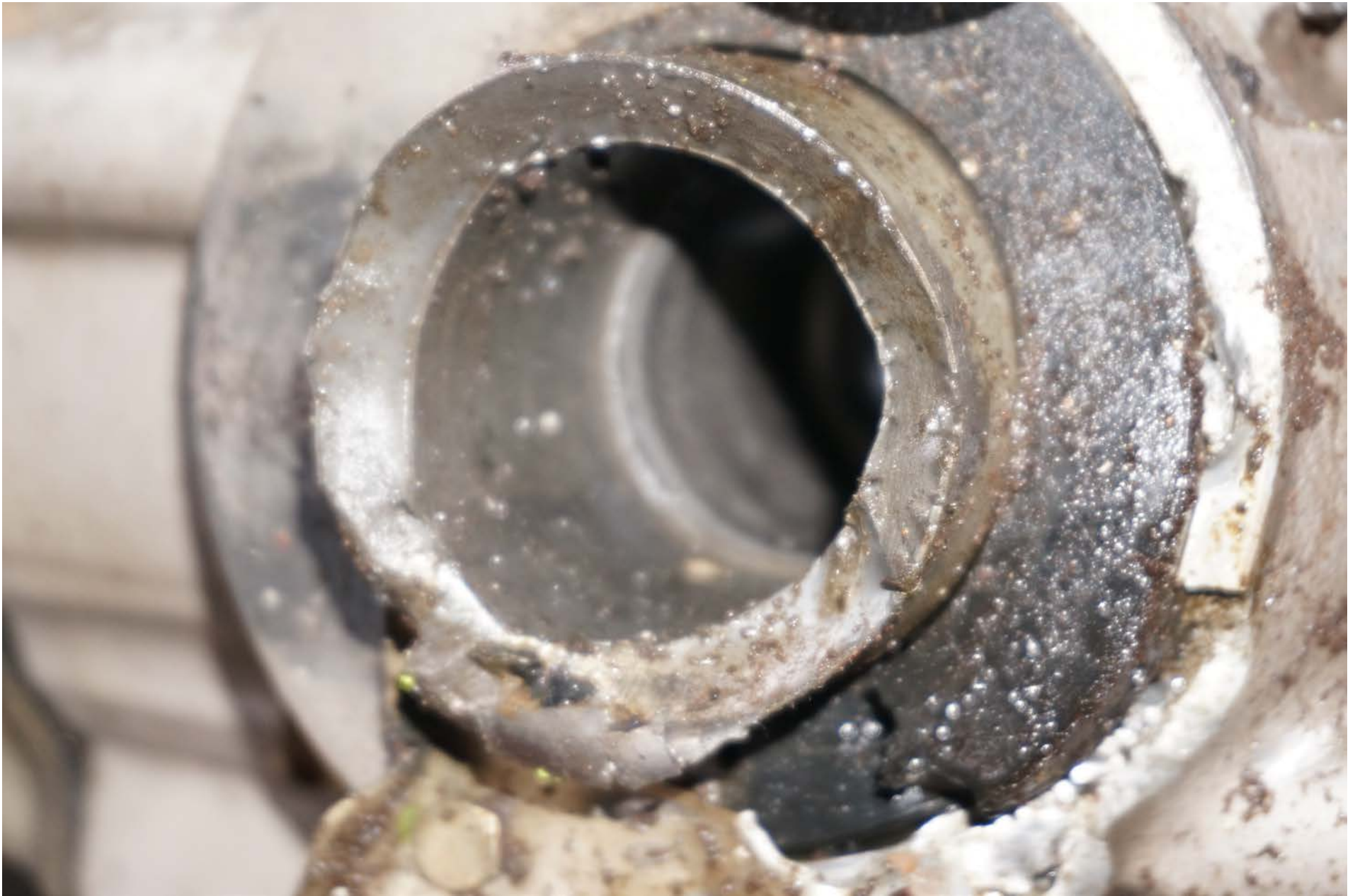
Photo 15 – Close Up Photograph of Fractured Crankshaft
