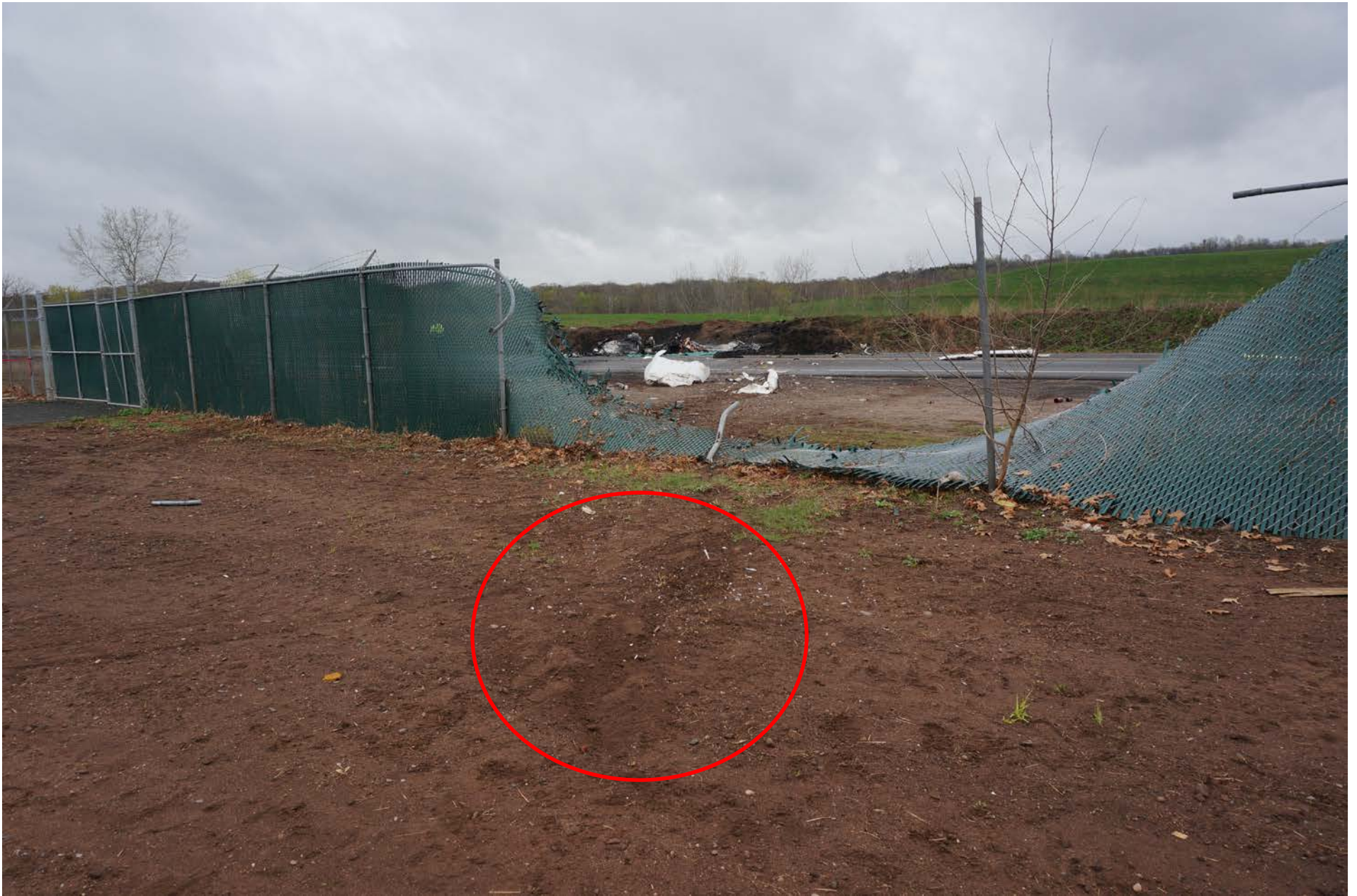
Photo 9 -Left Wing Tip Drag Mark
