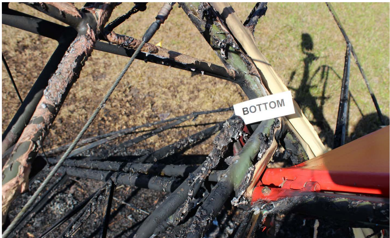
Figure 4 The reversed elevator cables.
