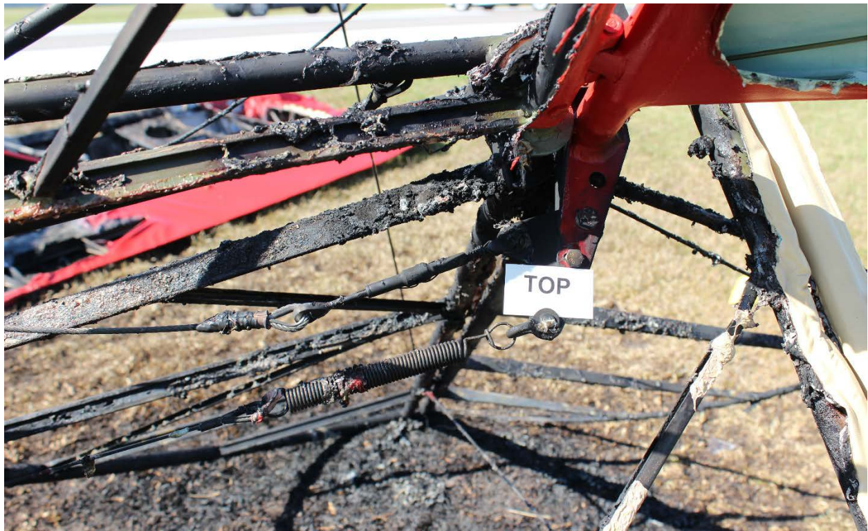
Figure 3 The reversed elevator cables.
