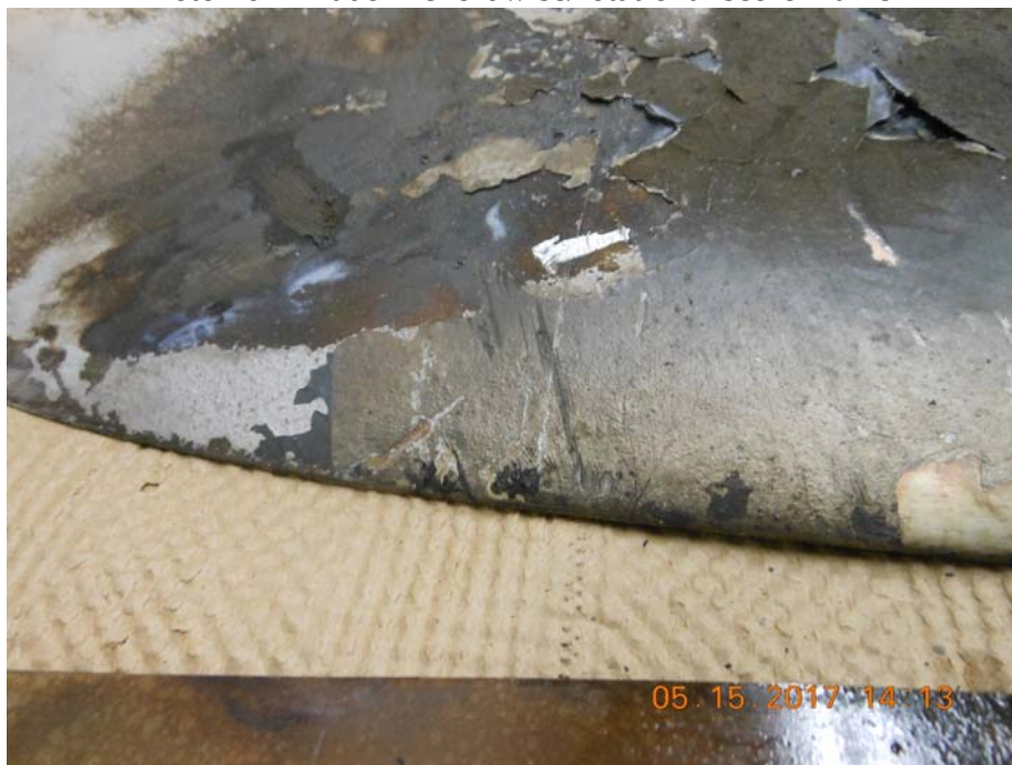
Photo #6 – Blade B chordwise/rotational score marks
