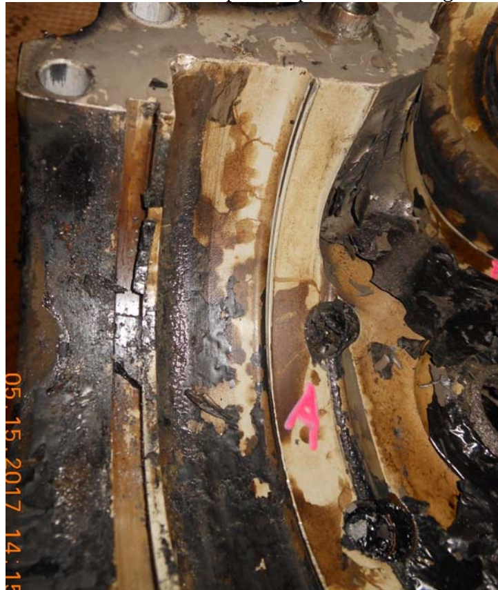
Photo #4 – Blade A preload plate shelf damage
