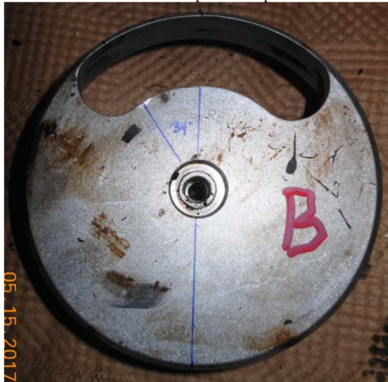
Photo #5 – Preload plate B impact mark
