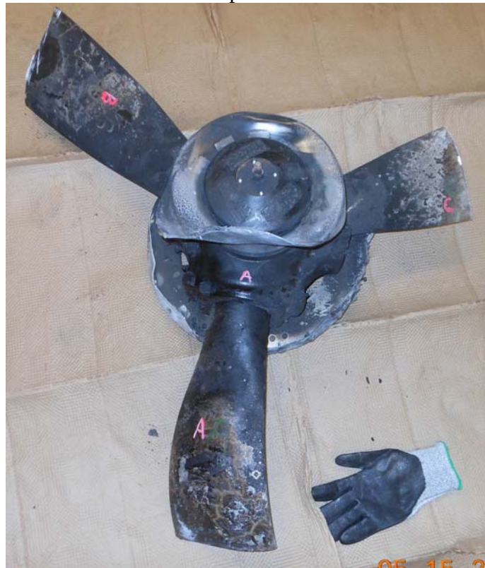
Photo #1 – Propeller As-Received
