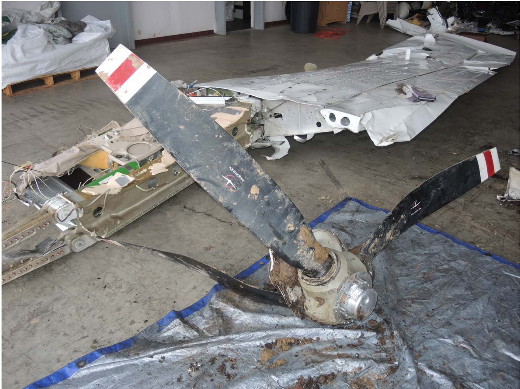
Photo 8 – View of damaged 3-bladed propeller
