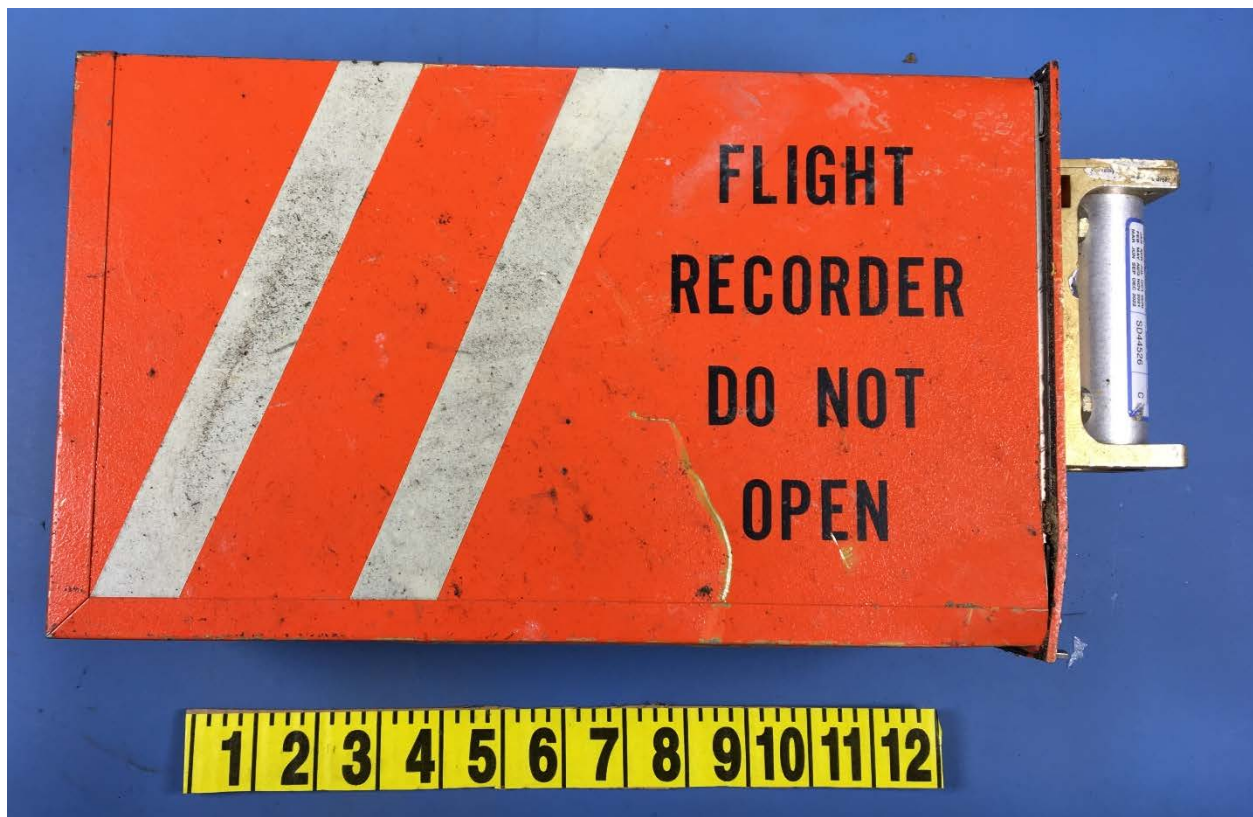
Figure 1. CVR, as received, showing impact damage.
