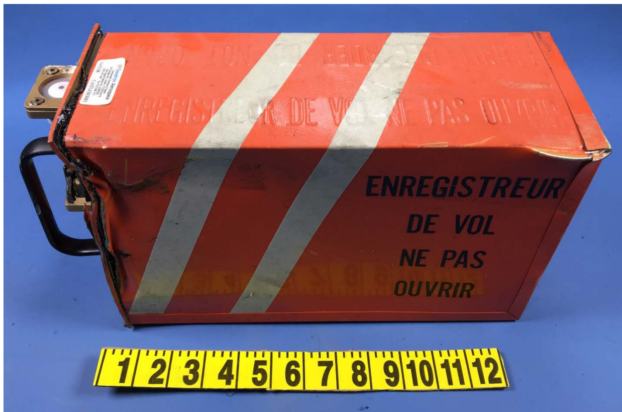
Figure 2. CVR, as received, showing impact damage.
