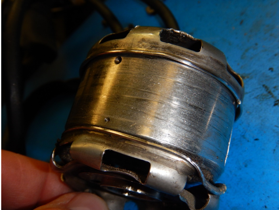
Figure 7 - Rotor removed from Vertical Gyro Number 1 (after cleaning), showing rotational scoring.
