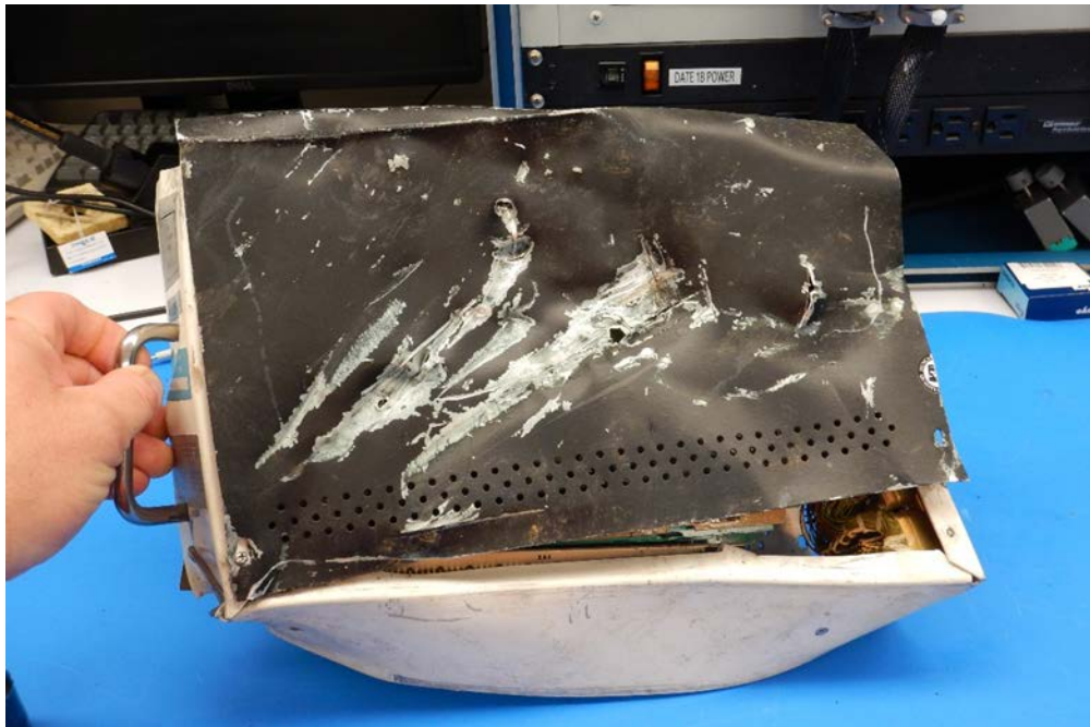
Figure 8 - The side of the Autopilot Computer, showing dust cover and chassis deformation.
