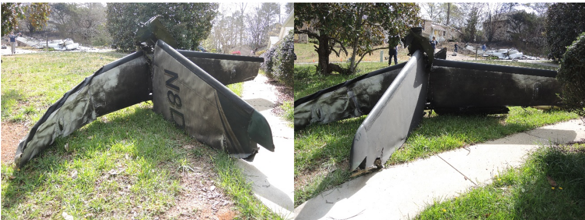
Figures 21a and 21b - Found Location of Vertical and Horizontal Stabilizers; Note Main Wreckage in Background.
