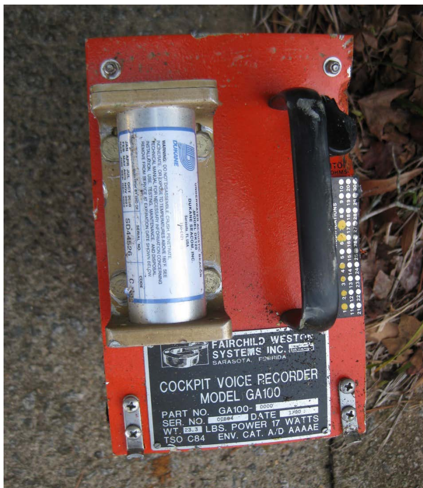
Figure 16 - The front face and data plate of the Cockpit Voice Recorder.
