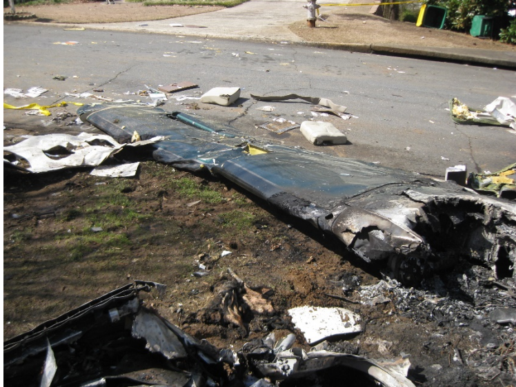
Figure 24 - Right wing, looking outboard, and noting fire at the inboard forward section.
