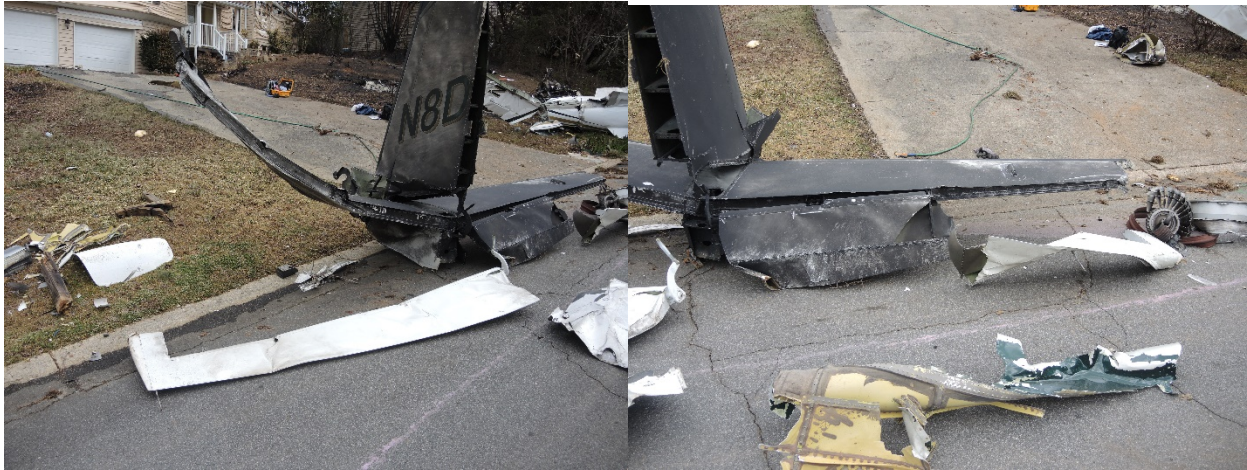
Figure 22a and 22b - The left and right elevator laid out near horizontal stabilizer.
