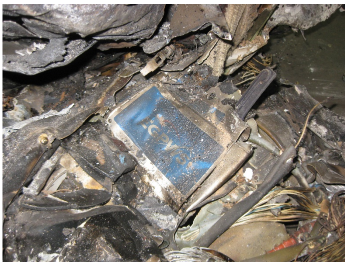
Figure 17 - The airplane's TAWS unit, prior to removal from the wreckage.
