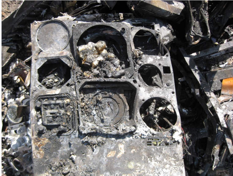
Figure 15 - The Left Main Flight Instrument Panel, as found. The Garmin GTN 750 is to the right of the panel.
