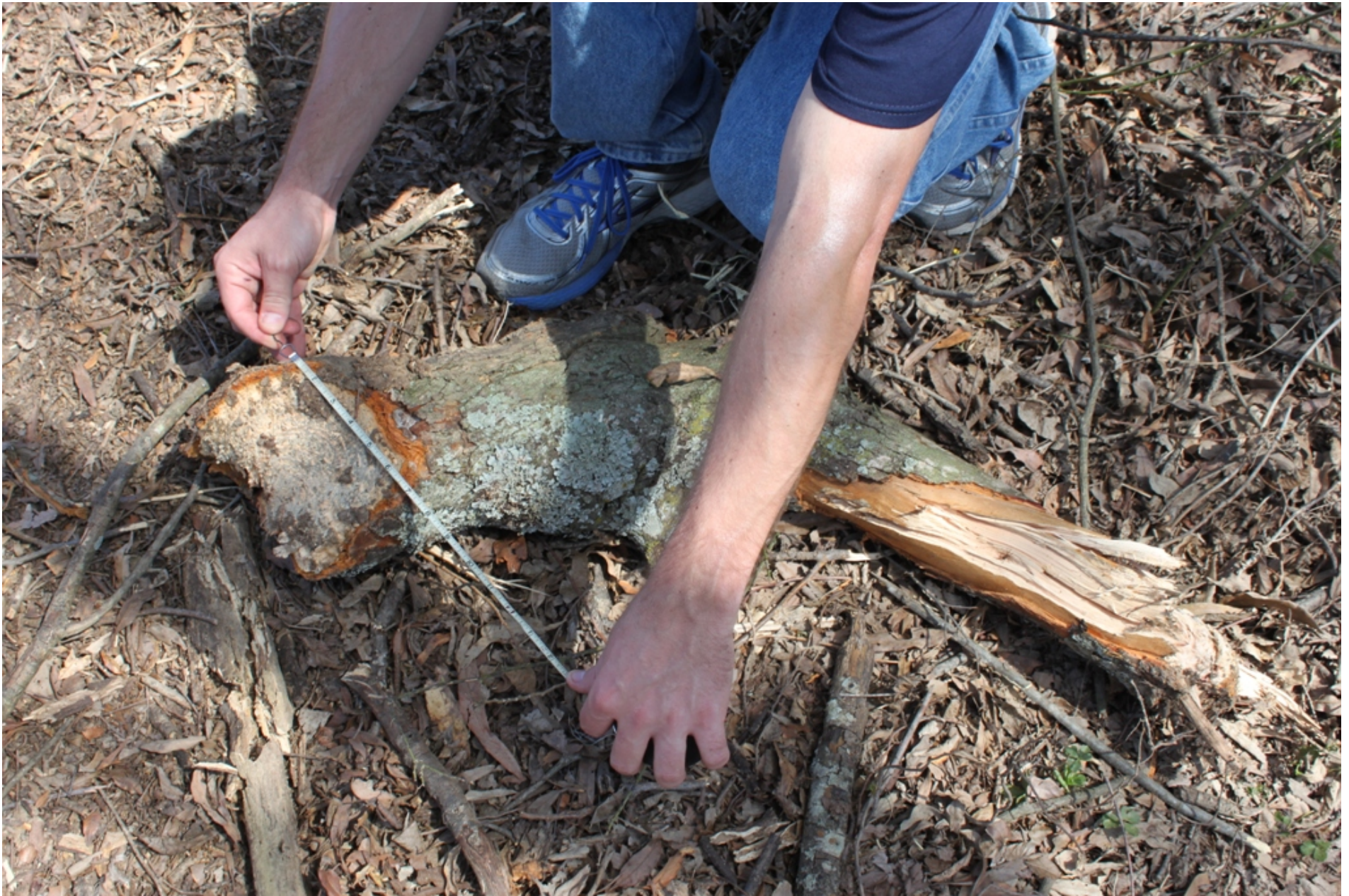
Photo 11 - NTSB Digital Photograph. View Depicting the Cut Surface With Gray Transfer of 7 Inch Diameter Tree Trunk
