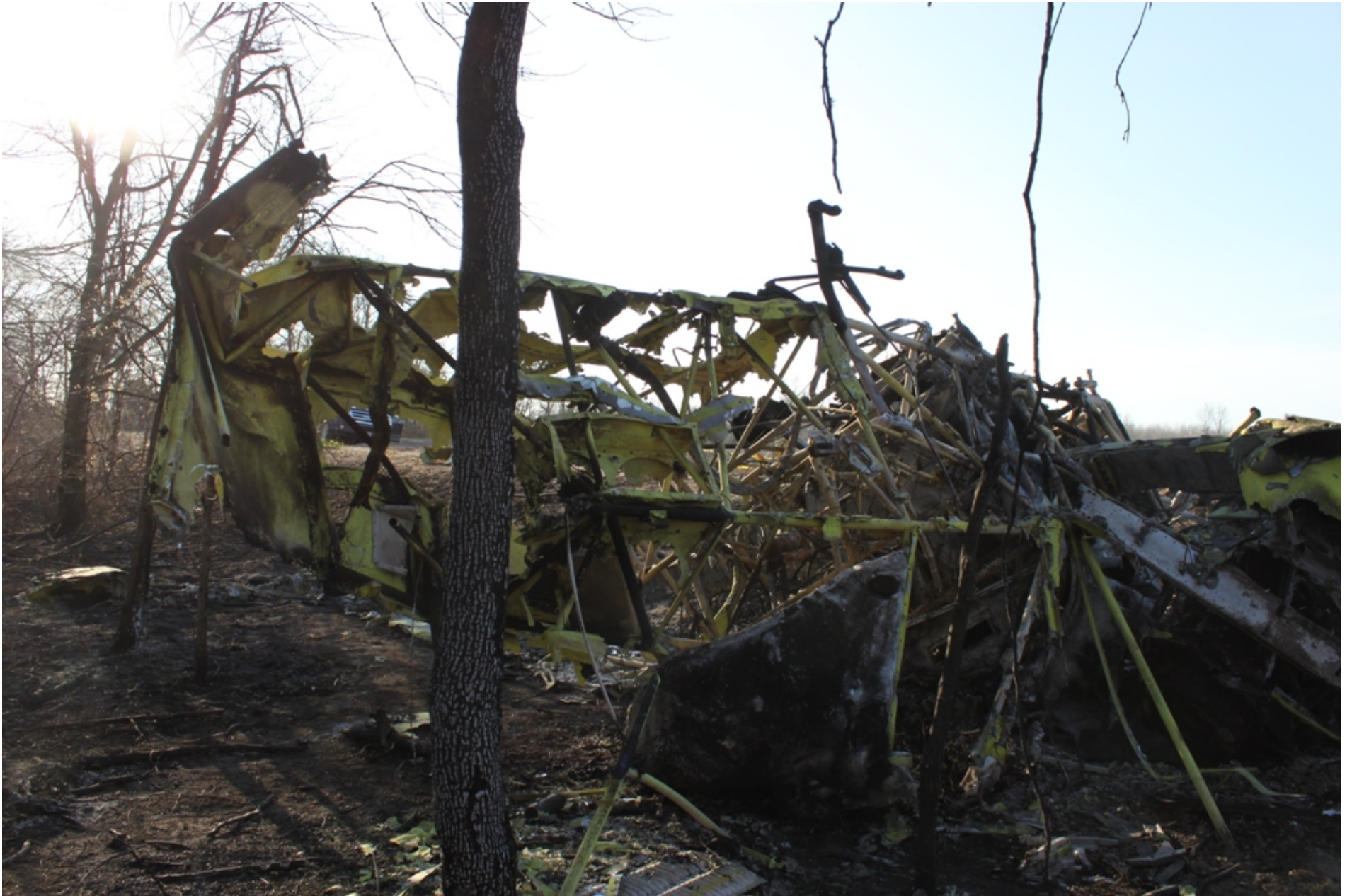
Photo 6 - NTSB Digital Photograph. Another View of the Heat Damaged Fuselage
