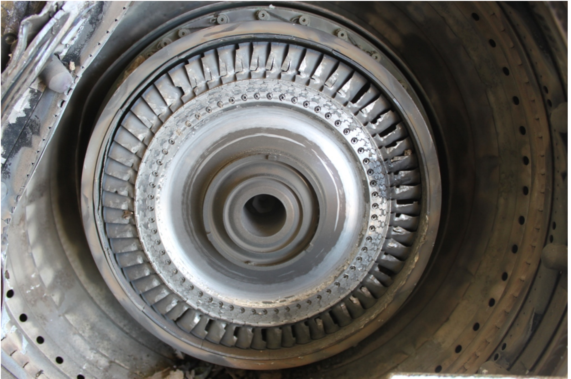
Photo 16 - NTSB Digital Photograph. Close-Up View of the Downstream Side of the Compressor Turbine. Note the Circumferential Damage to the Disk and Blades
