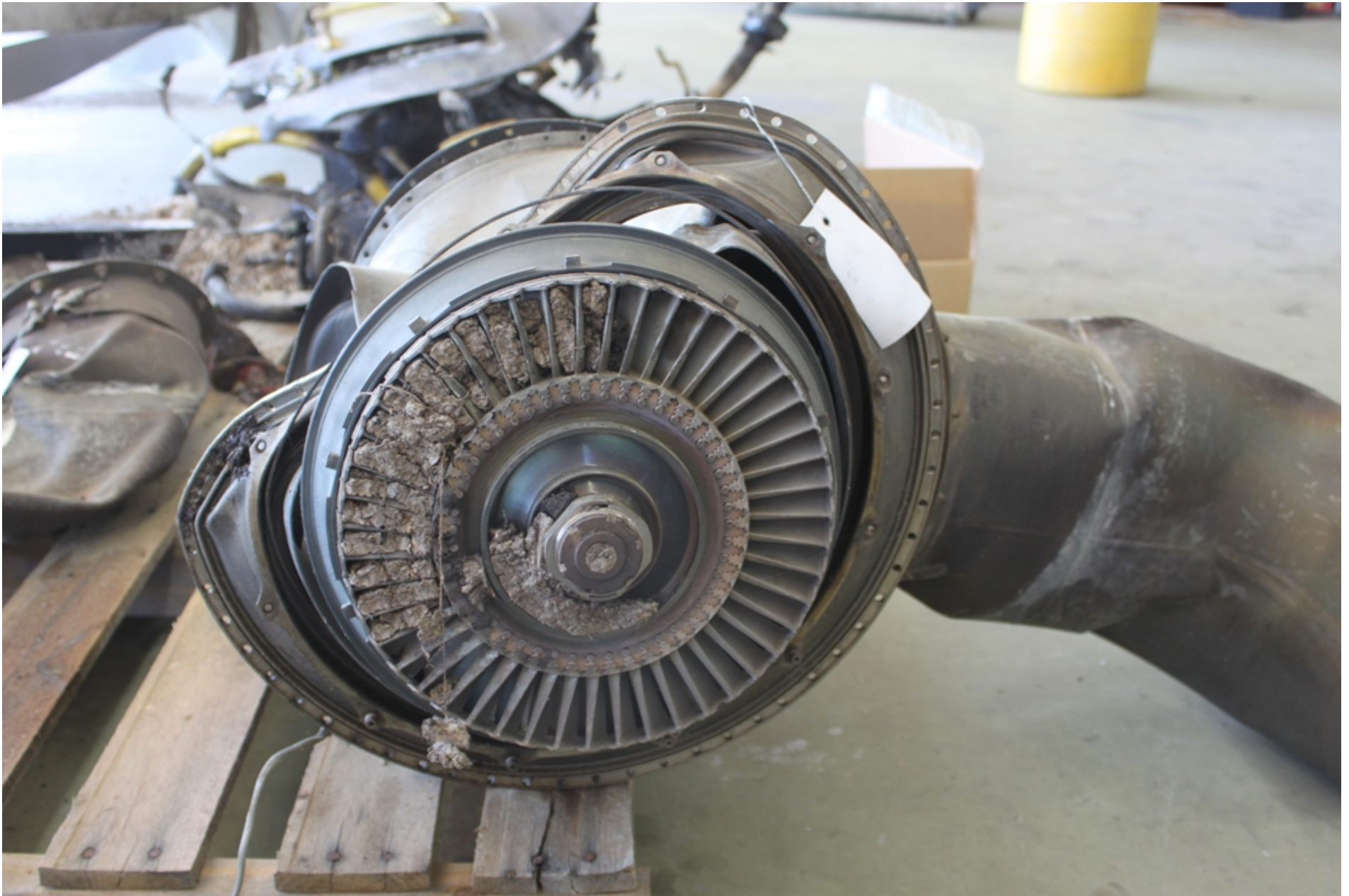
Photo 17 - NTSB Digital Photograph. Close-Up View of the 1st Stage Power Turbine. Note the Impacted Earth.
