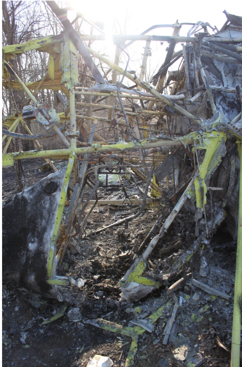
Photo 8 - NTSB Digital Photograph. View of the Cockpit Area of the Fuselage. Note the Minimal Distortion of the Occupiable Space
