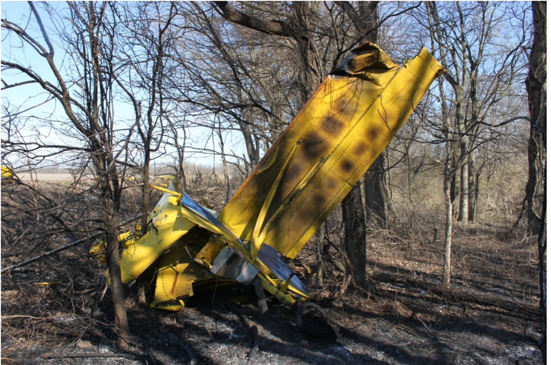
Photo 4 - NTSB Digital Photograph. View of the Empennage. Note the Heat Damage to the Ground Area Adjacent to the Empennage
