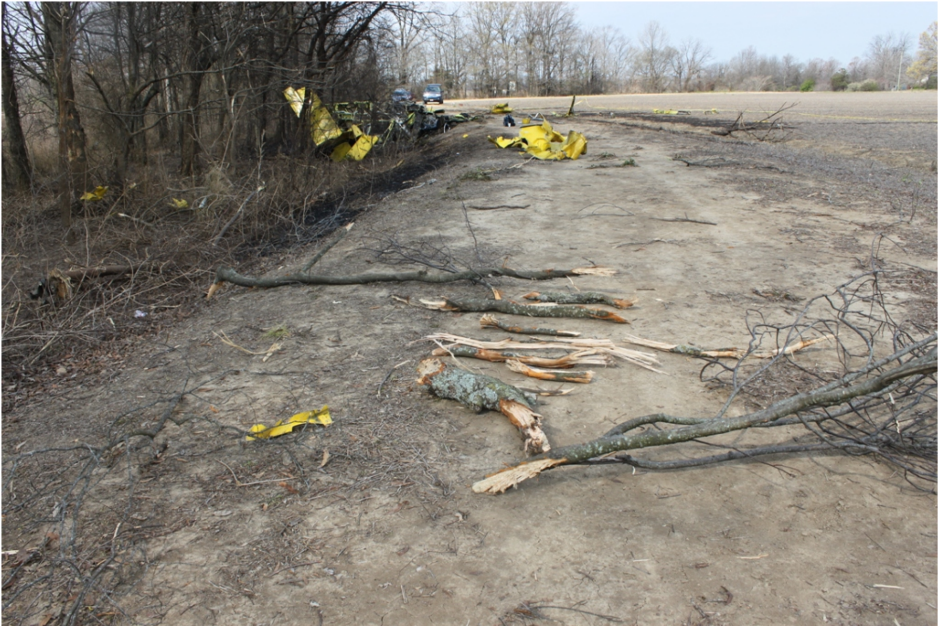
Photo 10 - NTSB Digital Photograph. View Depicting the Recovered Tree Limbs of Various Diameters and Trunk That Exhibited Cut Surfaces Consistent with Propeller Blade Contact
