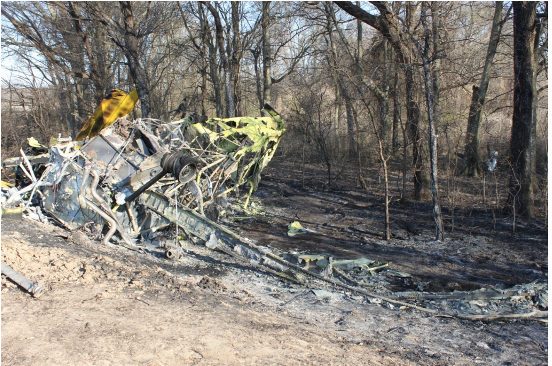
Photo 5 - NTSB Digital Photograph. View of the Heat Damaged Fuselage and Partial View of the Right Wing Spar
