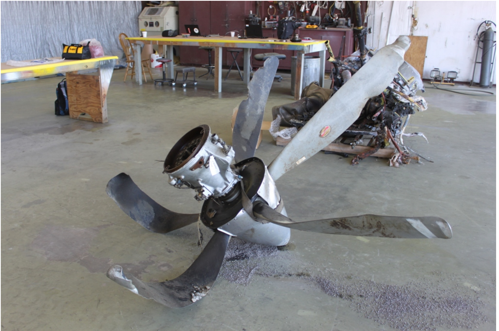
Photo 18 - NTSB Digital Photograph. View of the Propeller. Note the Blade Bending
