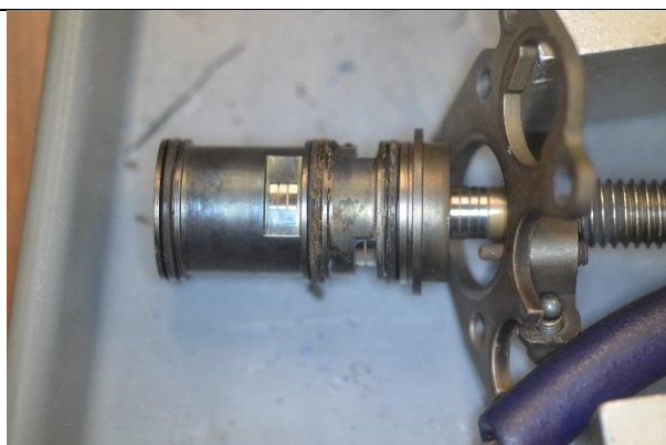
Figure 8 – Fuel Valve assembly showing heat degraded packings.
