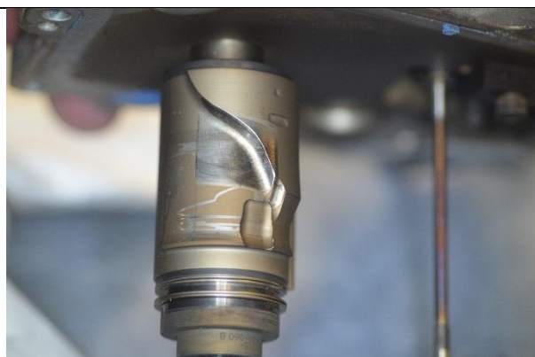
Figure 7 – Wear pattern showing operational area of cam
