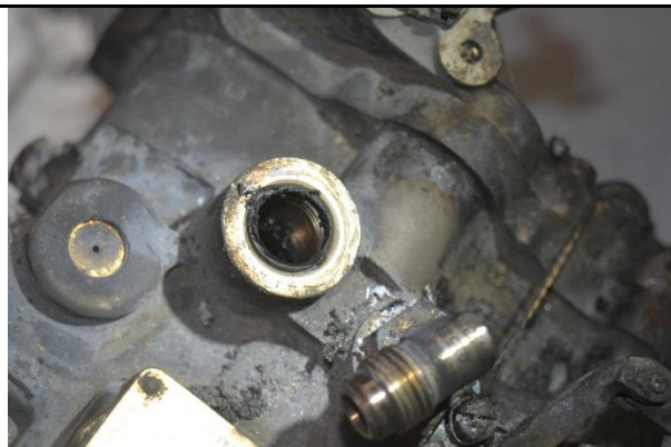
Figure 3 - Typical port with degraded seal visible
