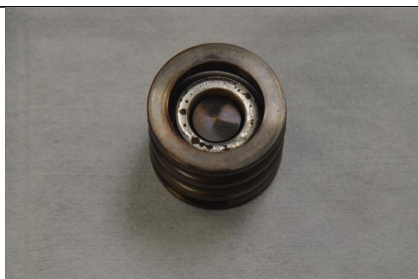
Figure 5 – Remainder of bellows showing other side of re-flowed solder joint
