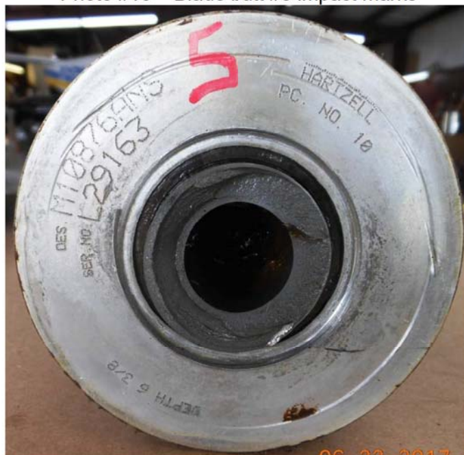
Photo #10 – Blade butt #5 impact marks
