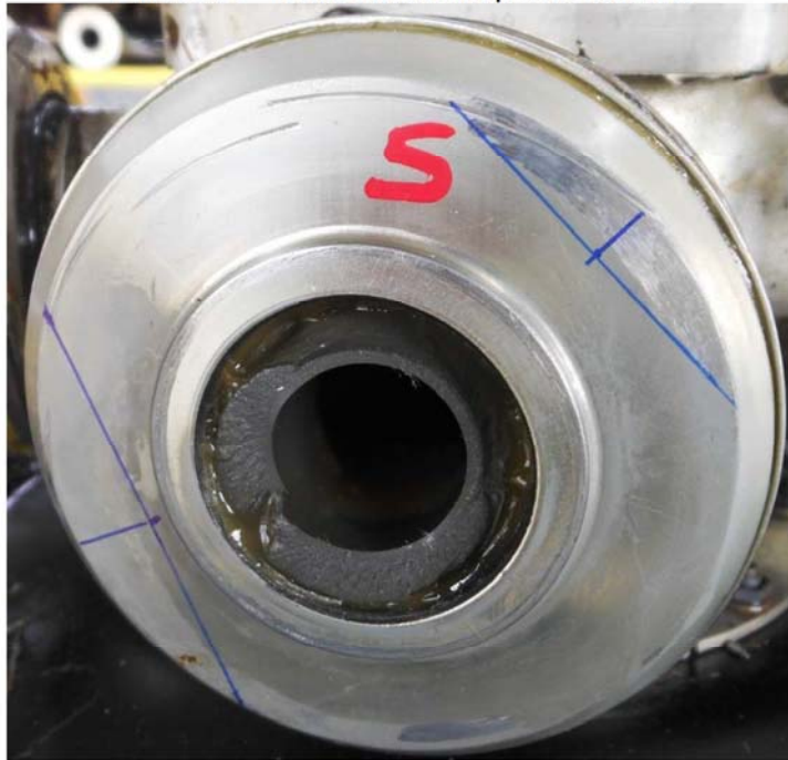
Photo #9 – Hub arm #5 impact crescent
