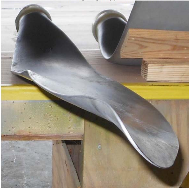
Photo #14 – Blade #2 leading edge, typical tree strike wave/bends
