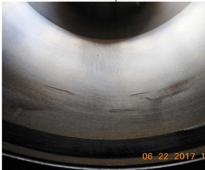
Photo #4 – Internal piston marks
