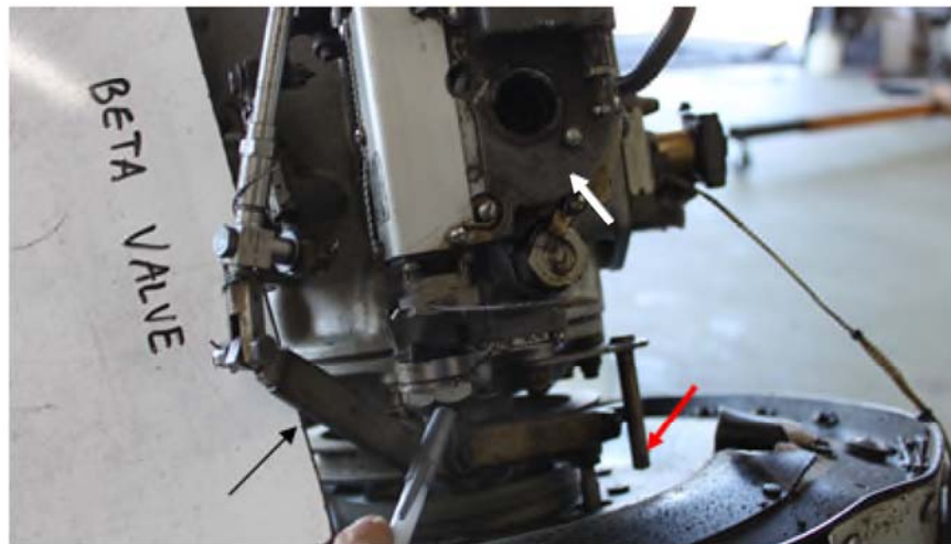
Photo No. 10 Beta guide pin and the propeller reversing lever
