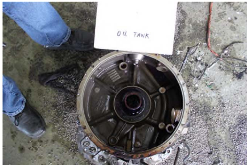
Photo No. 62 Accessories gearbox main oil tank
