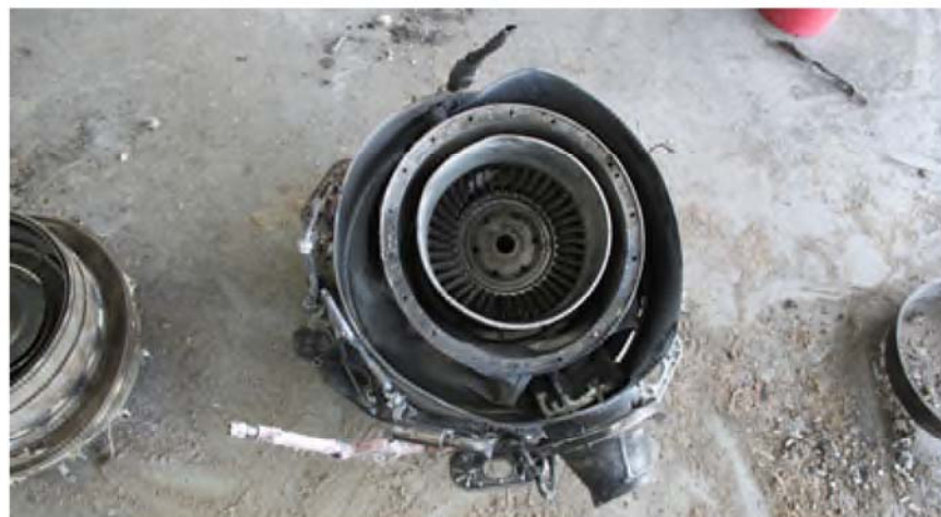
Photo No. 8 First stage compressor stator
