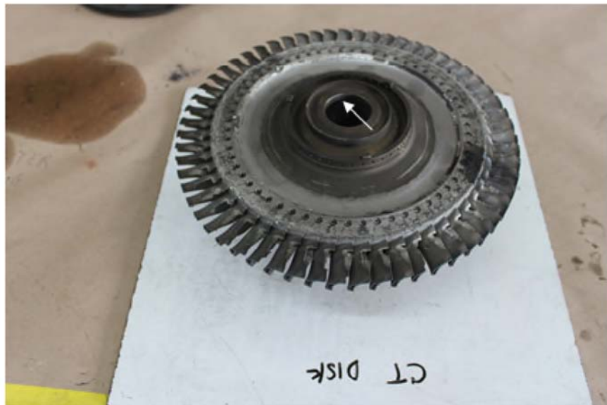
Photo No. 48 Compressor turbine disc inner diameter surface adjacent the retention bolt bore
