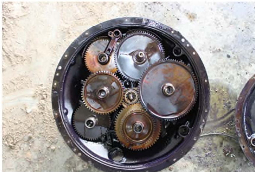
Photo No. 63 Accessories gearbox gear train
