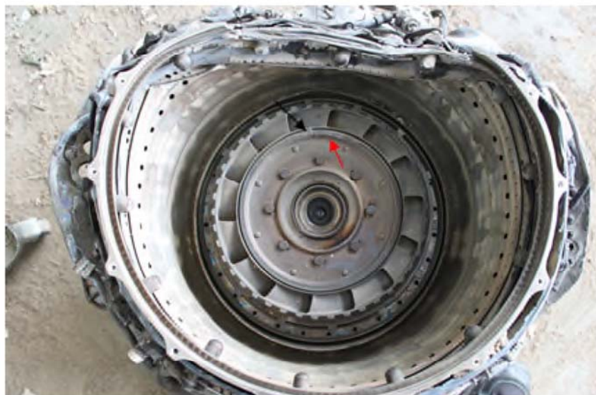
Photo No. 42 Downstream view of compressor turbine stator and fuel nozzles
