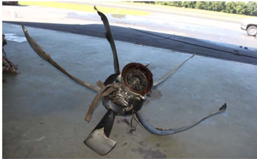
Photo No. 1 Propellers and front reduction gearbox housing
