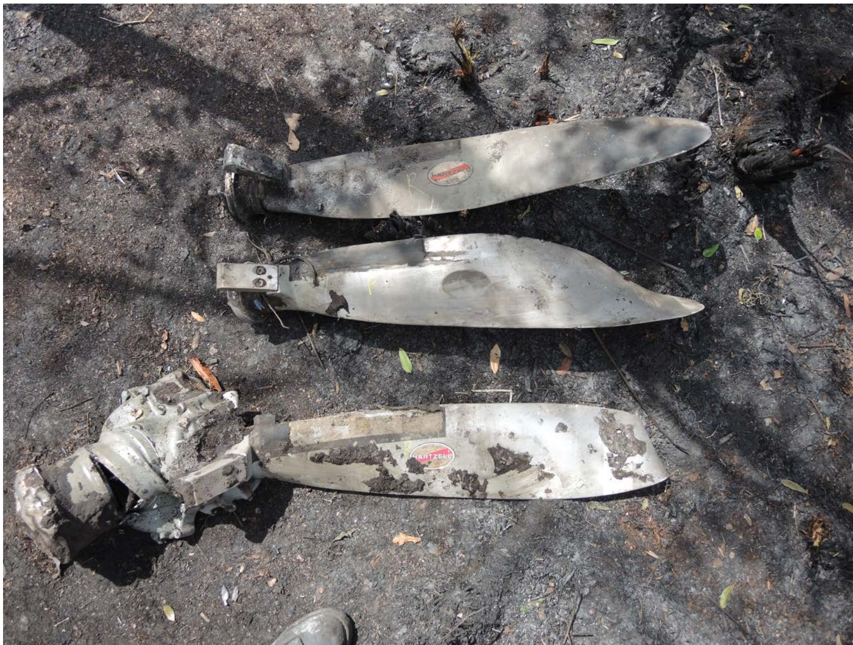
Photo 3 – View of Right Engine Propeller Blades after Recovery (Textron)
