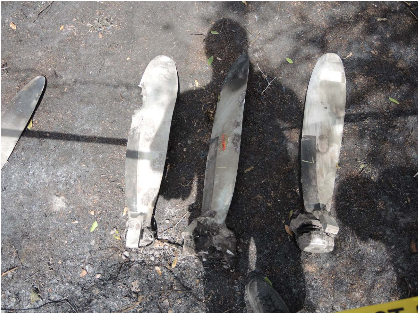
Photo 4 - View of Left Engine Propeller Blades after Recovery (Textron)
