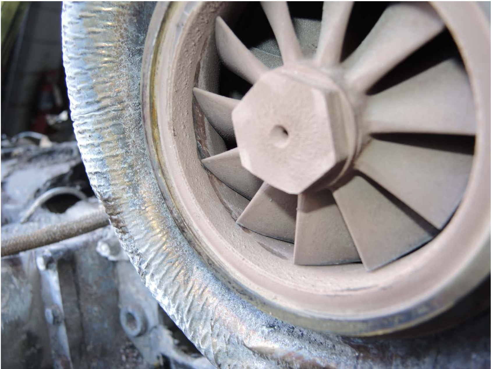
Photo 5 – View of Left Engine Turbocharger Impeller (Textron)
