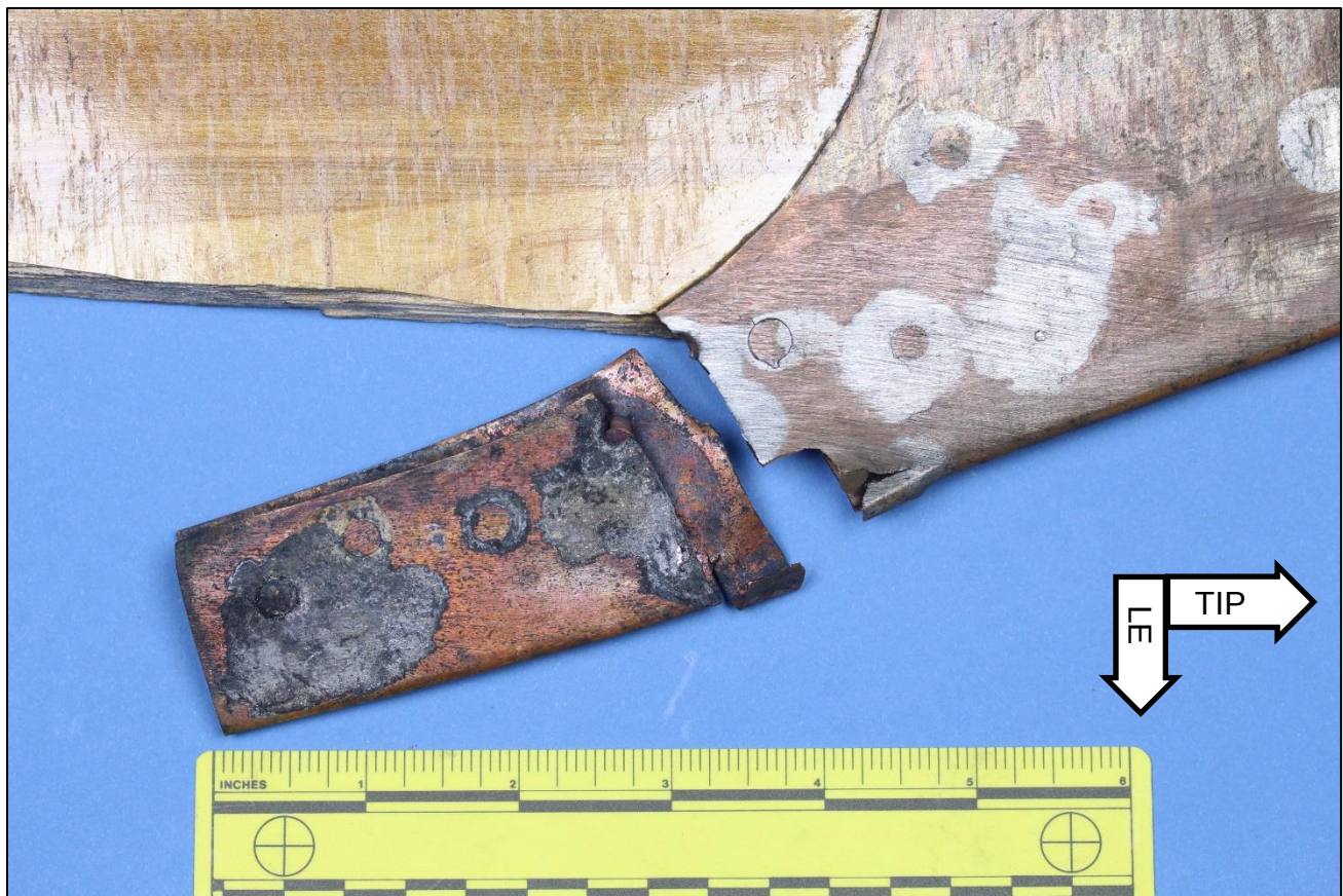
Figure 2. Mating sides of the copper leading edge fracture in blade A showing the aft (pressure) face of the blade.
