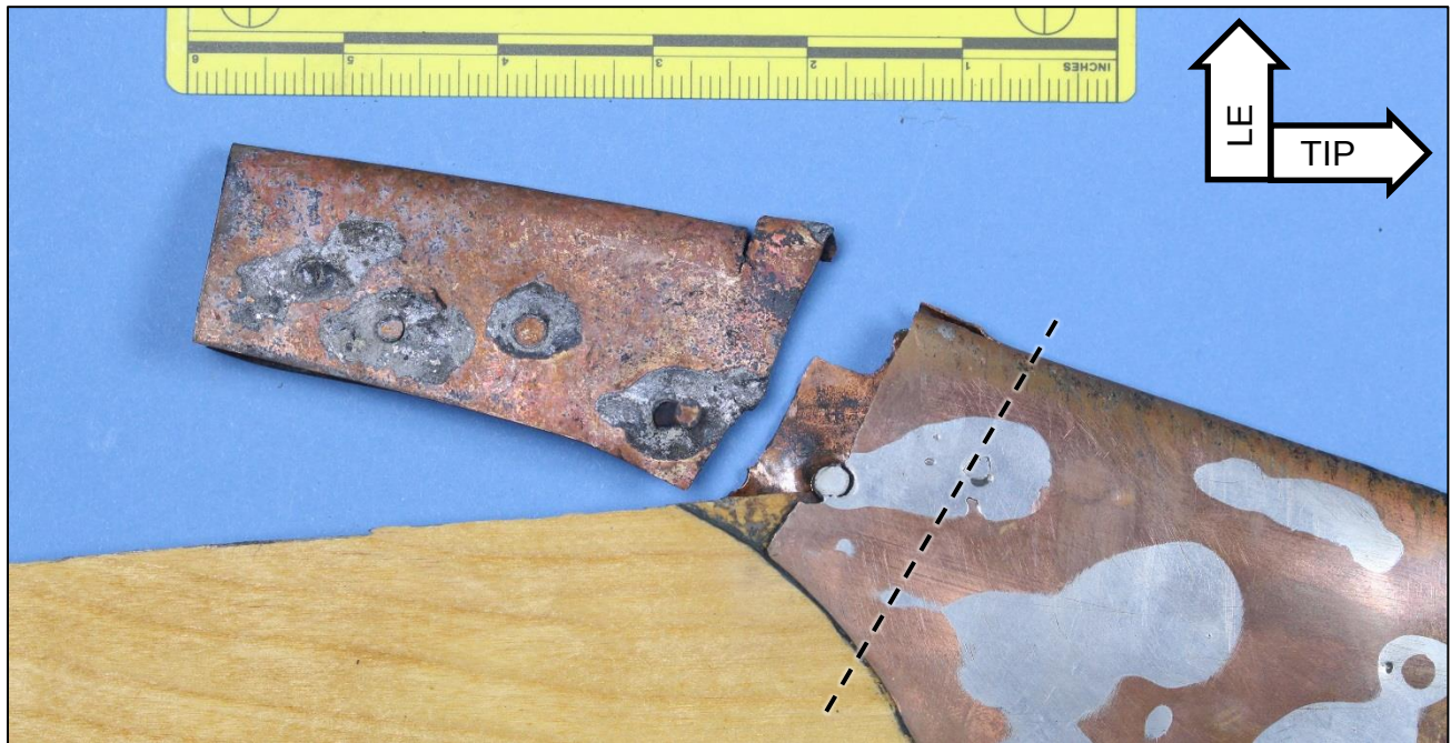
Figure 3. Mating sides of the copper tip and leading edge fracture in blade A showing the forward (suction) face of the blade. A dashed line indicates the approximate location where the leading edge was cut to facilitate further examination of the fracture surface.
