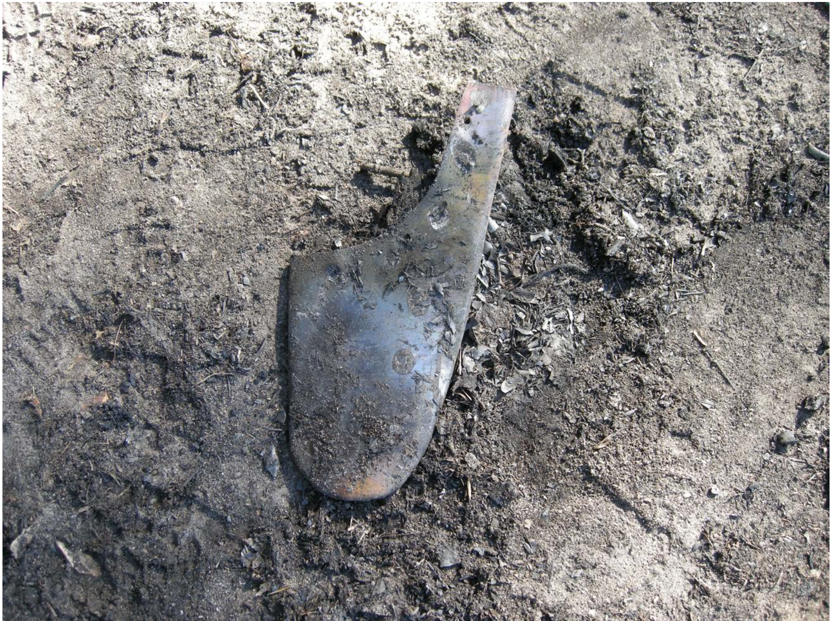
Photo 10 – Propeller Tip (NTSB Photo)
