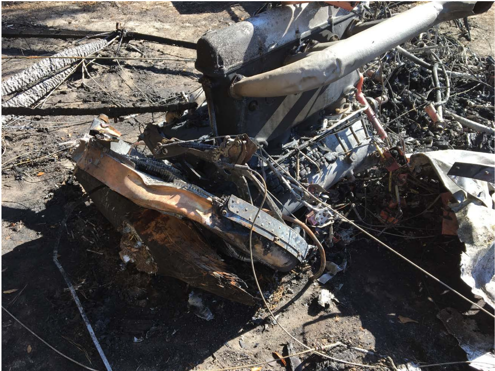
Photo 8 – Propeller Hub, Radiator, and Engine (NTSB Photo)
