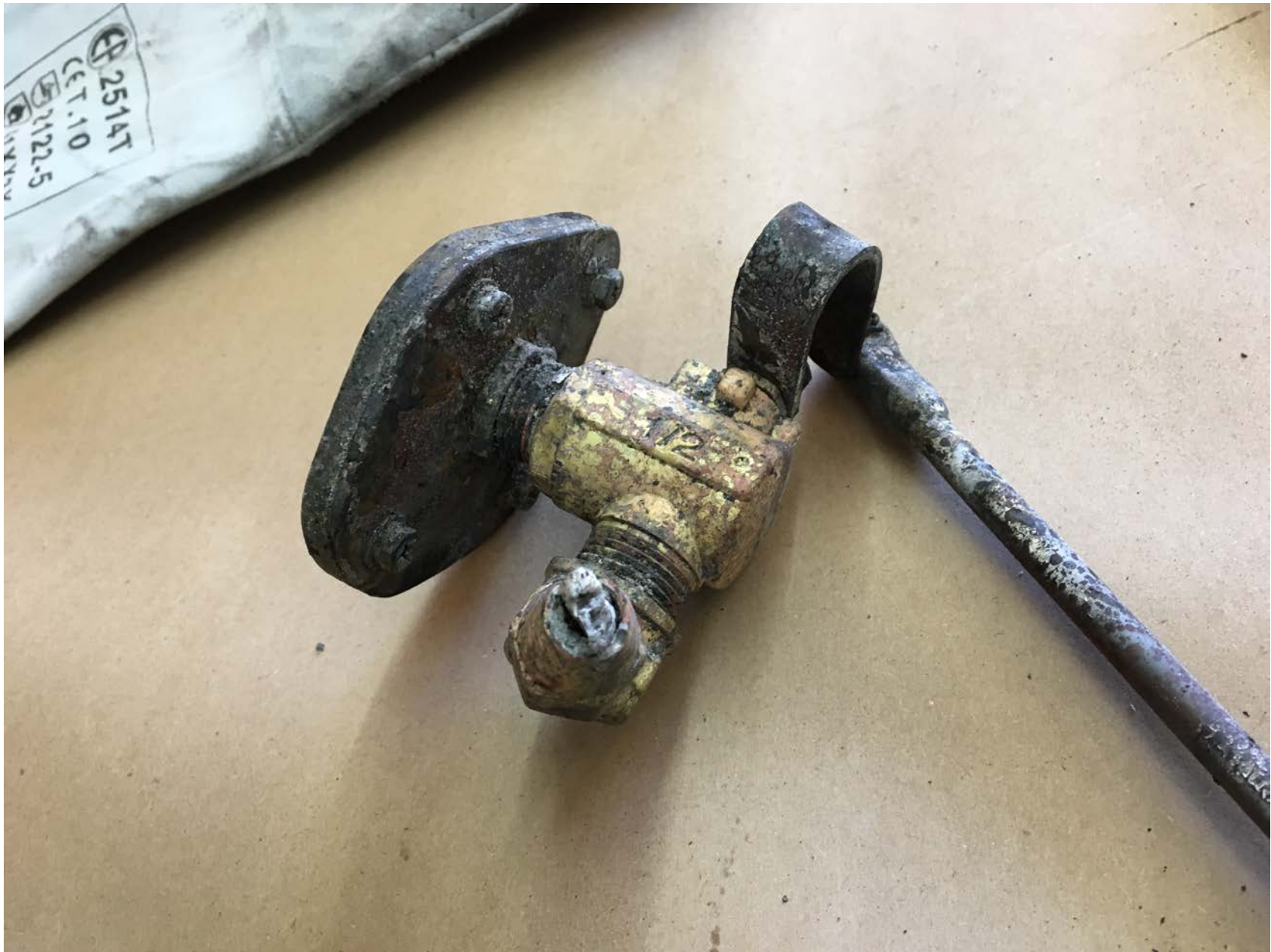
Photo 11 – Fuel Valve (NTSB Photo)
