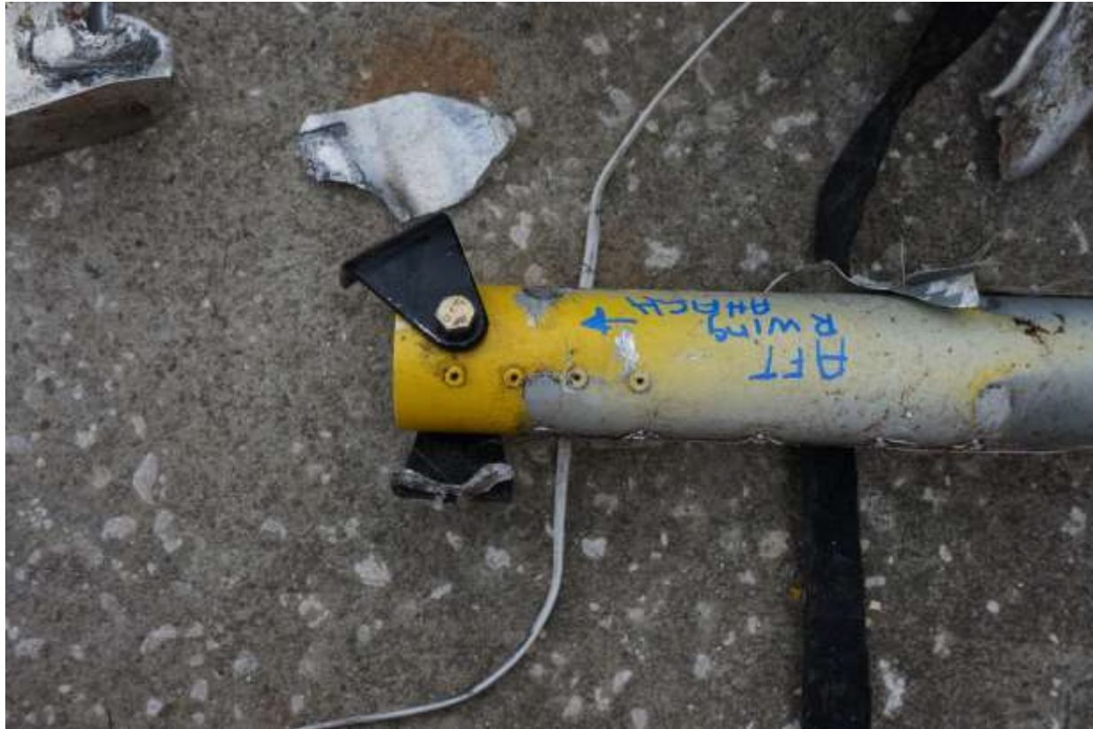
Photo 4 – Right Wing Aft Attach “Rony” Bracket
