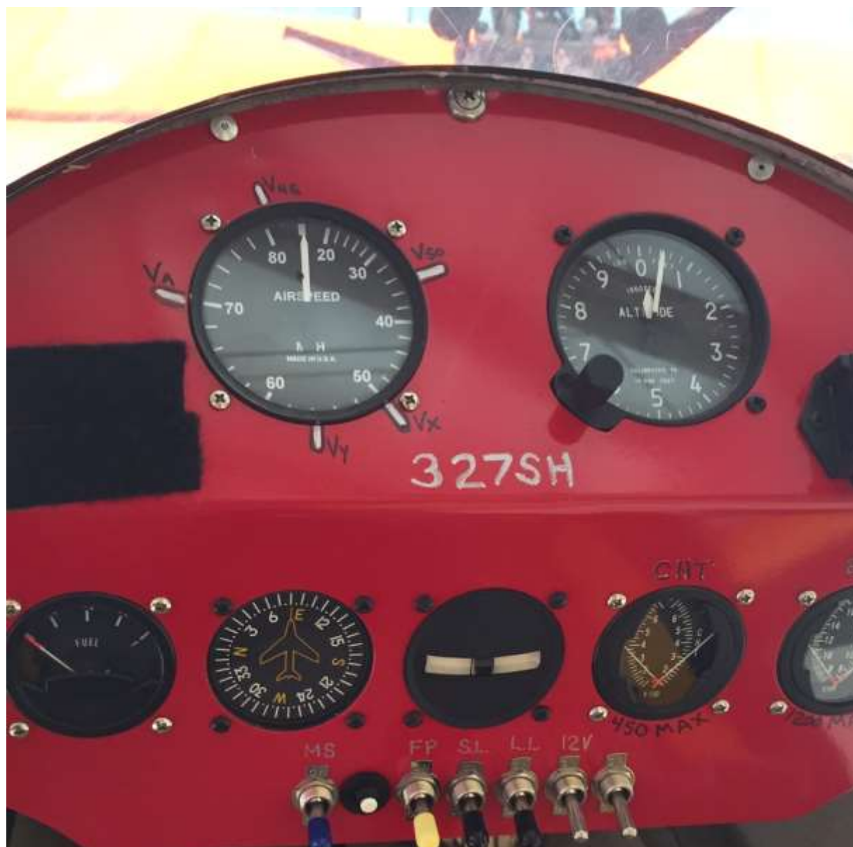
Photo 4 – Pre-accident photo of Instrument Panel – Airspeed Indicator Markings for Va and Vne
