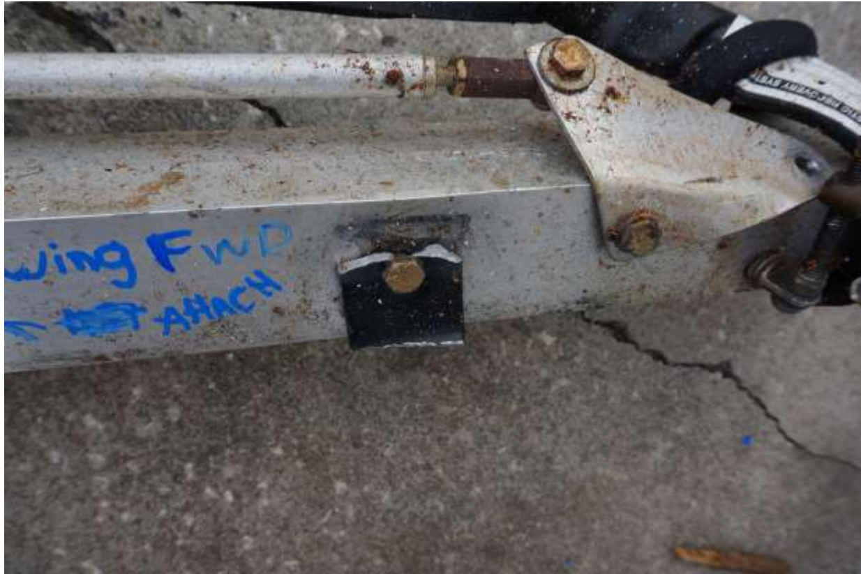
Photo 3 – Right Wing Forward Attach “Rony” Bracket
