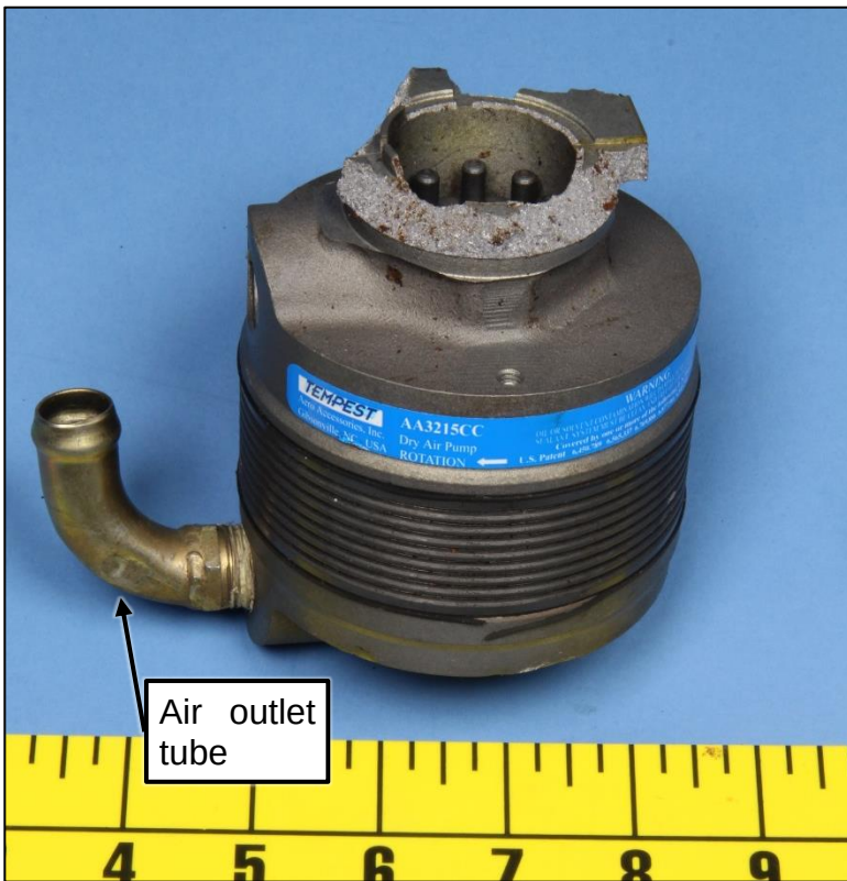
Figure 1. Overall view of the submitted vacuum pump.
