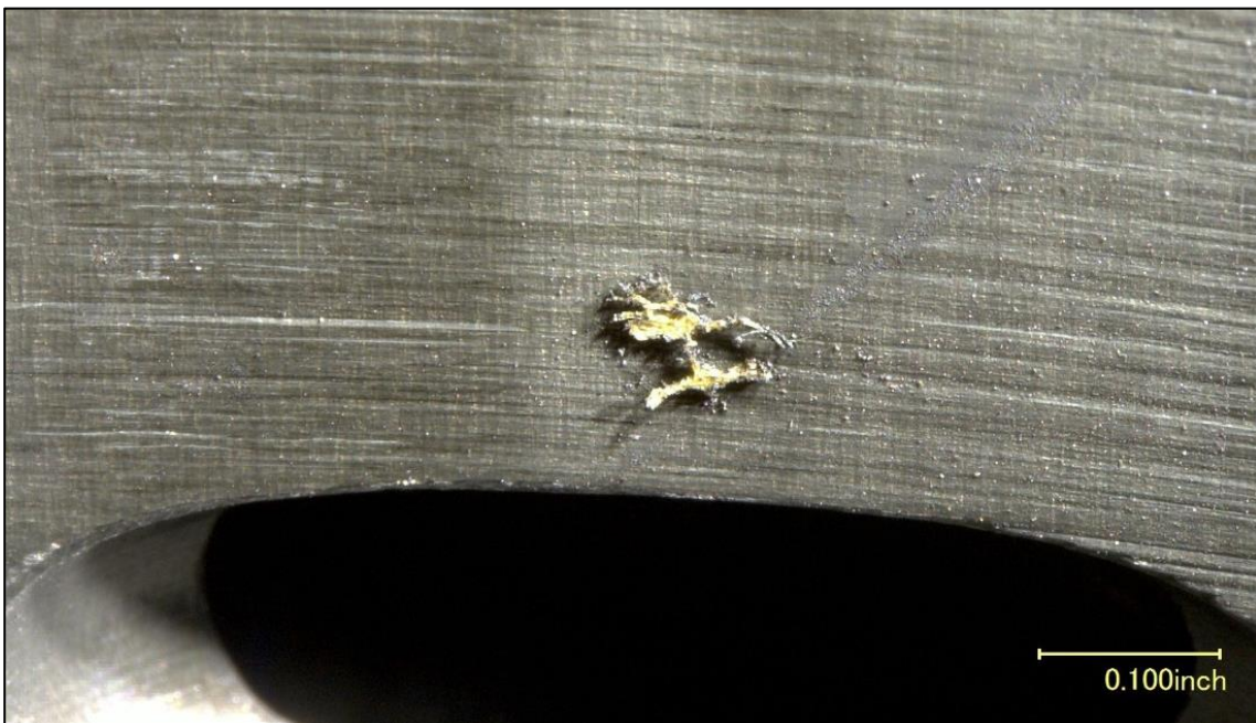
Figure 4. Piece of debris observed on the interior of the pump housing near an air outlet hole.
