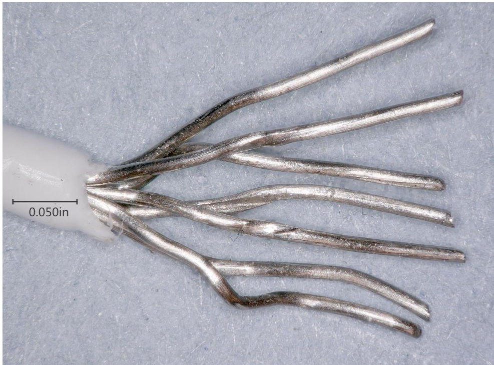
Figure 4. Power wires from separation 3, Forward wire at left, rear wire below.
