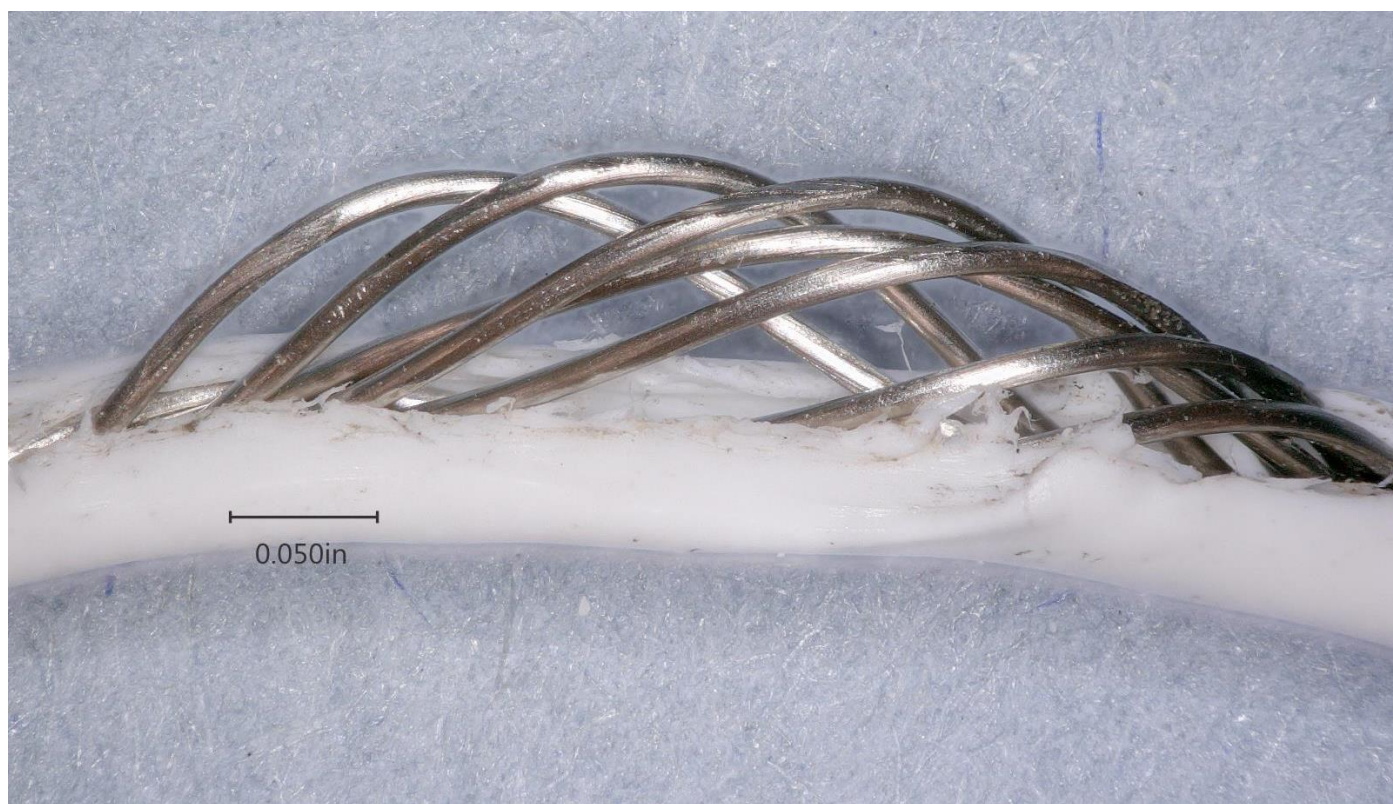
Figure 5. Two views of the exposed conductors in the forward pitot heater power wire. Lower view shows scraping damage on conductors.
