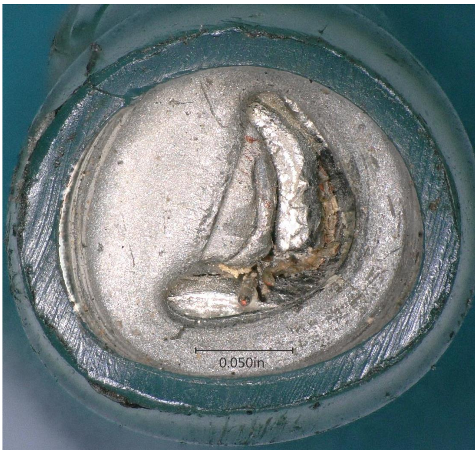
Figure 2. Wire separation 1 with tension overstress fractured wires at top and crimp at left.
