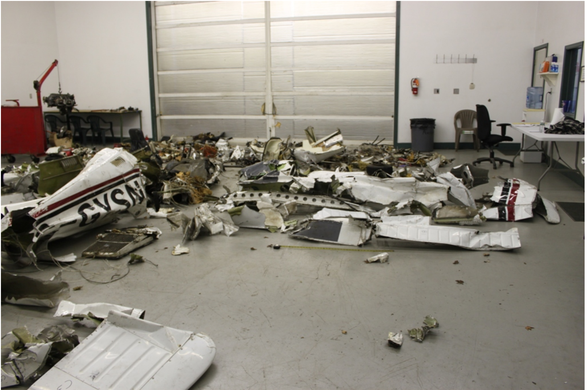
Photo 11 – NTSB Digital Photograph. Right Rear Quartering View of the Reconstructed Wreckage. Note the Fragmentation.
