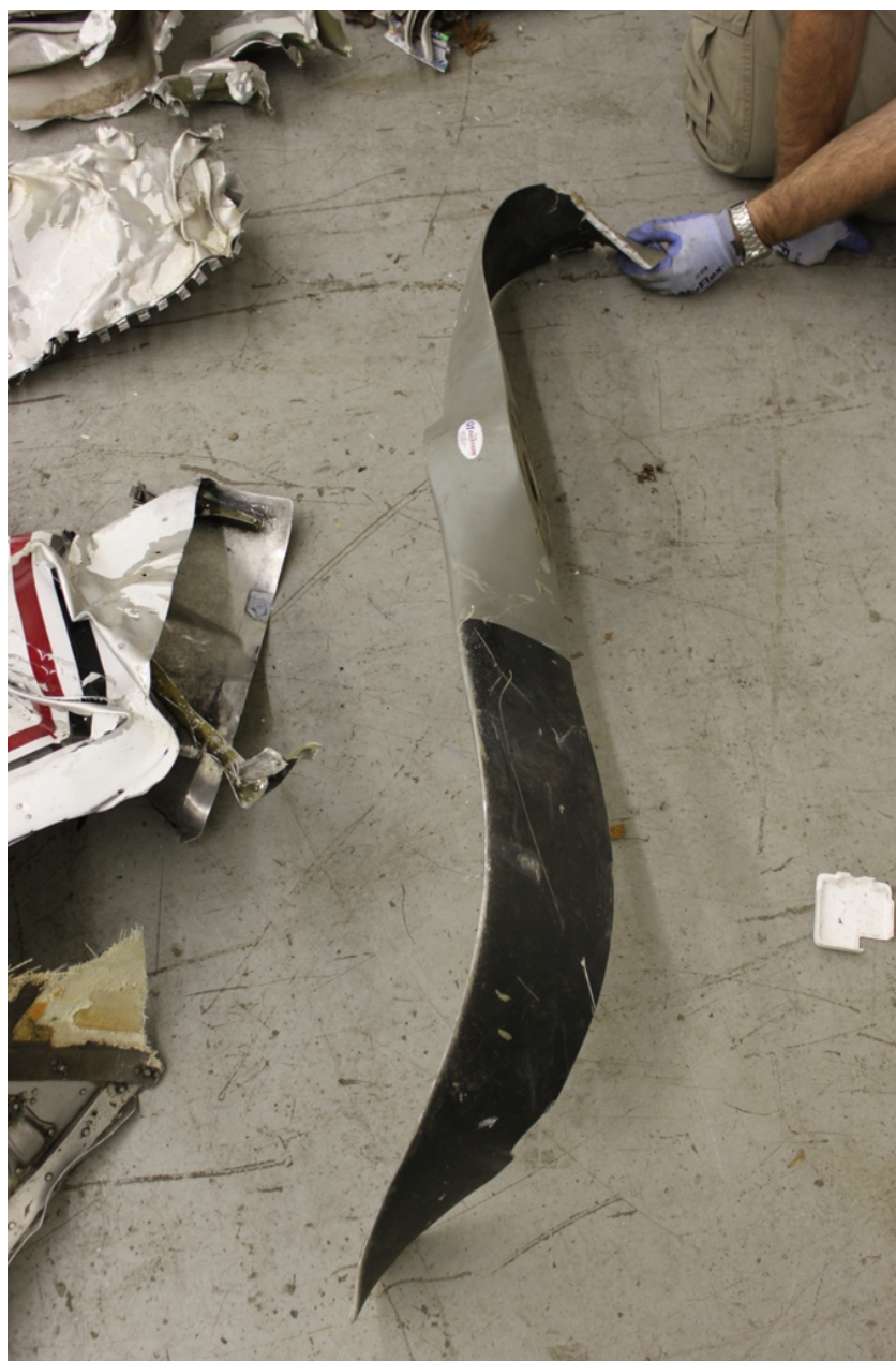
Photo 10 - NTSB Digital Photograph. View of the Propeller. Note the Blade Bending.
