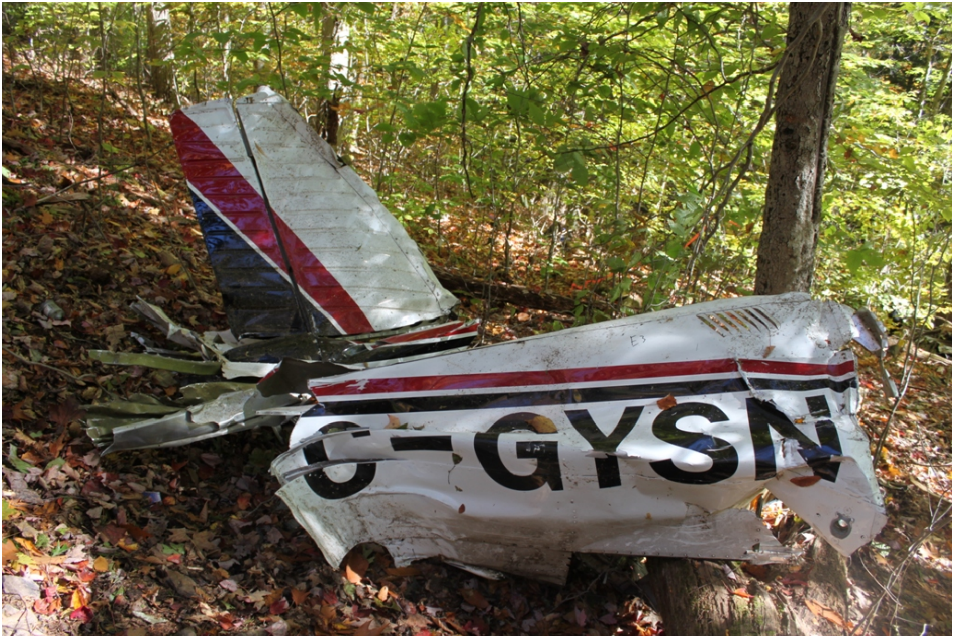
Photo 6 - NTSB Digital Photograph. Right Side View of Empennage, Vertical Stabilizer, and Rudder.
