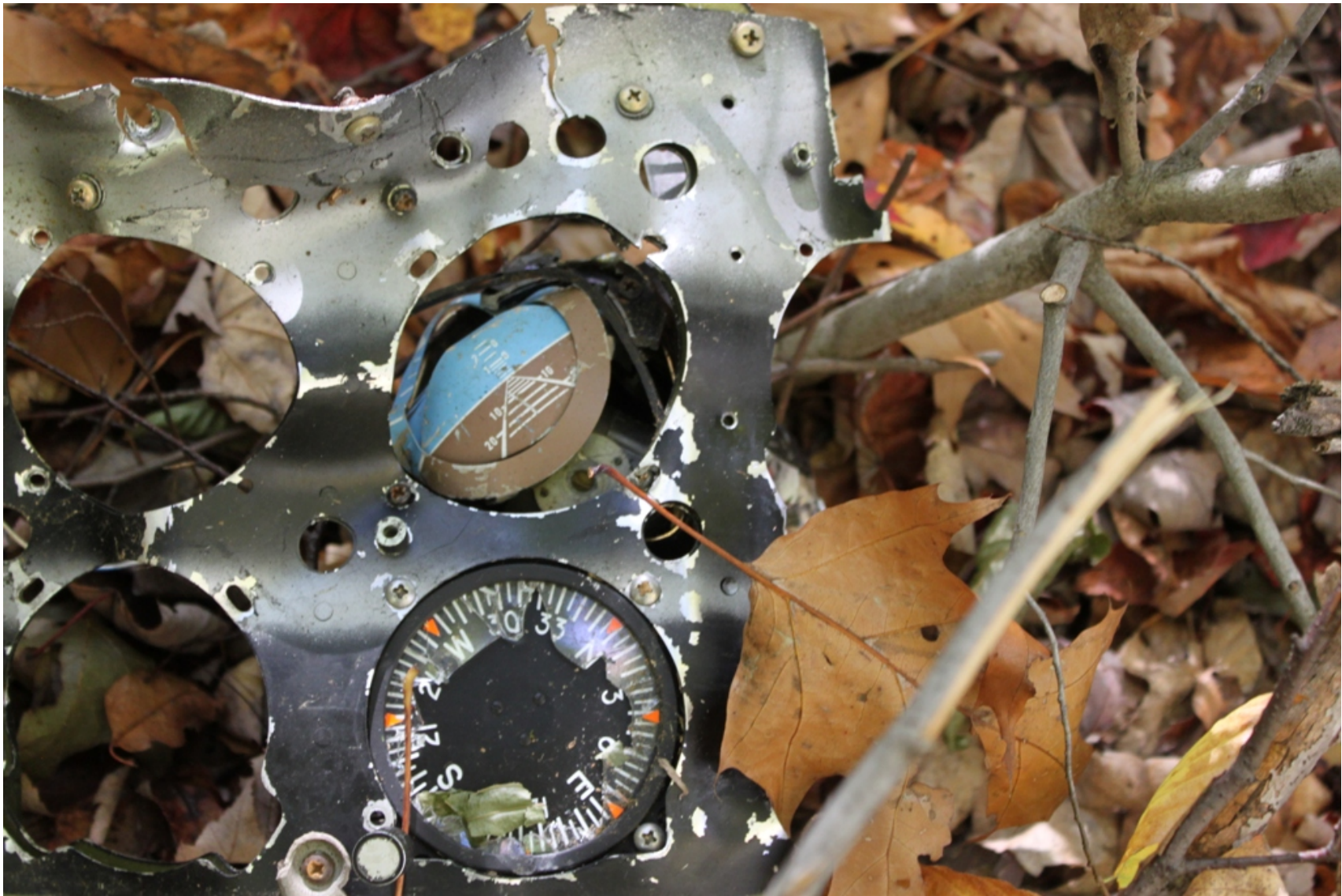
Photo 8 – NTSB Digital Photograph. View of the Separated Instrument Panel With Attached Attitude Indicator, and Directional Gyro.
