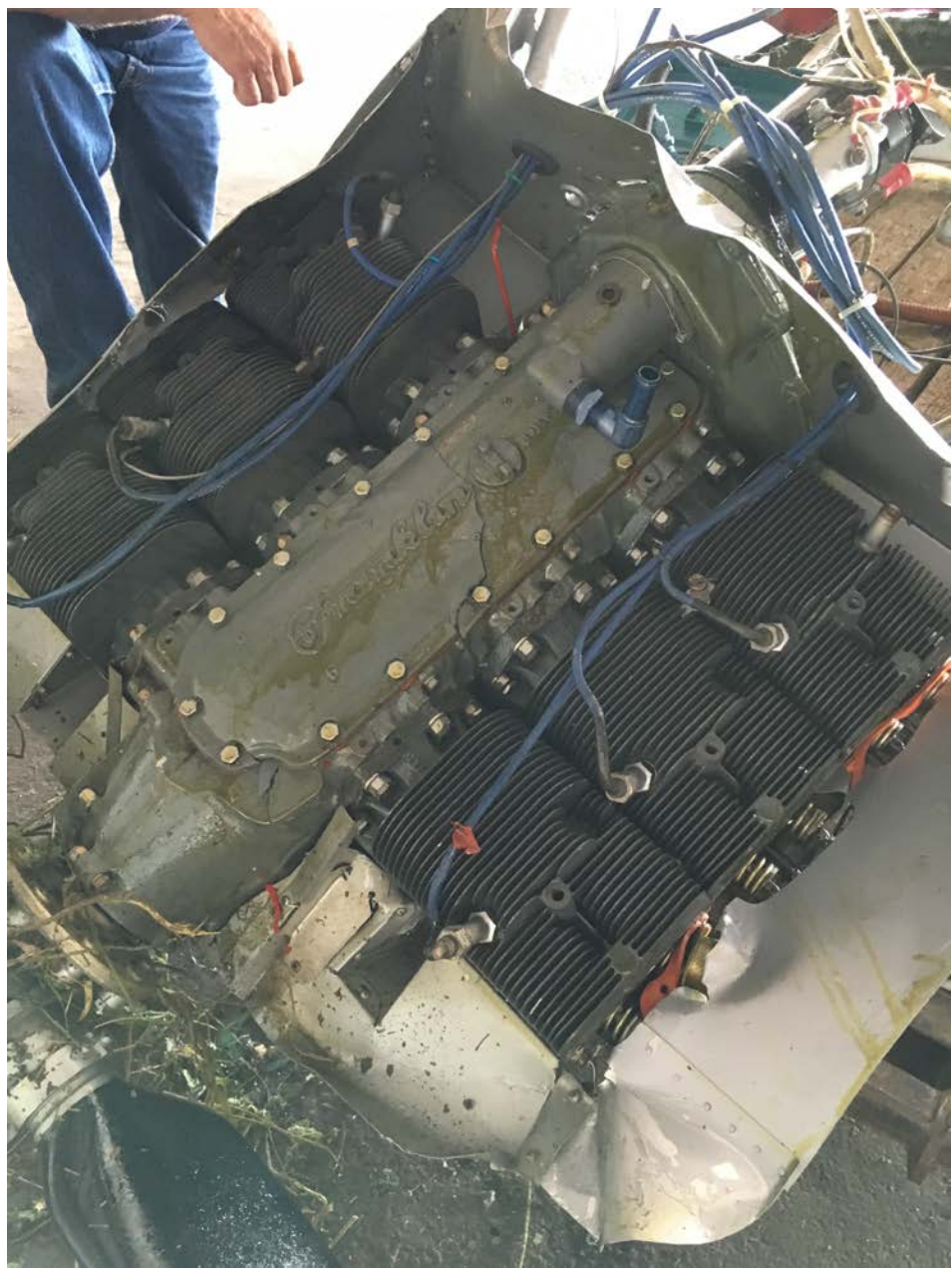
Photo 3 - View of Impact Damage to Engine Crankcase Cover
