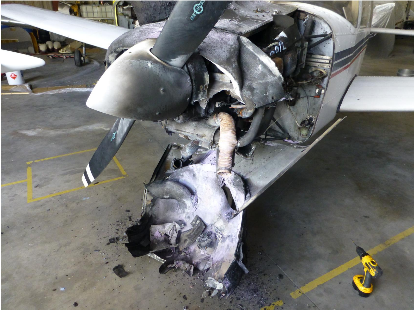
Photo 2 – engine cowling melted
