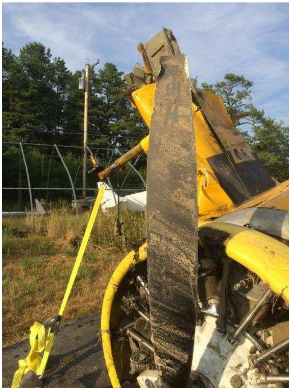
Photo 2 – Front View of Propeller with View of Damaged Right Wing in Background (Courtesy of FAA)
