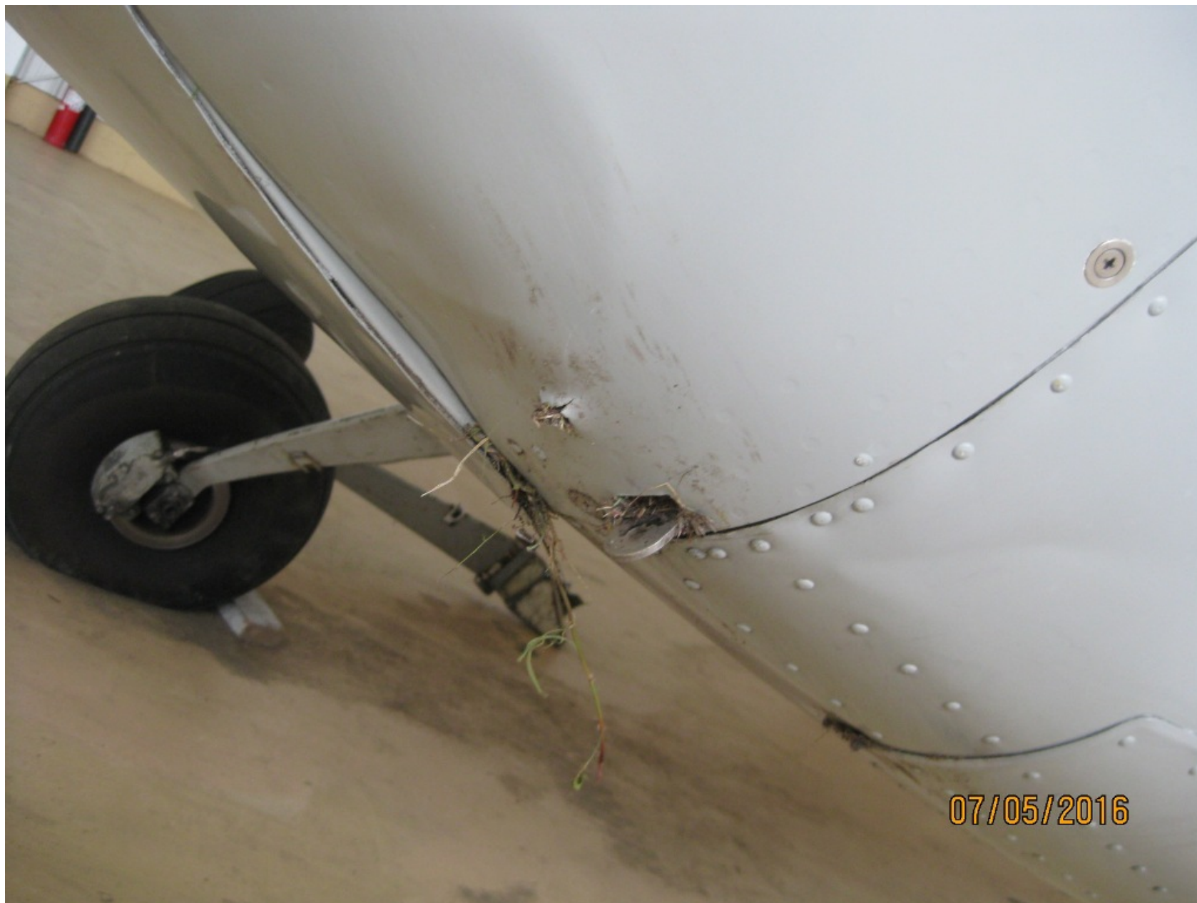
Photo 3 – Left Main Landing Gear Attachment Point (FAA Photo)
