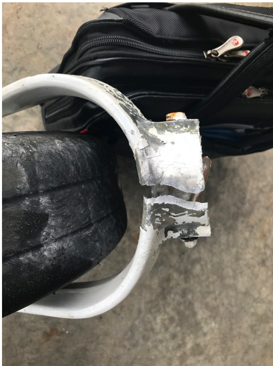
Photo 2 - Digital Photograph Provided by FAA. View of the fractured Nose Landing Gear Fork
