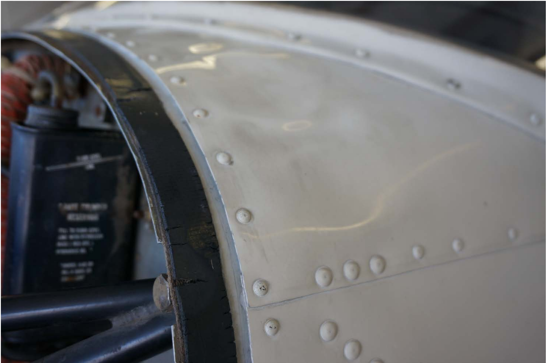
Photo 10 – Wrinkle Above Firewall
