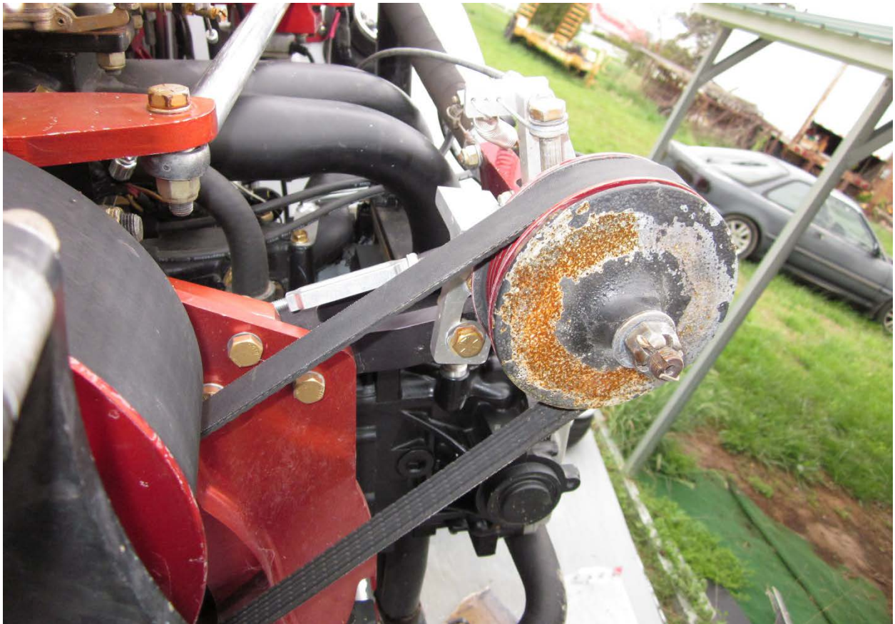
Figure 2 The adjusted prerotator motor after the accident
