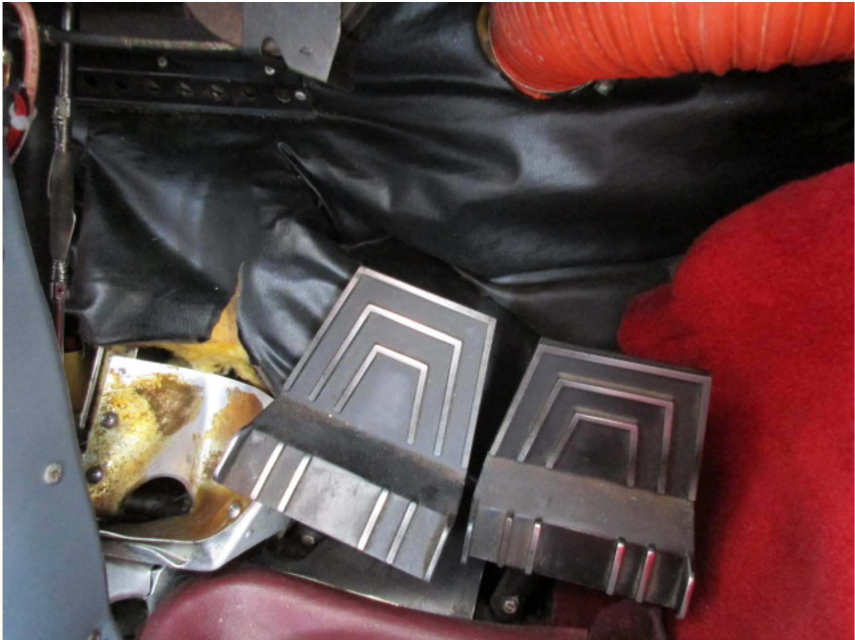
Photo 3 – FAA photo-floor board buckled
