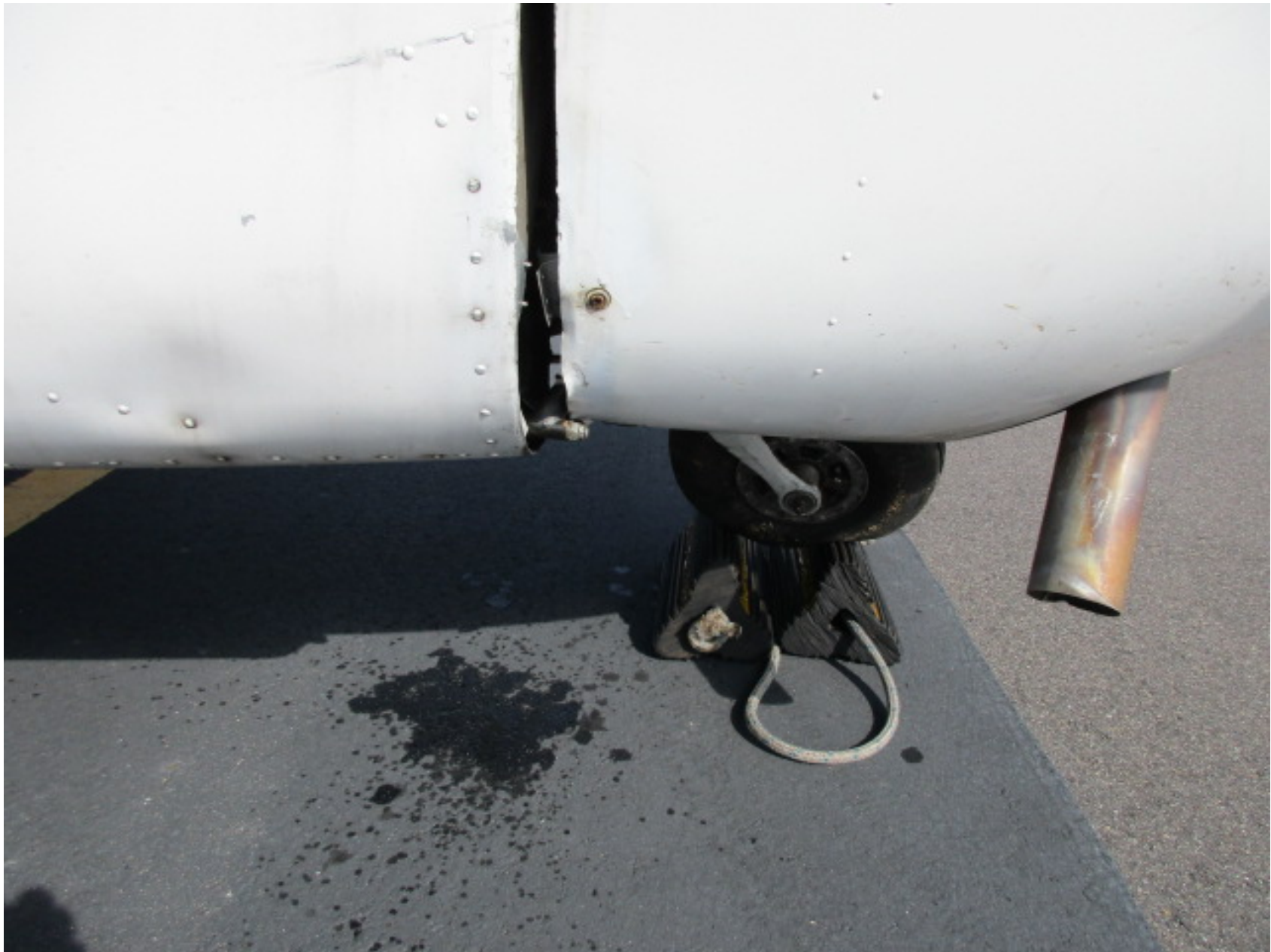
Photo 1 – FAA photo-Buckled airframe and firewall
