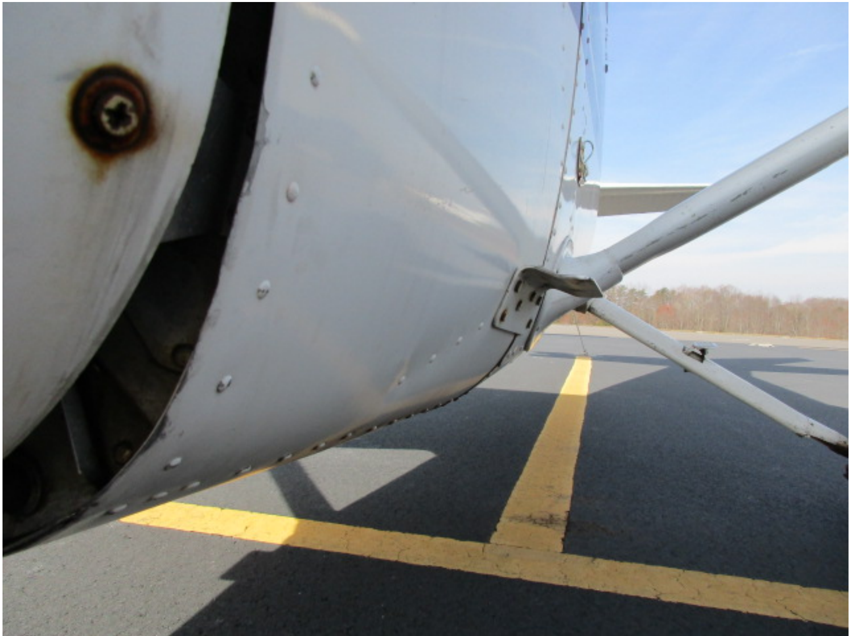
Photo 2 – FAA photo-left side buckled fuselage
