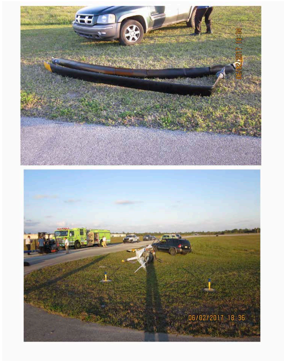
Photo 2 – FAA photo-View of bent main rotor blades and helicopter laying on its left side
