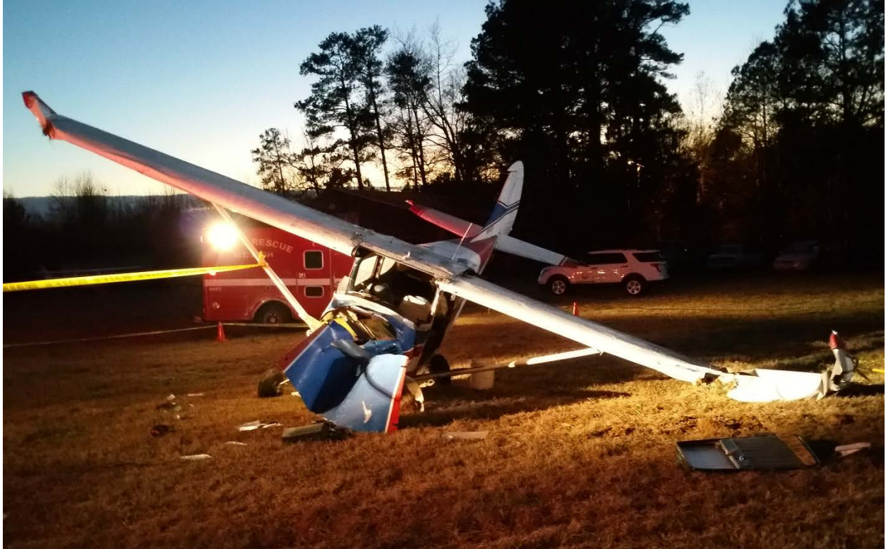
Figure 3 Front view of airplane, dent on the right wing leading edge
