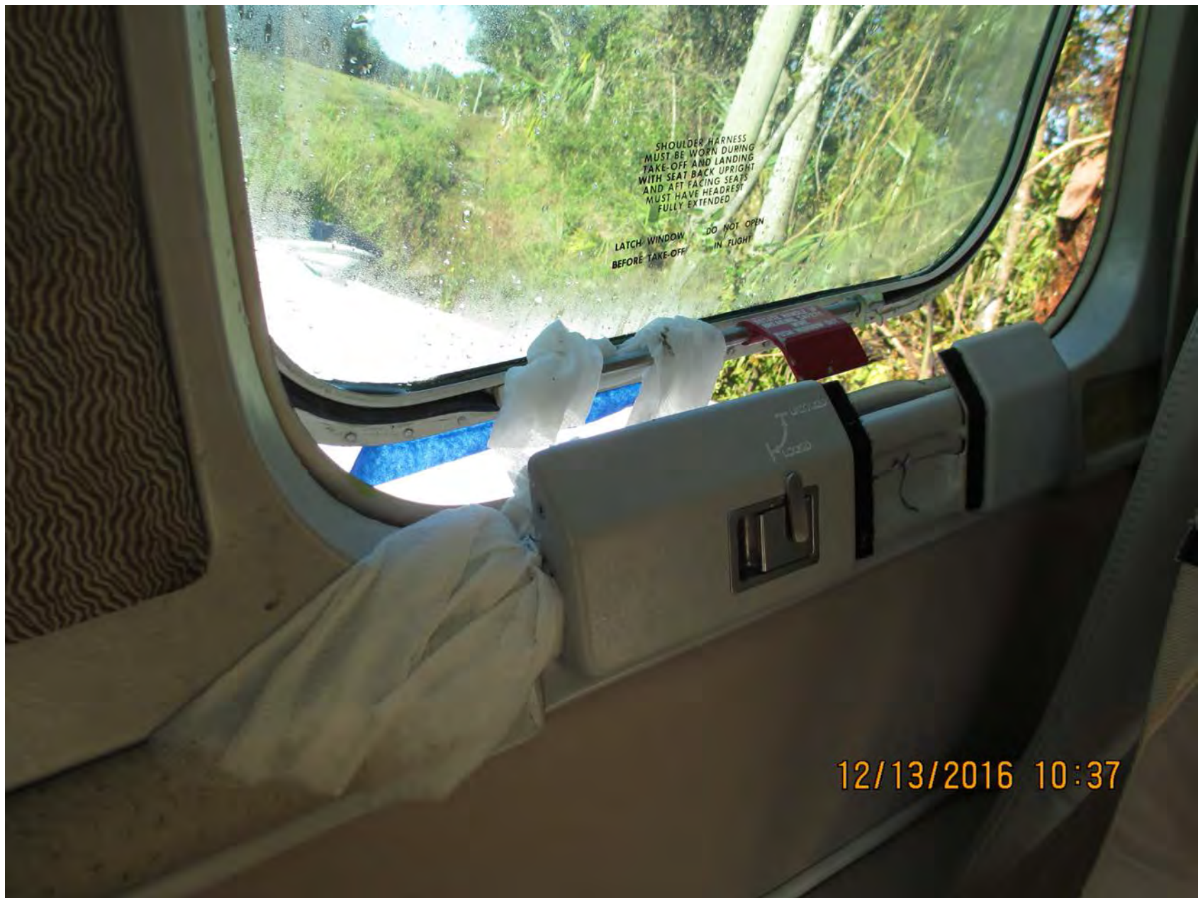
Photo 5 – Interior View of Emergency Exit Window – Courtesy of FAA
