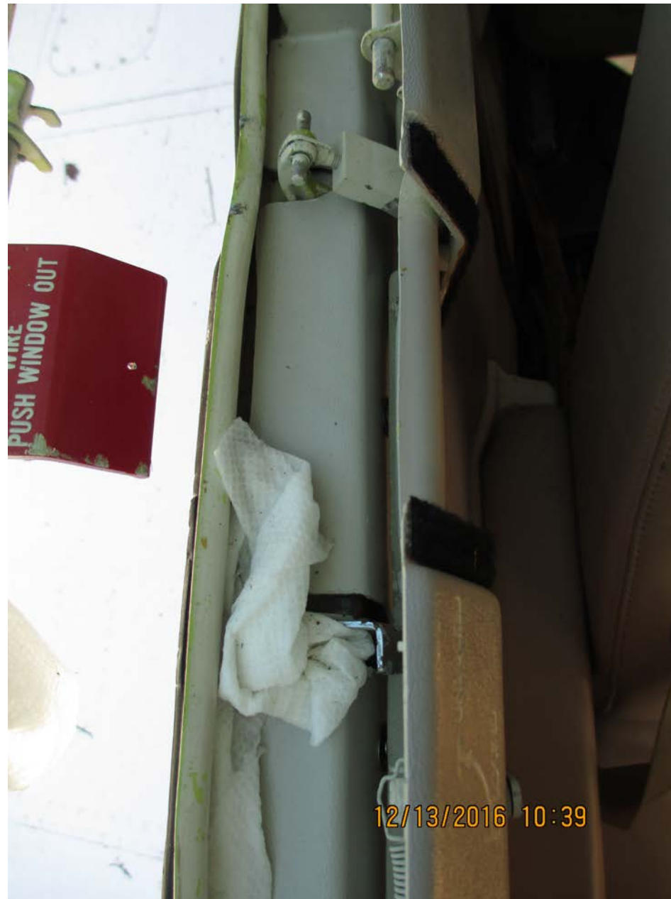
Photo 7 – Forward Portion of Emergency Exit Window Latching Mechanism – Courtesy of FAA
