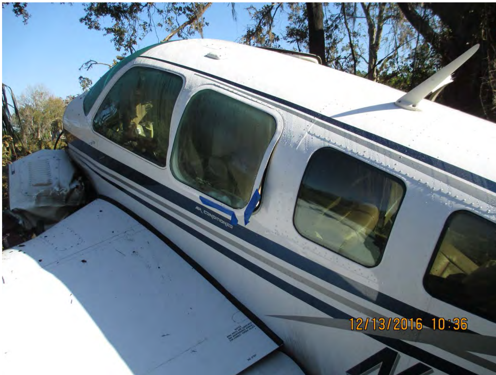
Photo 4 – Emergency Exit Window – Courtesy of FAA
