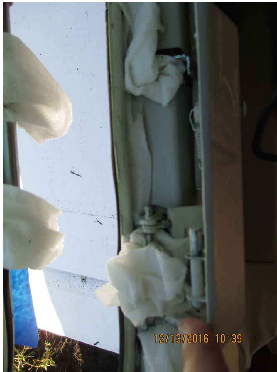
Photo 6 – Aft Portion of Emergency Exit Window Latching Mechanism – Courtesy of FAA
