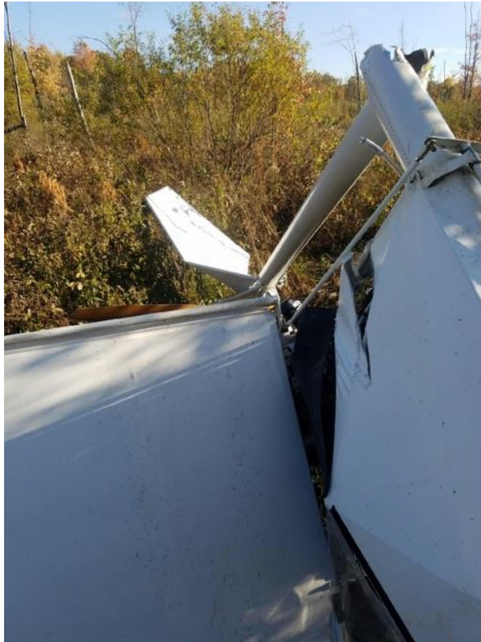
Photo 2 -View of broken emmpenage
