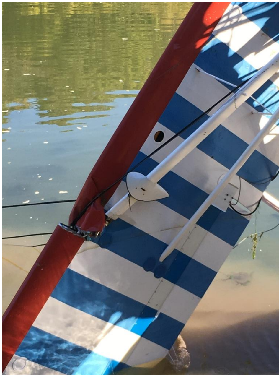
Photo 2 - Digital Photograph Provided by FAA. View of the Right Wing With Powerline Embedded in the Leading Edge
