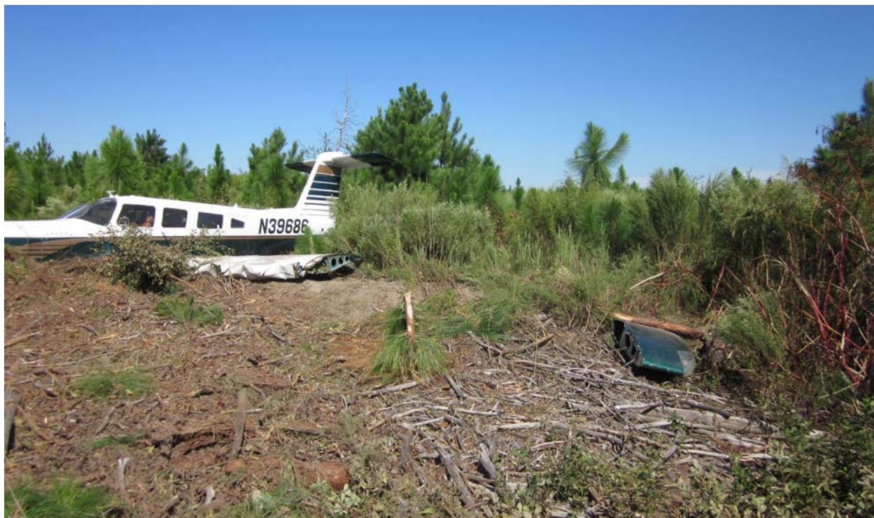
Figure 1 View of left side of airplane and separated left wingtip.
