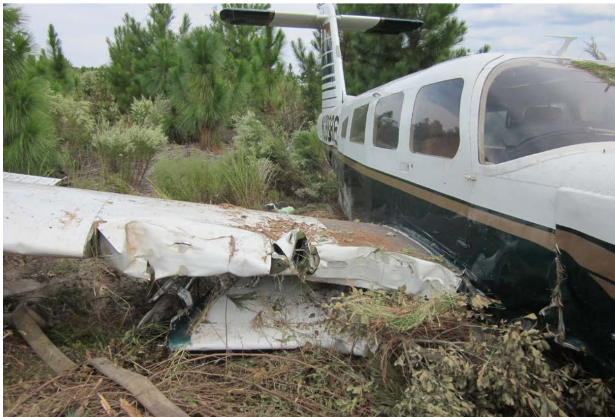
Figure 2 View of right side of airplane and crushed leading edge.
