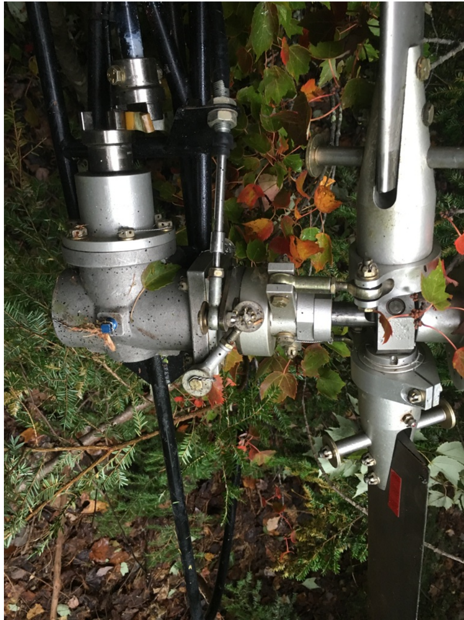
Photo 3 - FAA Digital Photograph. View of the Tailrotor Gearbox with Portions of both Tail Rotor Blades Visible.
