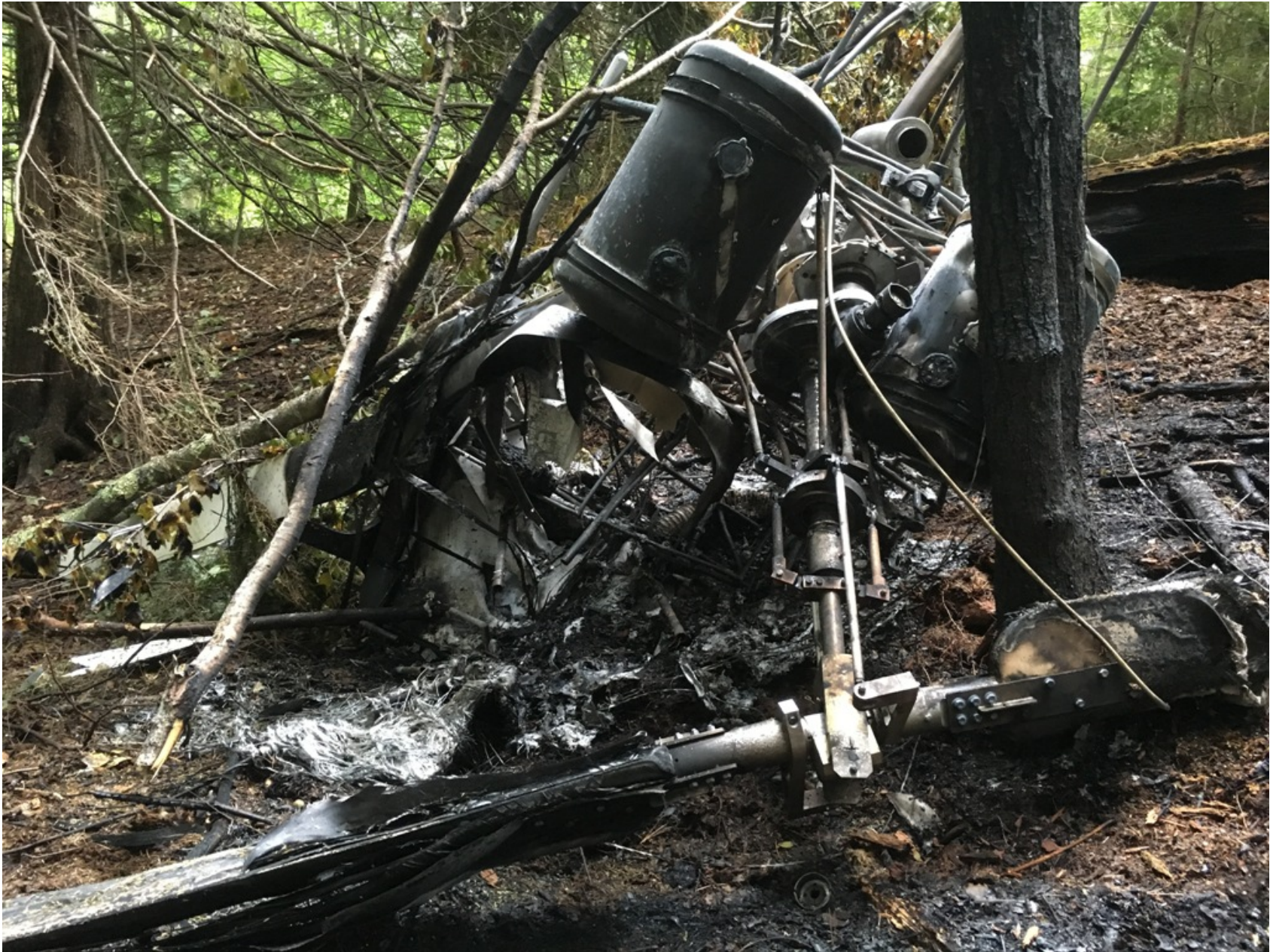
Photo 2 - FAA Digital Photograph. View of the Helicopter at the Accident Site. Note a portion of the Main Rotor Mast and Portions of Both Main Rotor Blades, with Corresponding Burn Damage.
