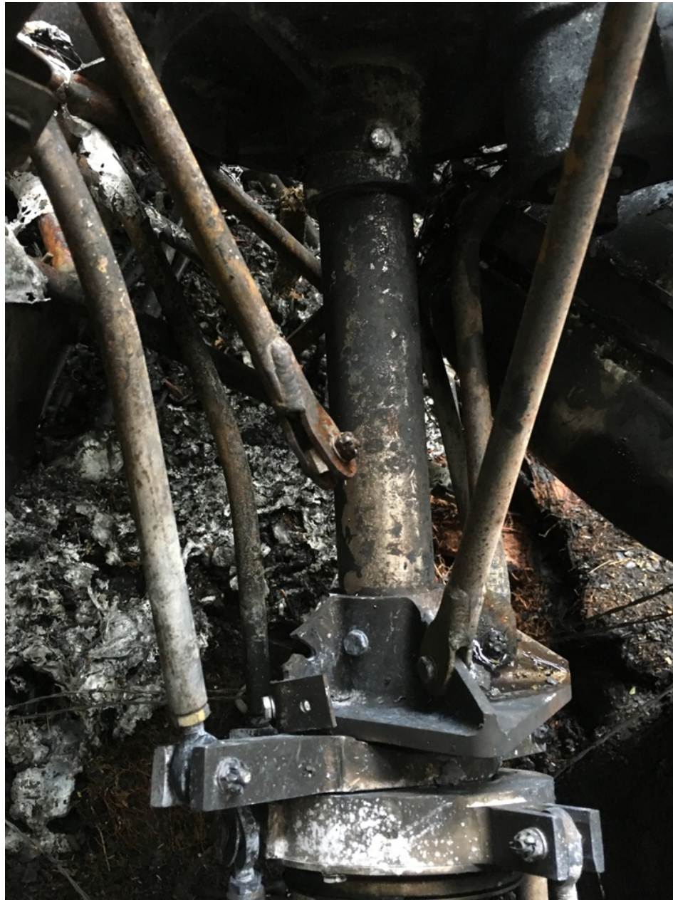
Photo 5 - FAA Digital Photograph. View Showing 3 of the 4 Transmission Struts, 2 of Which remained connected and 1 was Pulled Free From Its Attach.
