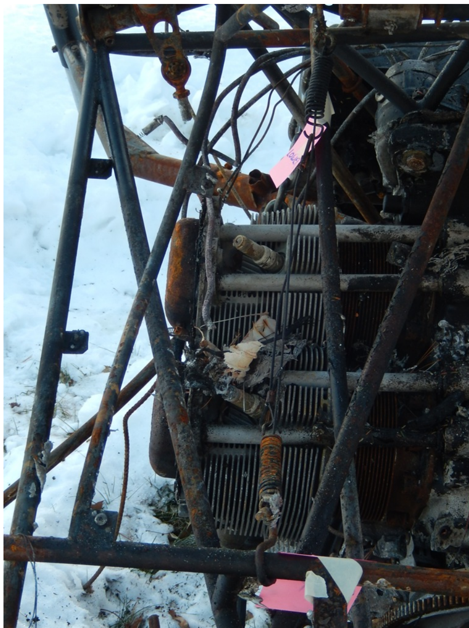
Photo 6 - Digital Photograph Provided by Pilot. View Depicting Both Collective Springs and Cables.
