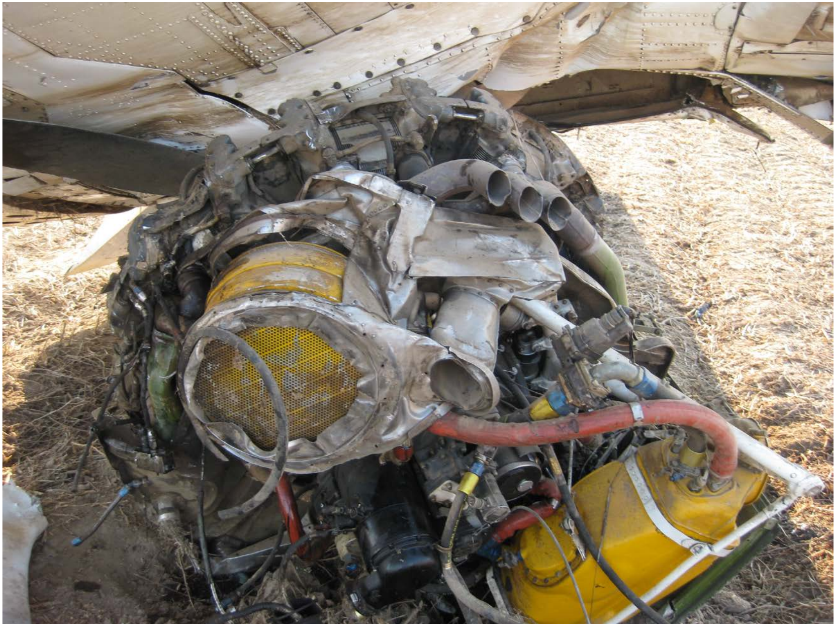
Photo 4 – View of damaged radial engine
