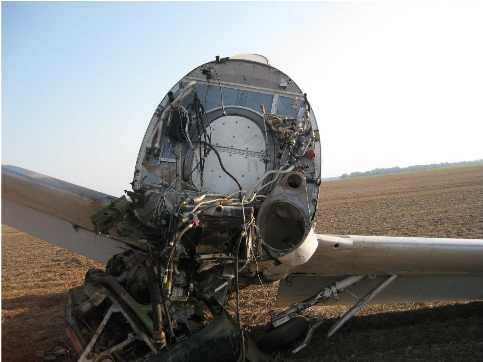
Photo 3 – Front view of engine under airplane showing firewall damage
