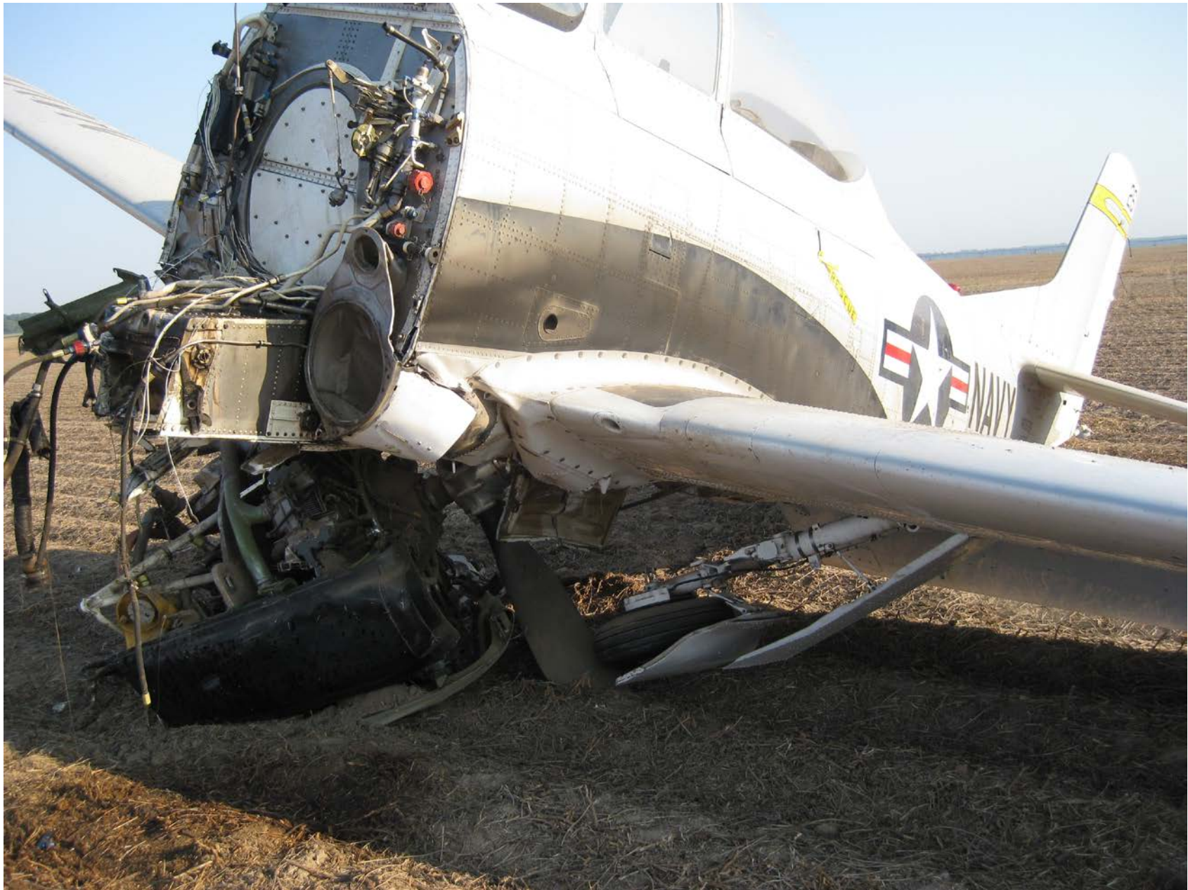
Photo 2 – View of engine separated from firewall on left side showing heavy damage
