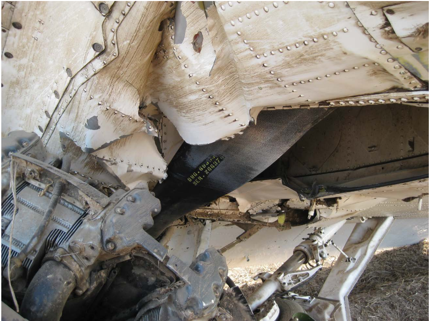
Photo 5 – View of part of the propeller and engine lodged under the damaged fuselage.
