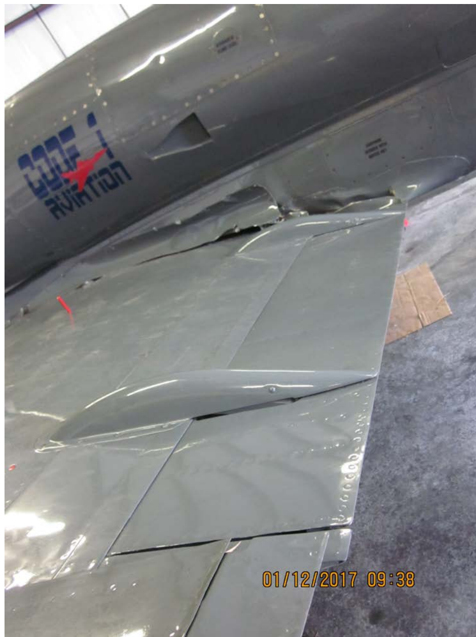
Photo 2 – Left Side Damage to Airplane (Courtesy of FAA)
