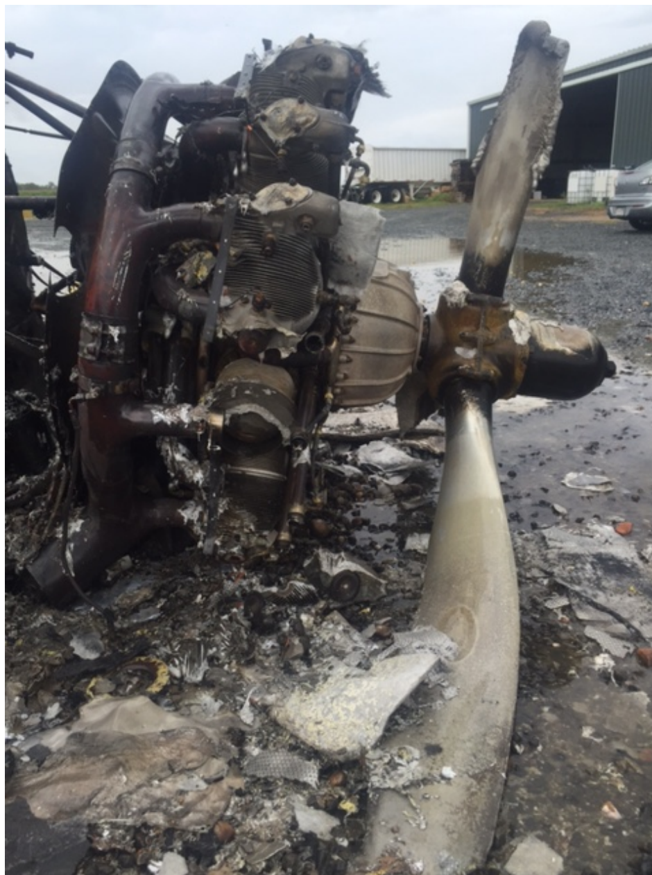
Photo 5 – Right side of radial engine damage. Note cylinders shown are number 1 on top through number 4 on bottom. (Courtesy of FAA)
