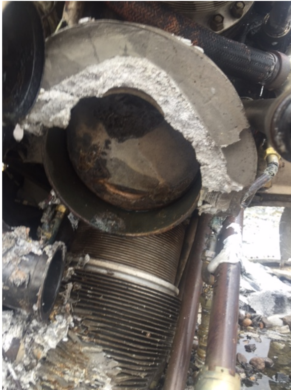
Photo 7 – Additional closeup of number 3 cylinder damage. (Courtesy of FAA)
