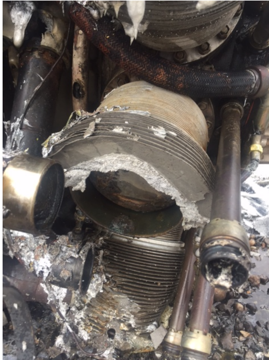
Photo 6 – Closeup of number 3 cylinder damage. (Courtesy of FAA)
