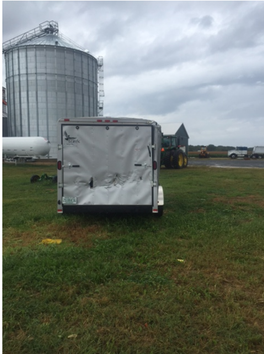
Photo 4 – View of trailer impact damage. (Courtesy of FAA)
