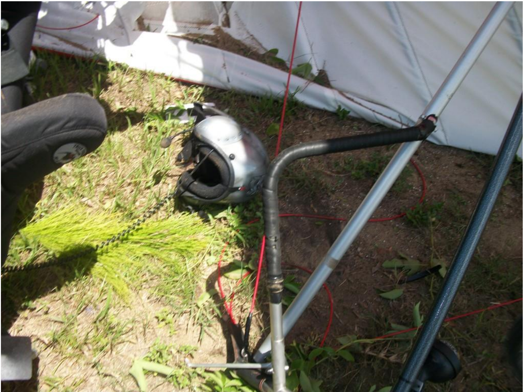
Photo 2 – Spar Damage (Eustis FL Police Photo)
