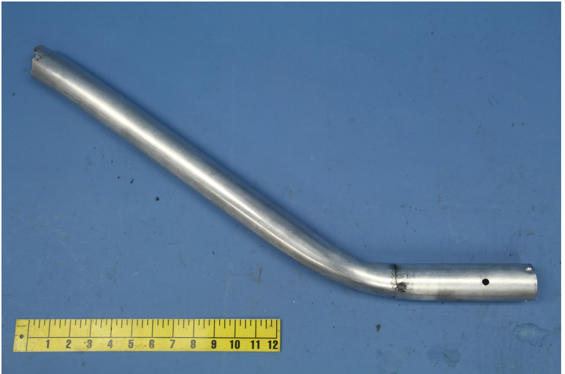
Photo 1 – Lateral View of Fractured Skid Tube
