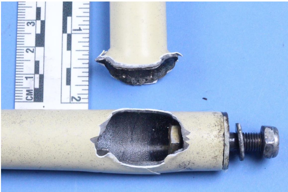
Figure 2: Fracture between the horizontal and vertical portions of the rudder pedal control tube.
