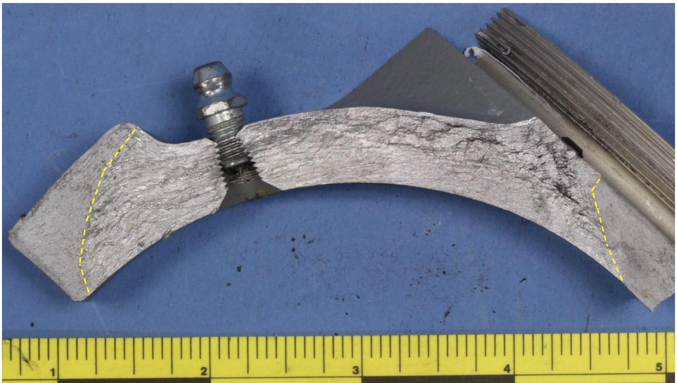
Figure 4 – The fracture surface in Figure 3, after sectioning and cleaning. The fatigue crack edges are labeled.
