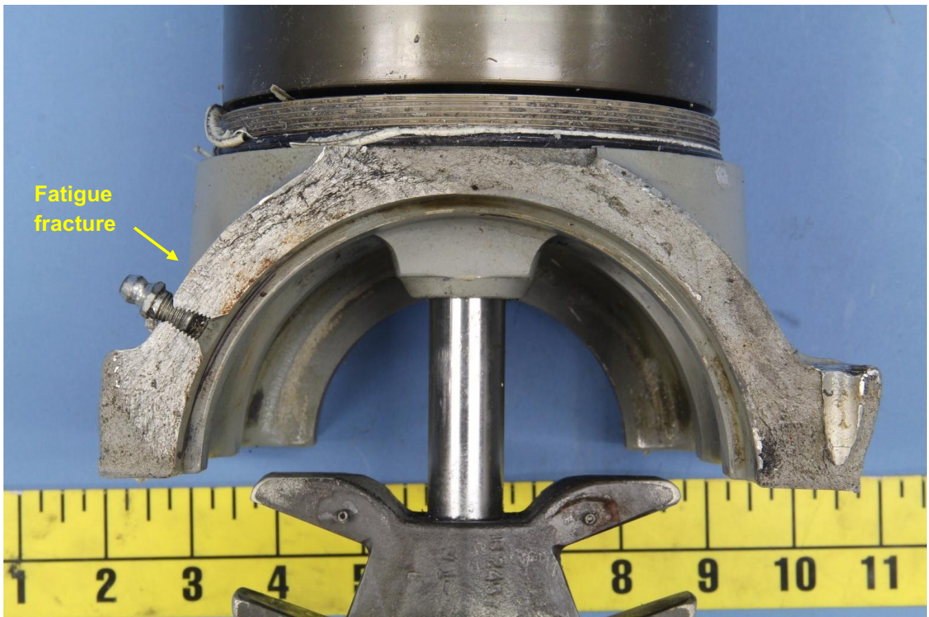
Figure 3 – The forward propeller hub half, as received, showing the fatigue cracking about a grease fitting hole.
