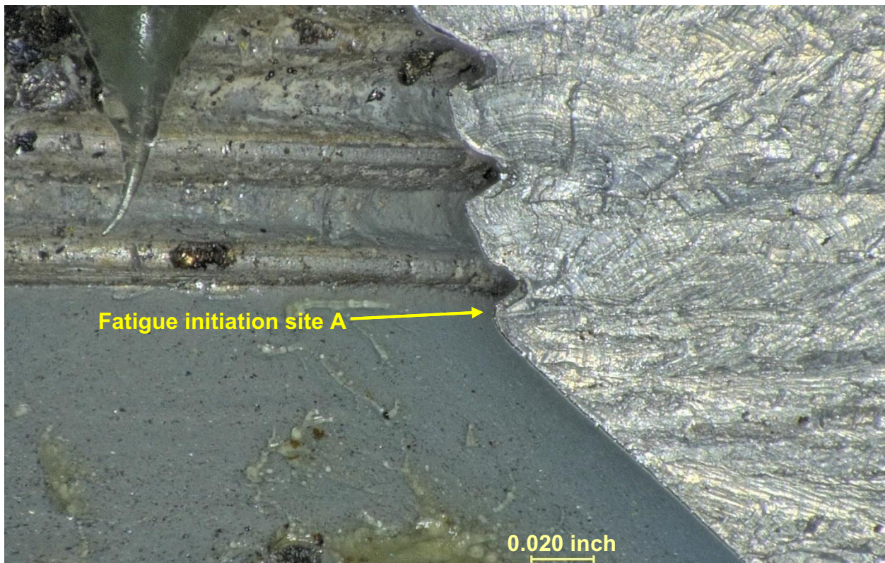
Figure 7 – Closer view of fatigue crack initiation site A (arrow), showing crack arrest marks emanating from a thread crest.
