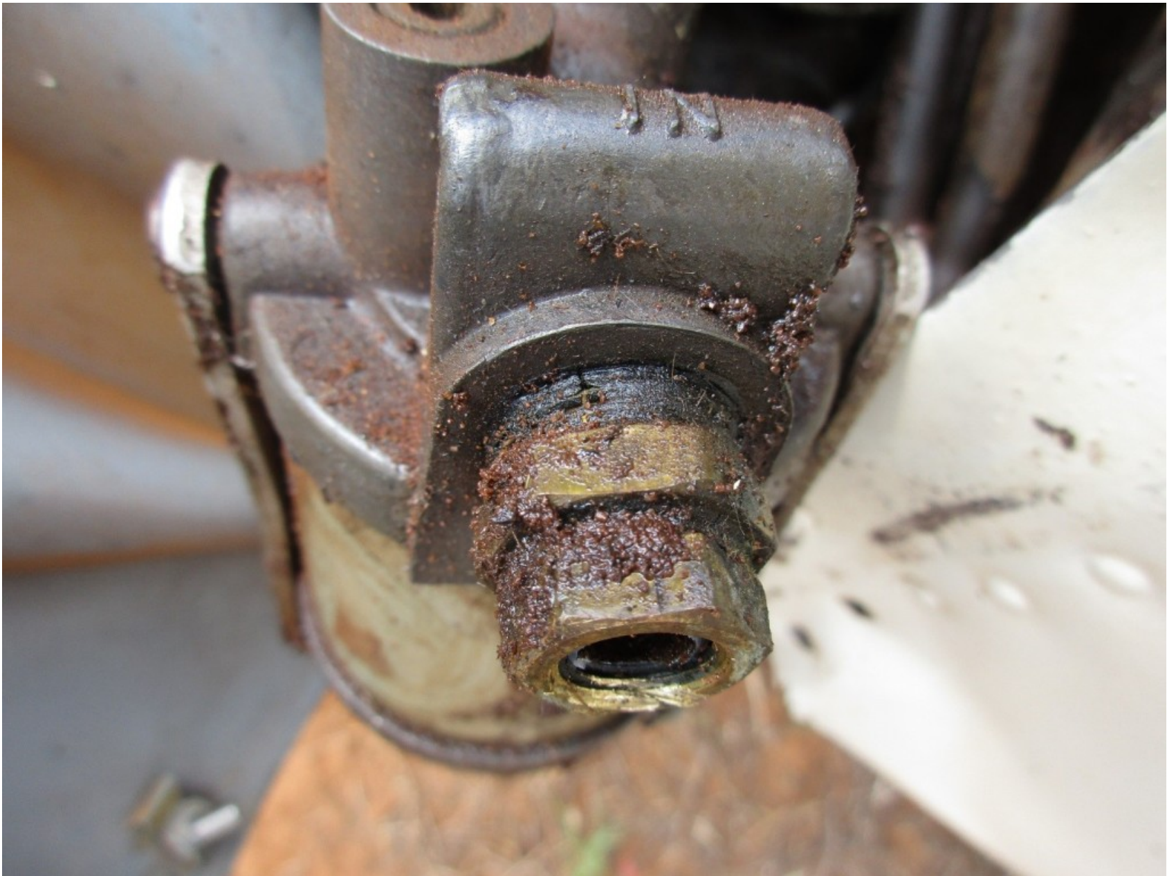
Photo 2 - FAA Digital Photograph. View of the Fractured Inlet of the Fuel Strainer.
