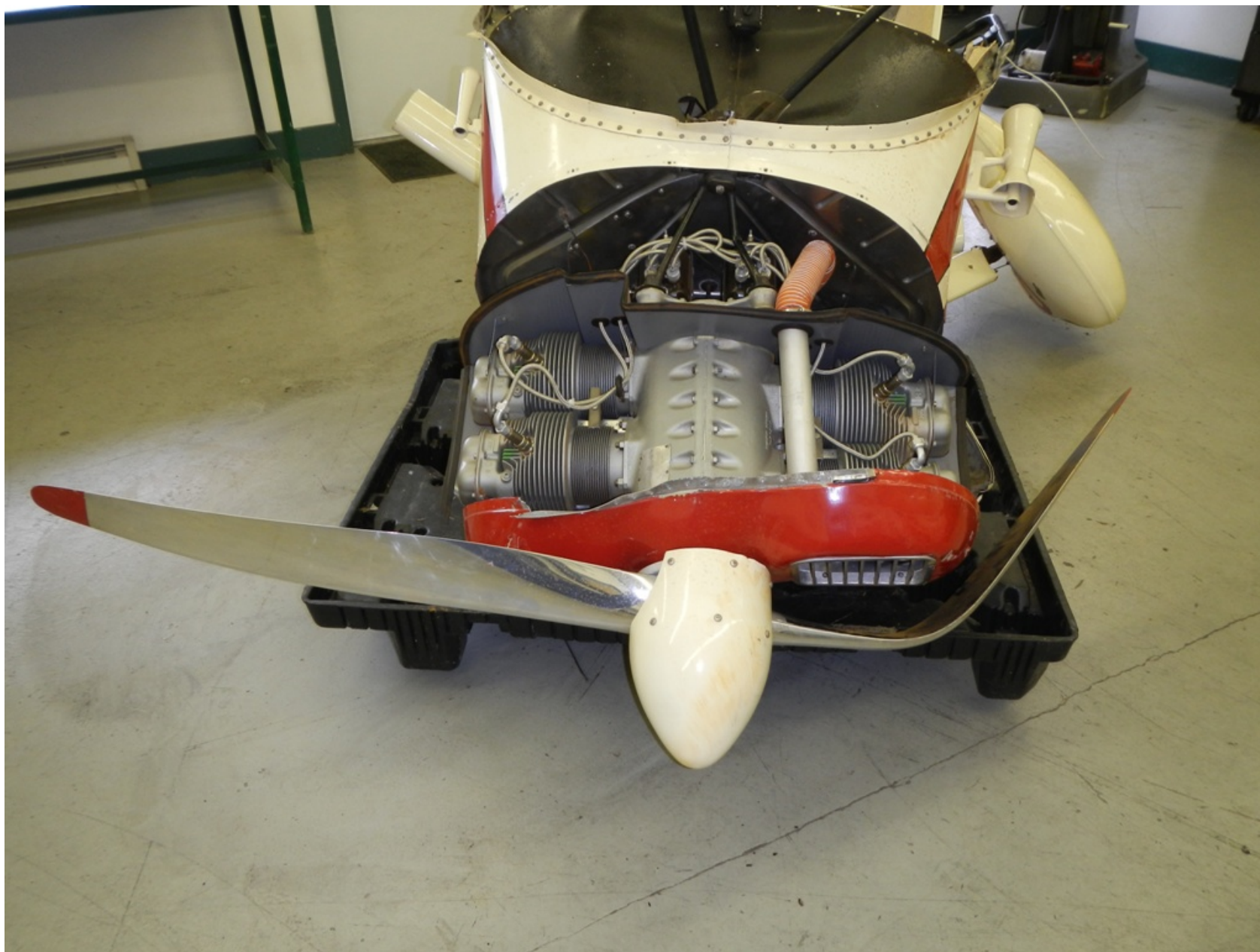
Photo 6 - CMI Digital Photograph. Forward View of the Propeller and Engine Assembly.
