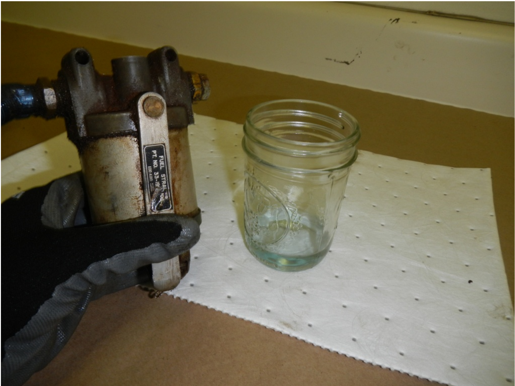
Photo 4 – CMI Digital Photograph. View of the Fuel Drained from the Fuel Strainer.
