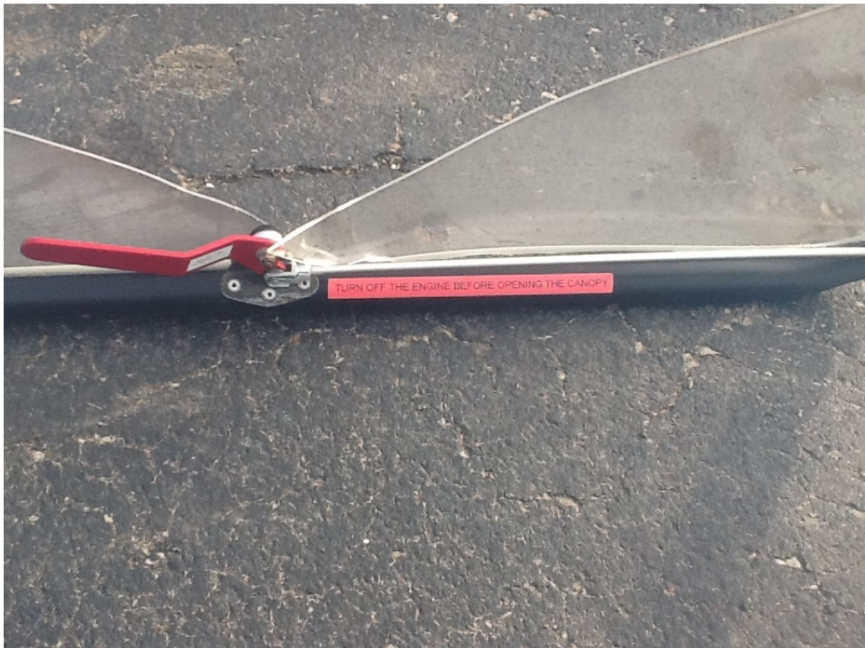
Photo 6 - Photograph Provided by Recovery Personnel. View of the Right Canopy Latch Handle
