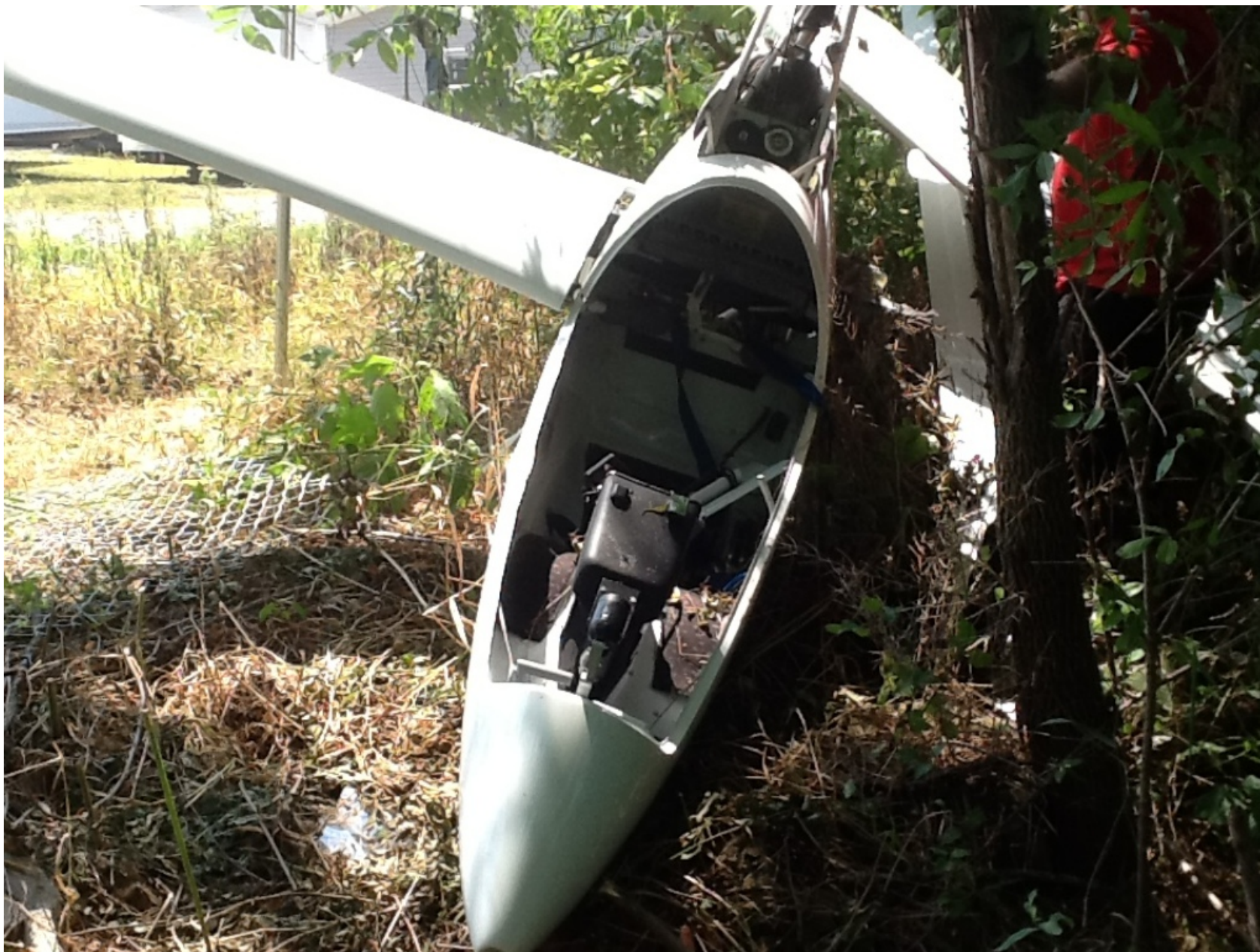
Photo 3 - Photograph Provided by Recovery Personnel. View of the Cockpit Showing the Detached Canopy
