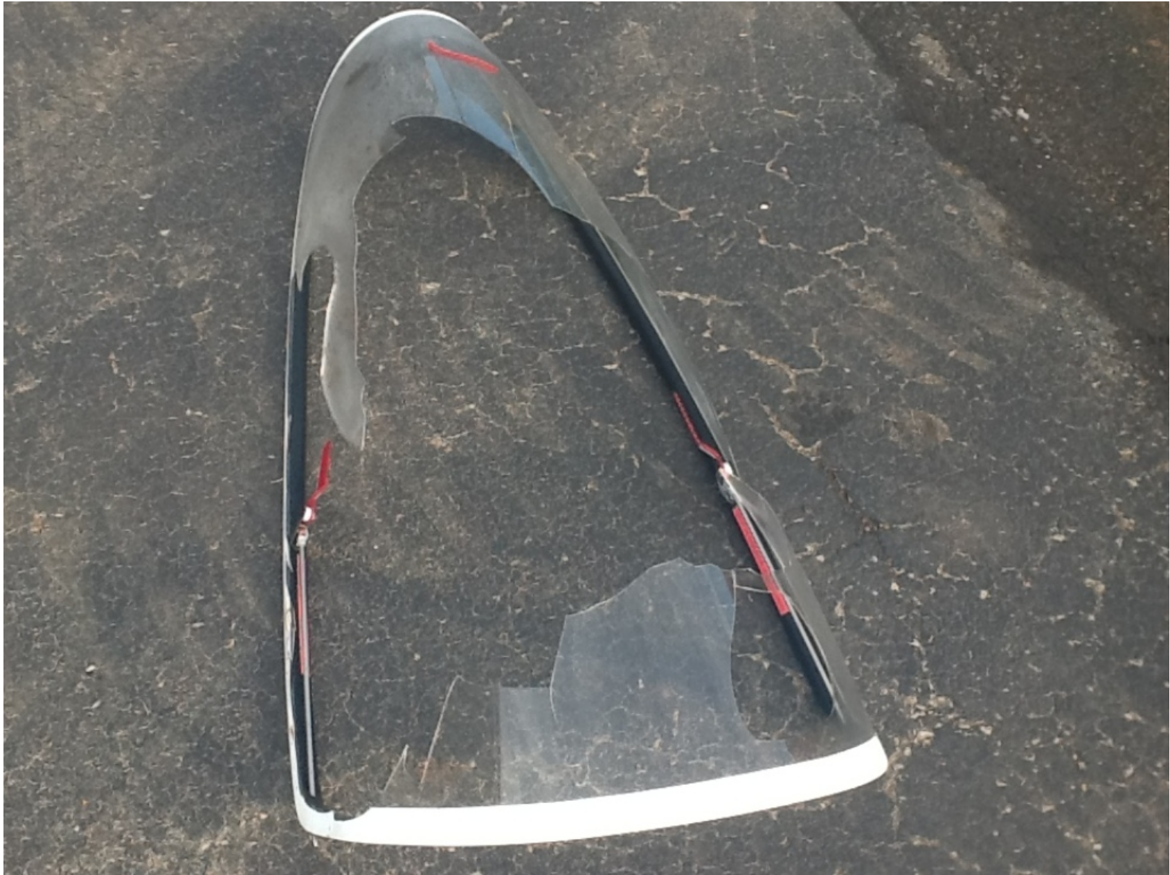
Photo 5 - Photograph Provided by Recovery Personnel. View of the Canopy. Note the Position of the Left and Right Canopy Latches
