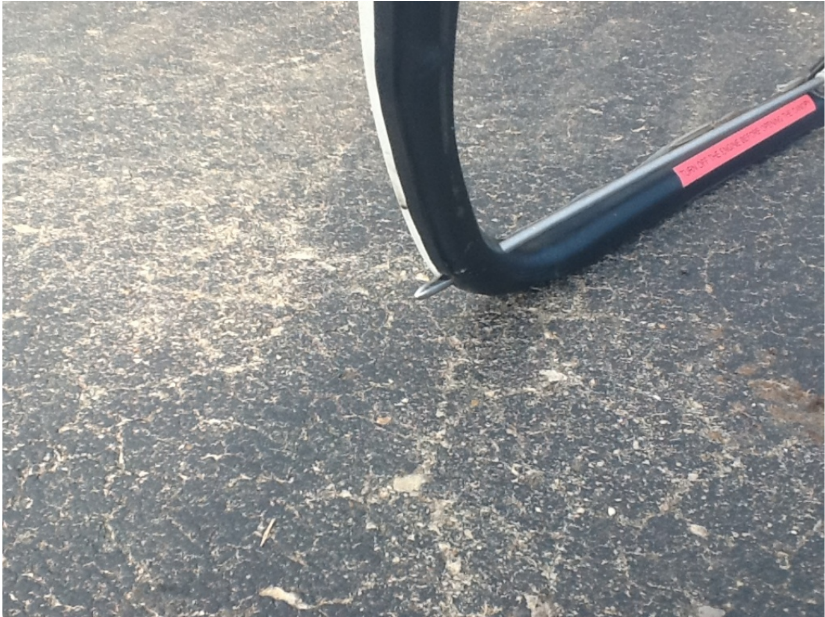
Photo 9 - Photograph Provided by Recovery Personnel. View of the Left Canopy Latch Assembly Depicting the Pin Extending Beyond the Canopy Frame
