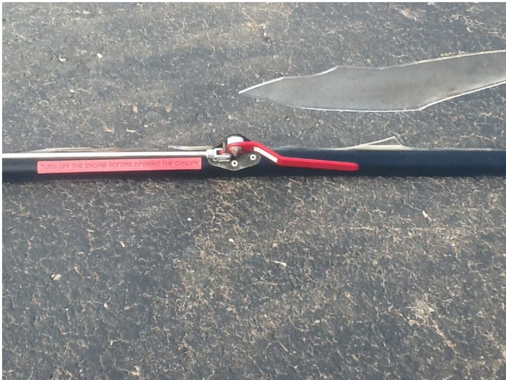
Photo 7 - Photograph Provided by Recovery Personnel. View of the Left Canopy Latch Handle
