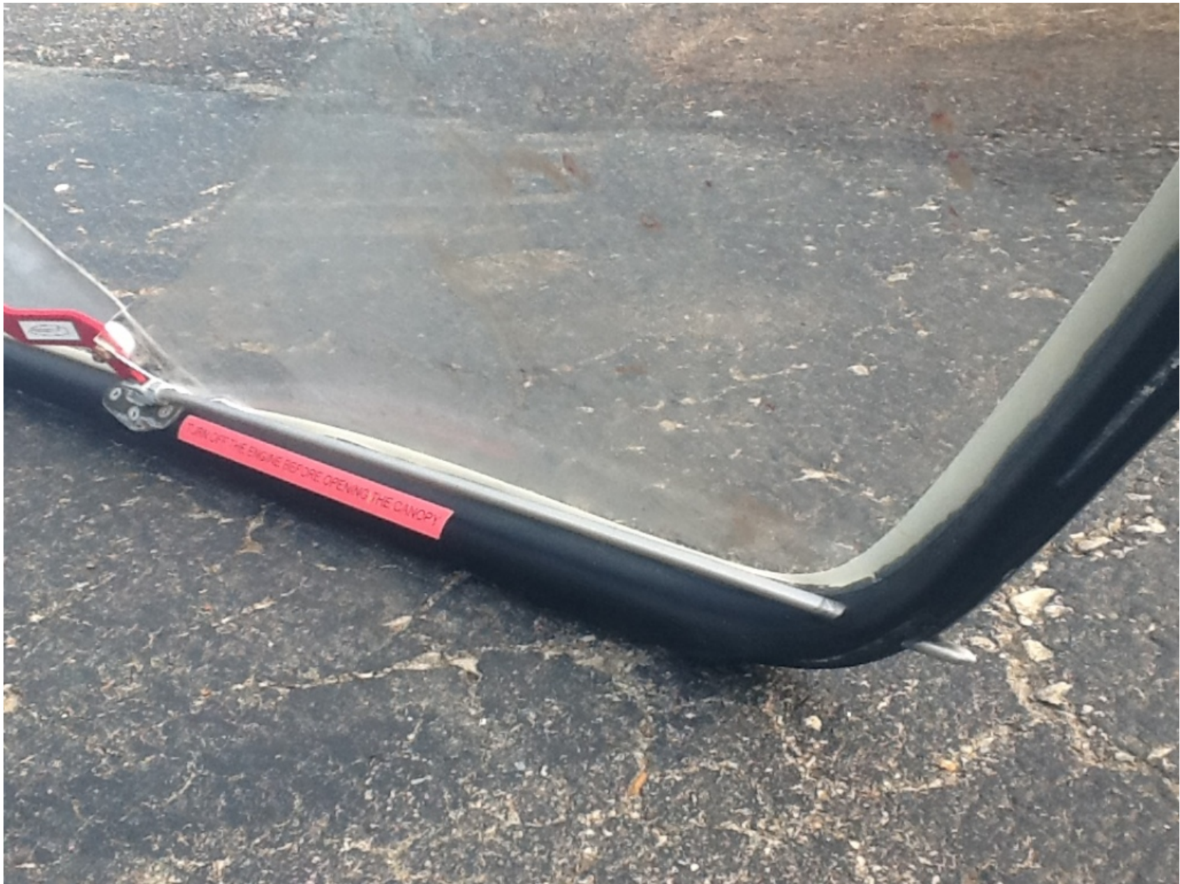
Photo 8 - Photograph Provided by Recovery Personnel. View of the Right Canopy Latch Assembly Depicting the Pin Extending Beyond the Canopy Frame
