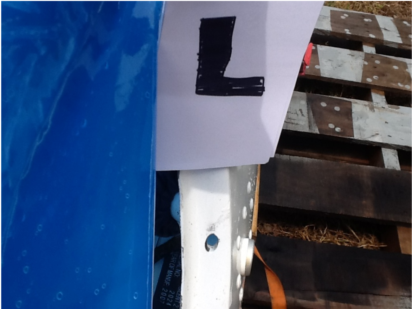
Photo 10 - Photograph Provided by Recovery Personnel. View of the Left Canopy Latch Pin Receiver
