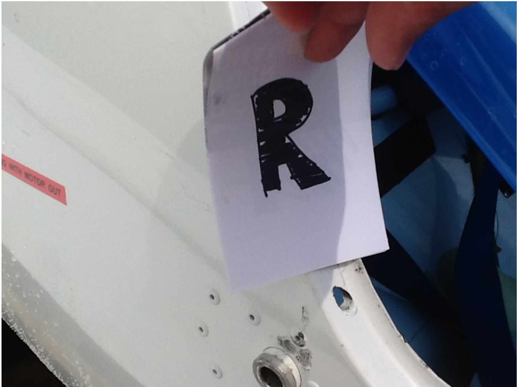
Photo 11 - Photograph Provided by Recovery Personnel. View of the Right Canopy Latch Pin Receiver
