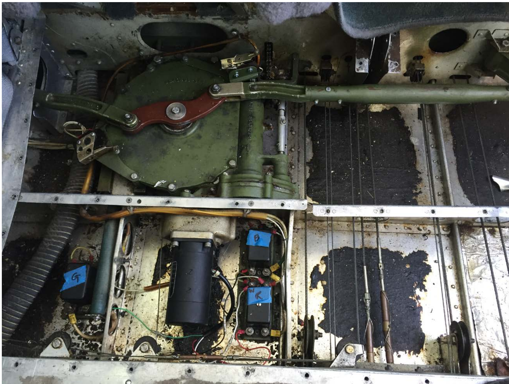
Photo 5 - View of Accident Landing Gear Actuator as Found (FAA)
