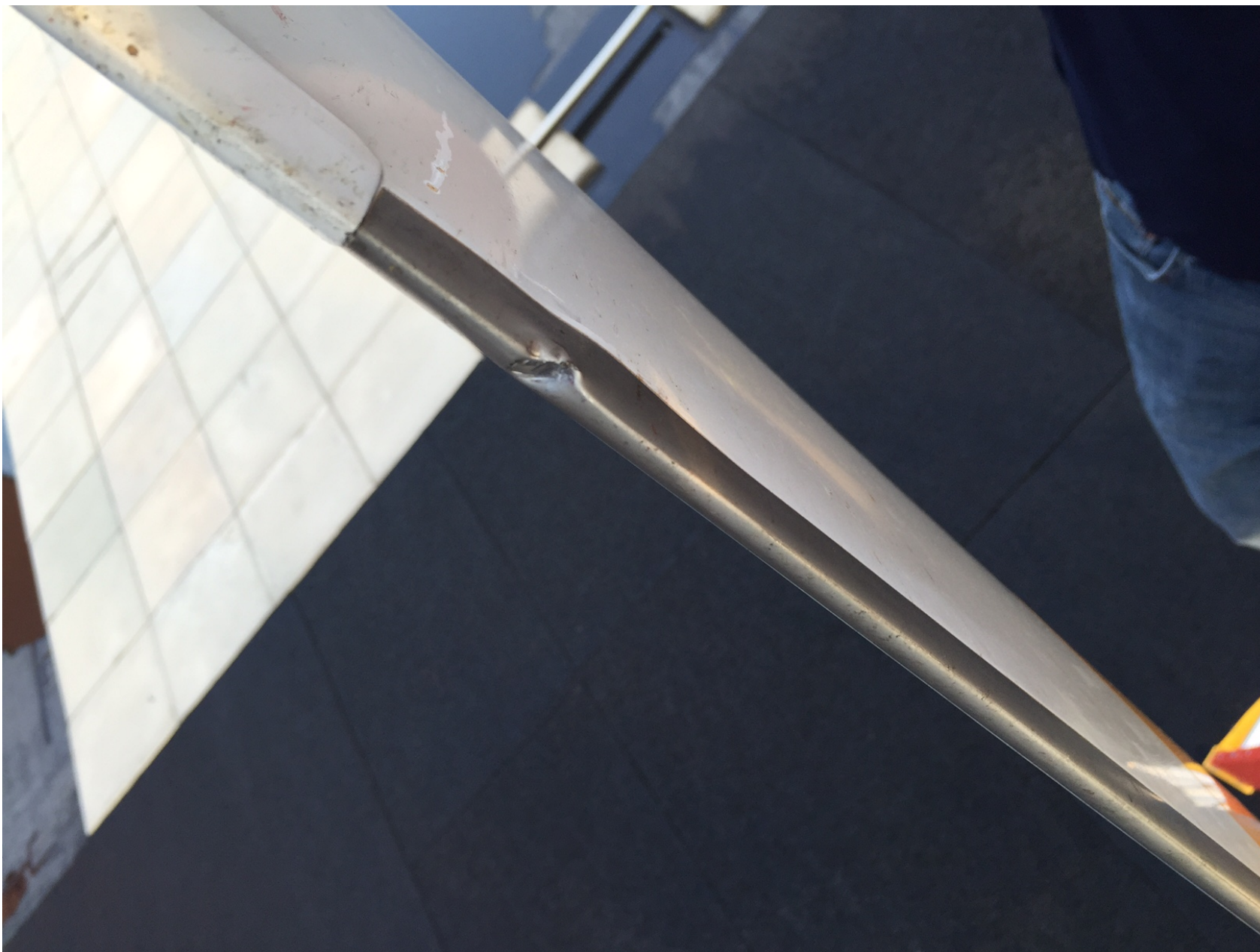
Photo 1 – Tailrotor Blade Damage (Photo Courtesy of FAA)
