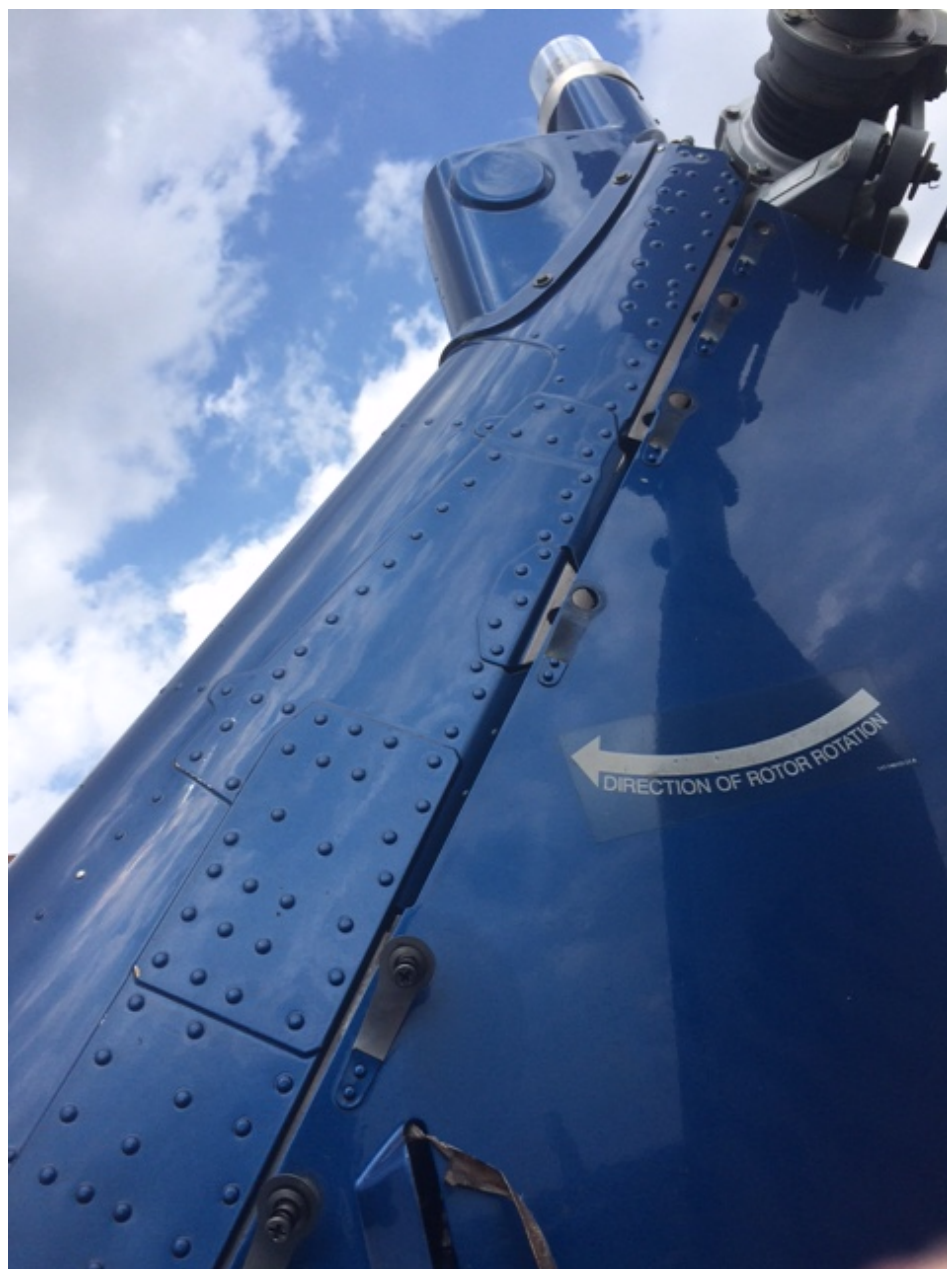
Photo 2 – Aft Vertical Cowling (Photo Courtesy of FAA)
