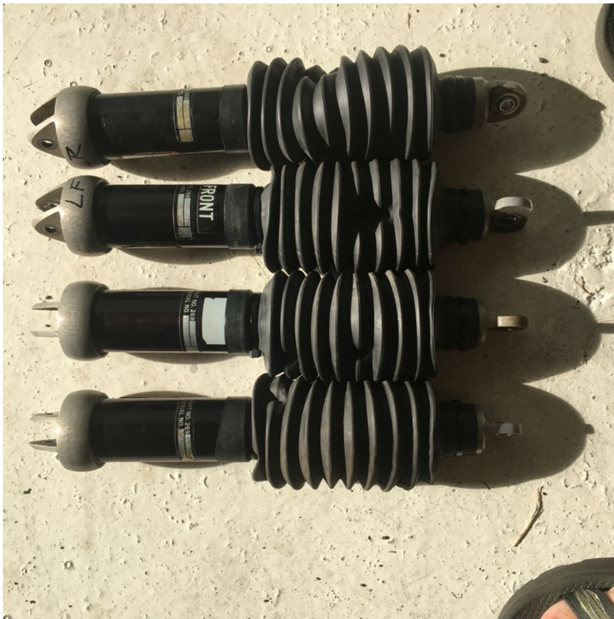
Photo 4 - FAA Digital Photograph. View of the Landing Gear Dampers Following Removal
