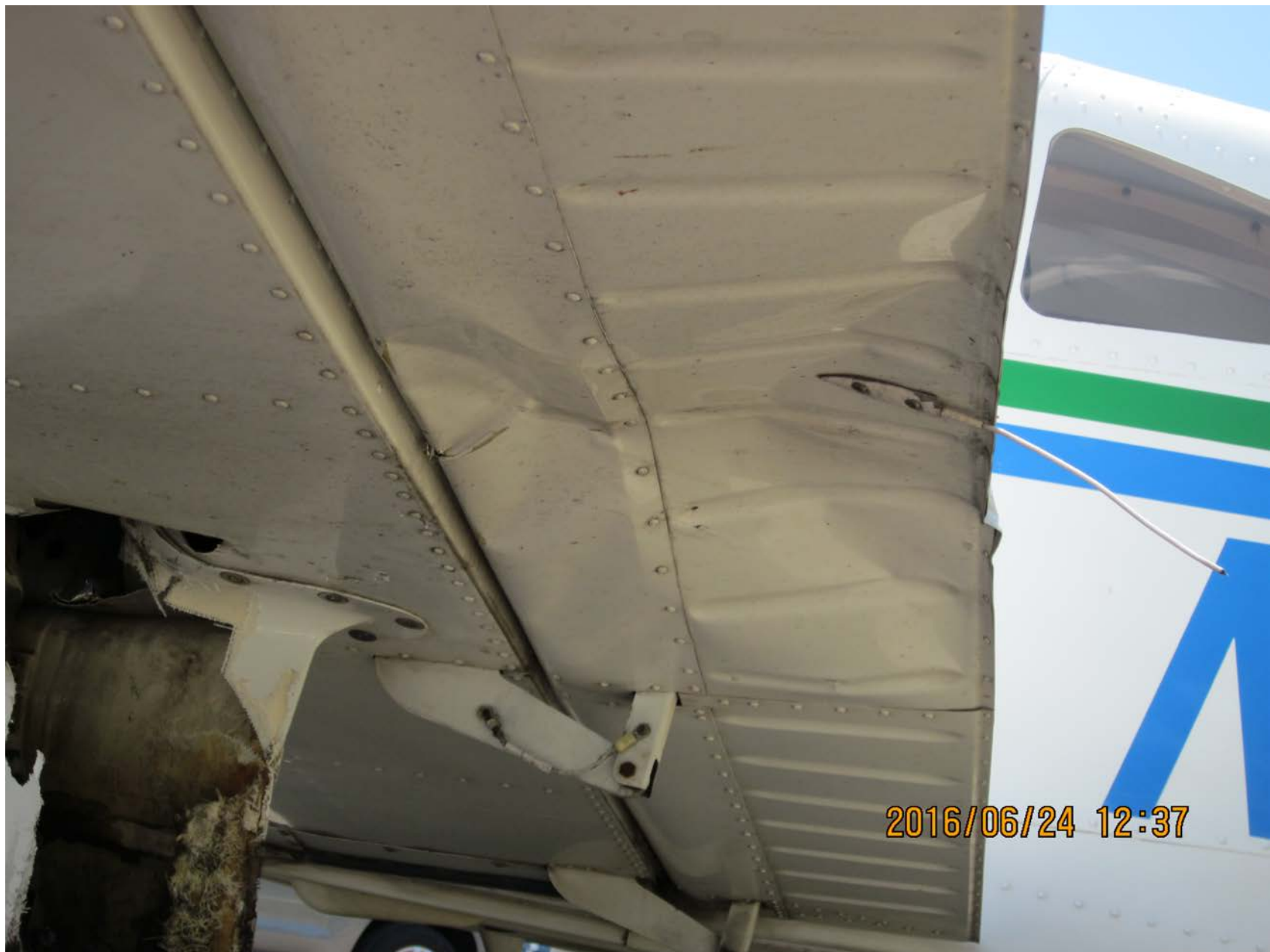
Photo 2 – FAA photo- View of under wing showing left flap damage
