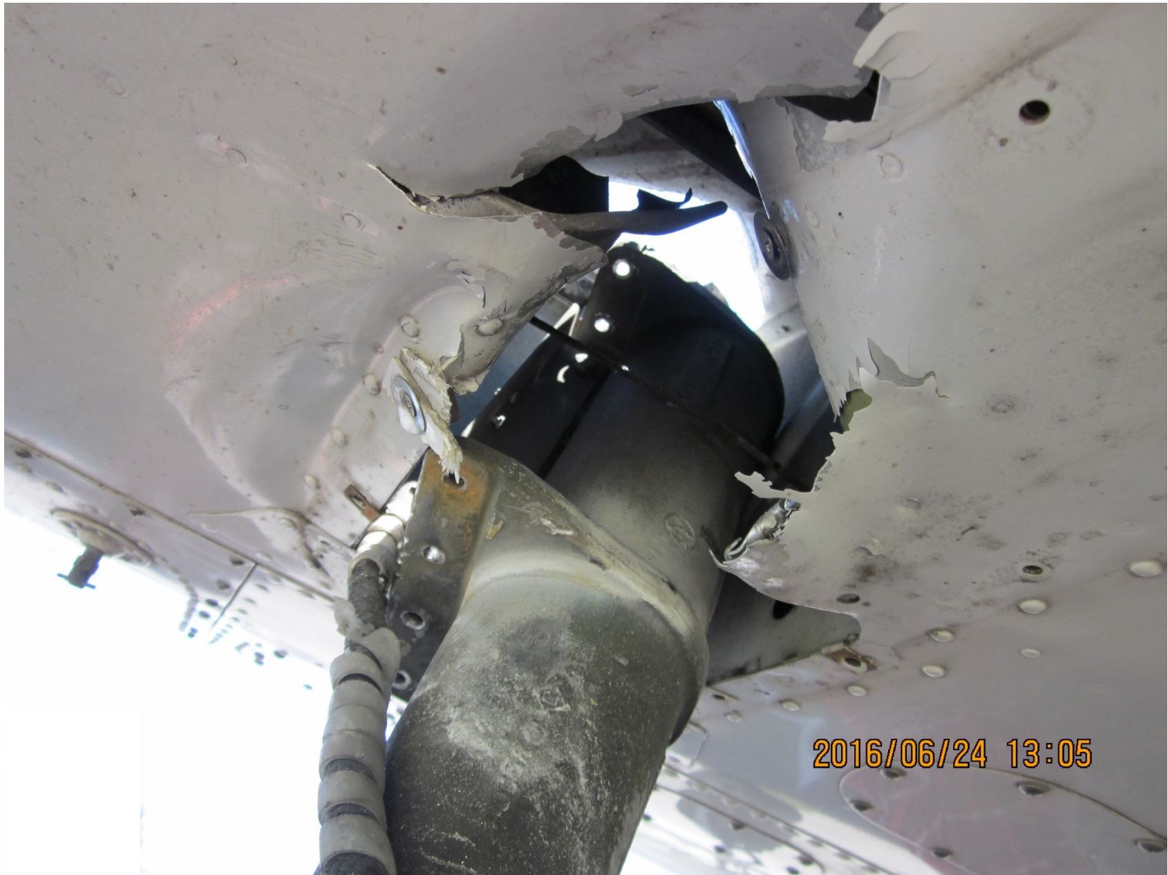
Photo 4 – FAA photo-view of strut separated in wing
