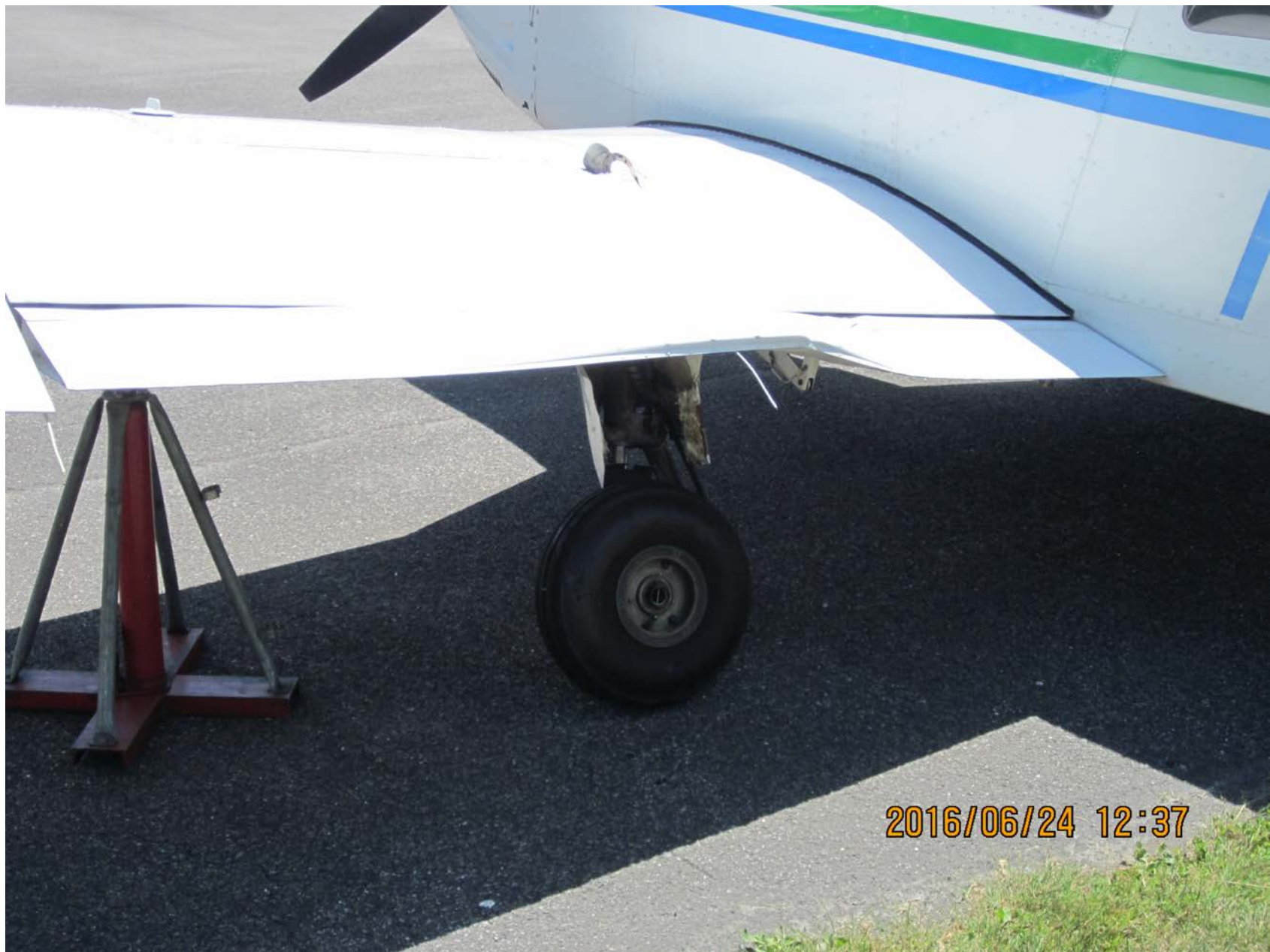
Photo 1 – FAA photo- Left landing gear strut protruding from top of left wing
