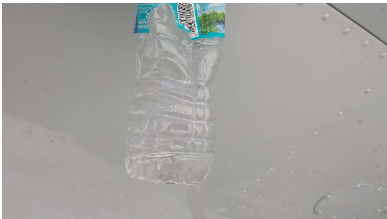
Figure 2. Sample of the water sumped from the engine.
