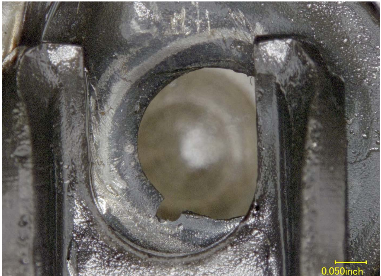
Figure 5 – Closer view of the diaphragm retainer from Figure 4, showing a slanted circular fracture.
